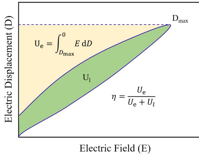
**Fig. S5.** Schematic diagram of D-E hysteresis loop. Where  $D_{\max}$  represents maximal electric displacement, the discharged energy density is determined from the area in yellow, the green area reveals the loss of energy density, and the discharged energy efficiency is determined from the ratio between the yellow area and the total area of yellow and green.
