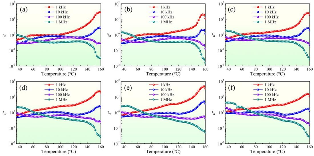
**Fig. S2.** Temperature-dependence of dielectric loss ( $\epsilon''$ ) at 1 kHz, 10 kHz, 100 kHz and 1 MHz for the pure PVDF films (a) and its polymer composite films with different PTC terpolymer contents of 10 wt% (b), 20 wt% (c), 30 wt% (d), 40 wt% (e) and 50 wt% (f).
