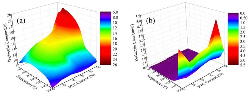
**Fig. S3.** Temperature-dependence of dielectric constant ( $\epsilon'$ ) (a) and loss tangent ( $\tan\delta$ ) (b) at 1 kHz for the pure PVDF films and its polymer composite films with different PTC terpolymer contents of 10 wt%, 20 wt%, 30 wt%, 40 wt% and 50 wt%.
