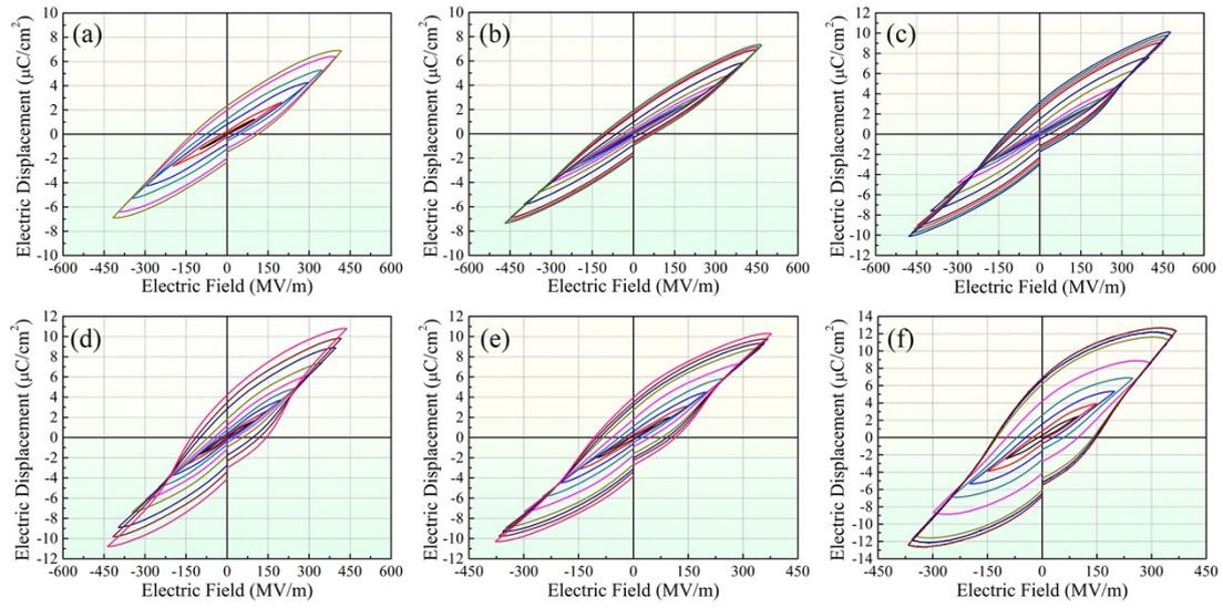
**Fig. S4.** D-E loops of the pure PVDF films (a) and its polymer composite films with different PTC terpolymer contents of 10 wt% (b), 20 wt% (c), 30 wt% (d), 40 wt% (e) and 50 wt% (f).
