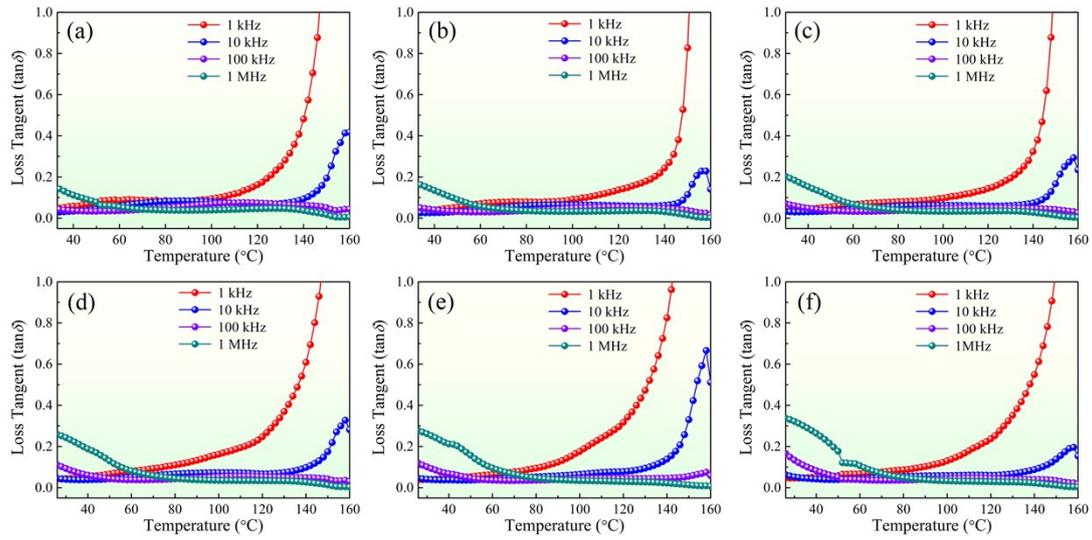
**Fig. S1.** Temperature-dependence of loss tangent ( $\tan\delta$ ) at 1 kHz, 10 kHz, 100 kHz and 1 MHz for the pure PVDF films (a) and its polymer composite films with different PTC terpolymer contents of 10 wt% (b), 20 wt% (c), 30 wt% (d), 40 wt% (e) and 50 wt% (f).
