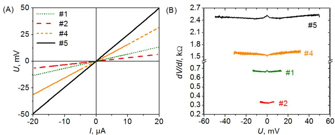
**Fig. S6.**  $V(I)$  (A) and  $dV/dI(V)$  (B) curves for single Bi nanowires measured at 1.2 K. Data for the samples #1, #2, #4, and #5 are presented by green, red, orange, and black lines, respectively.
