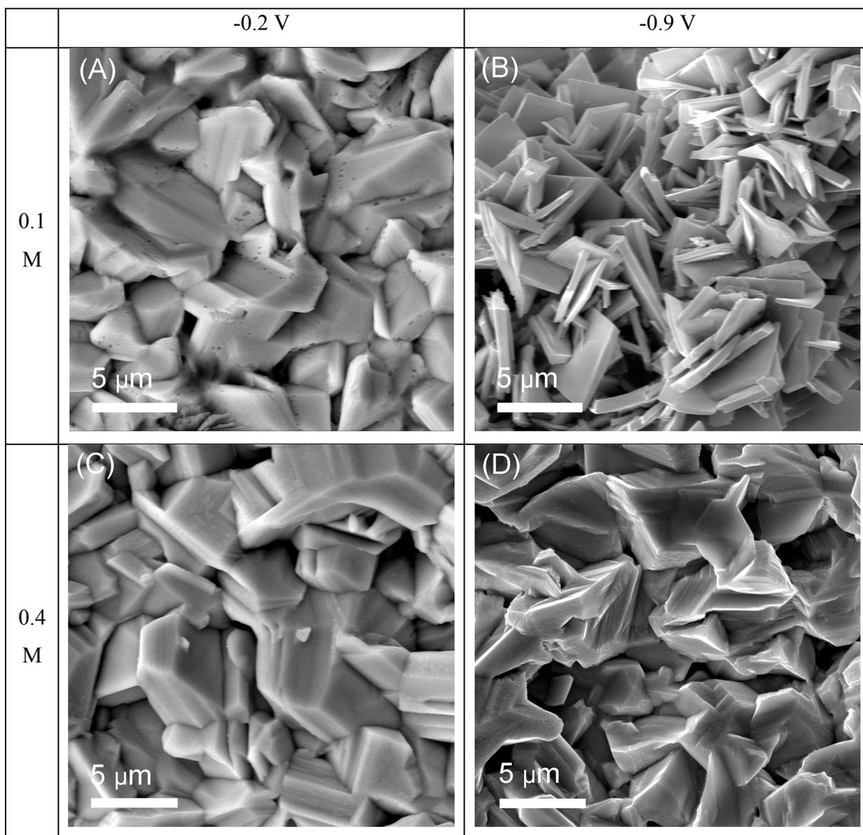
**Fig. S3.** SEM images of Bi deposits obtained in kinetic (left column) and diffusion (right column) regimes on bare Au/Bi substrates. Electrolytes containing 0.1 M and 0.4 M  $\text{Bi}(\text{NO}_3)_3$  were used.
