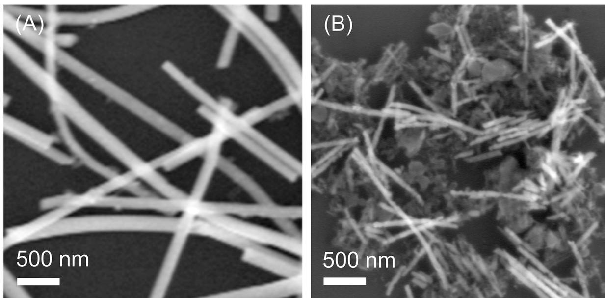
**Fig S5.** SEM images of Bi nanowires seeded onto Si/SiO<sub>2</sub> substrates from (A) as-prepared and (B) four month aged isopropanol-based suspensions. Nanowires are obtained from the nanocomposites based on AAO\_120V (A) and AAO\_40V (B).
