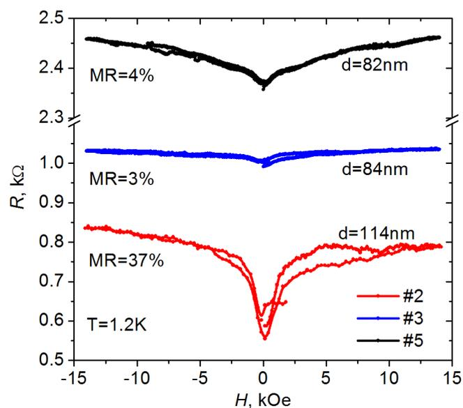
**Fig. S7.** Typical dependence of the resistance on the perpendicular magnetic field at 1.2 K for individual Bi nanowires. Data for the samples #2, #3, and #5 are presented by red, blue, and black lines, respectively. The current of 50 nA has been passed through the samples during measurements.
