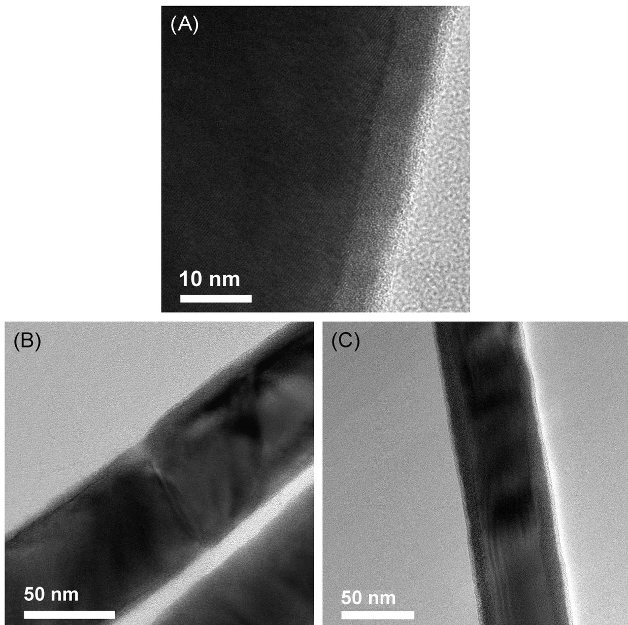
**Fig. S4.** (A) HRTEM data for as-prepared Bi nanowire obtained from the electrolyte containing 0.4 M  $\text{Bi}(\text{NO}_3)_3$  at  $E_d = -0.2$  V. TEM images of bismuth nanowires suspended in hexane (an aprotic solvent): (B) as-prepared, (C) after one month storage.
