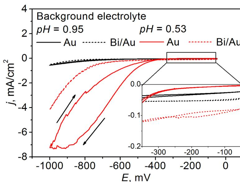
**Fig. S2.** Cyclic voltammograms recorded for Bi-free baths at potential scan rate of  $5 \text{ mV s}^{-1}$ . A bare polycrystalline Au plates with (marked as Bi/Au) and without predeposited Bi (marked as Au) served as working electrodes. Potentials are given versus saturated (KCl) Ag/AgCl reference electrode.
