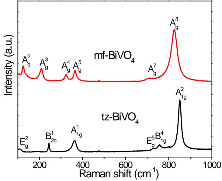
**Figure S2.** Raman patterns of fergusonite- and zircon-type  $\text{BiVO}_4$  obtained at ambient conditions.
