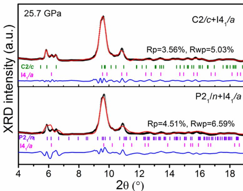
**Figure. S3.** Comparison of the Rietveld refinement of XRD pattern at 25.7 GPa using  $P2_1/n$  and  $C2/c$  structure models respectively. The experimental data are shown as black crosses with refinements shown as red solid lines and the difference between calculated and observed intensities is shown as blue lines. Ticks indicate the positions of Bragg peaks.
