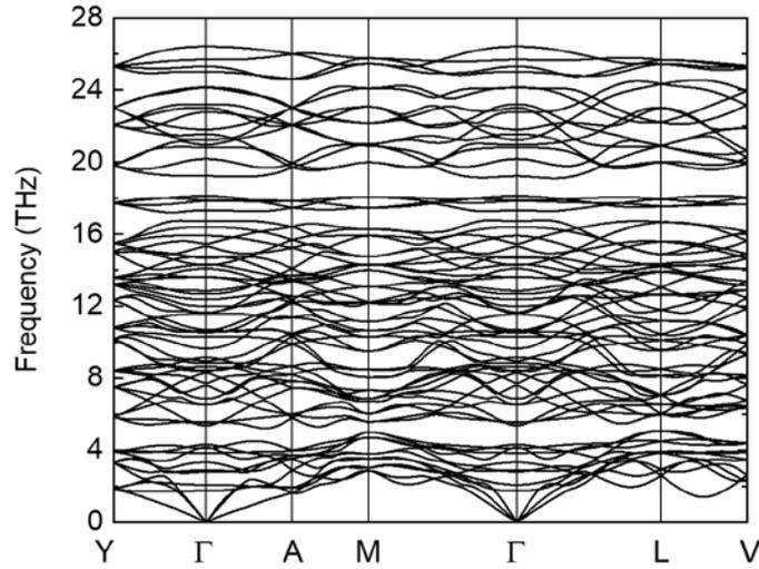
**Figure S4.** Calculated phonon dispersion relations for  $\beta$ -fergusonite structure at 30 GPa.
