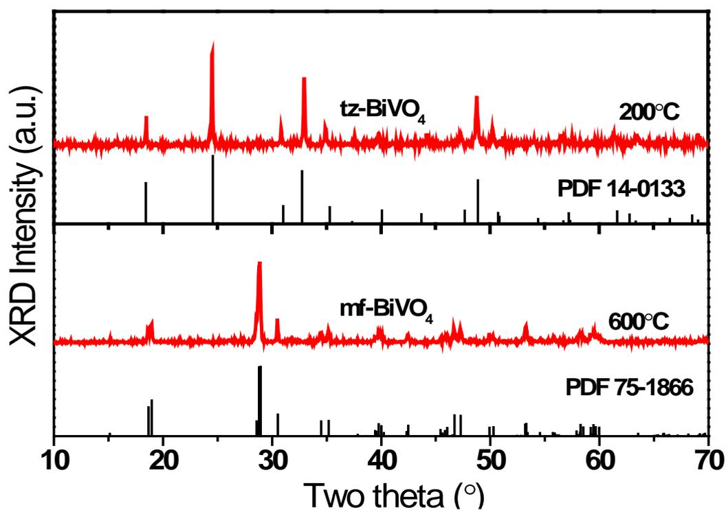
**Figure S1.** XRD patterns of fergusonite- and zircon-type BiVO<sub>4</sub> synthesized using a hydrothermal method.
