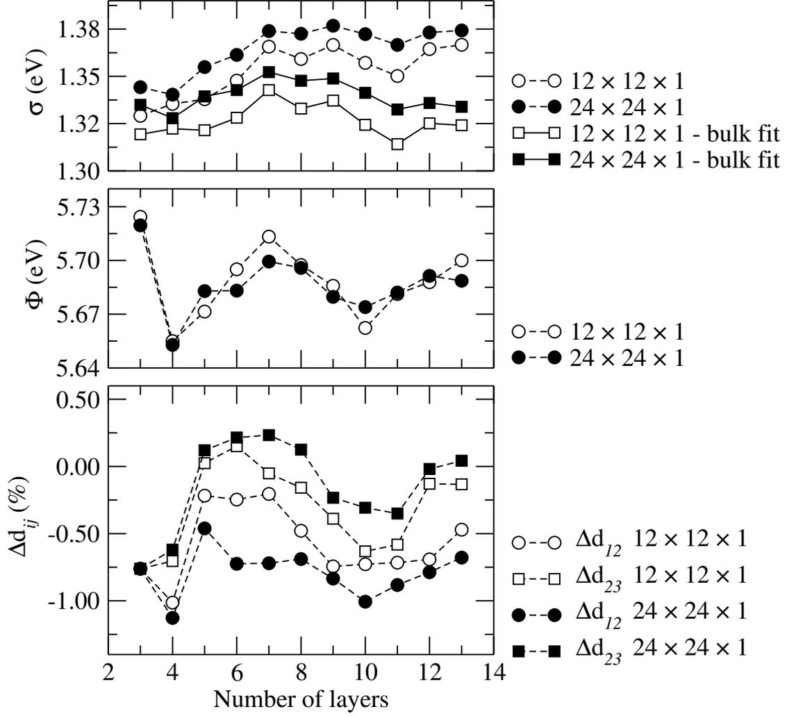
Figure S6: Surface energy  $\sigma$ , work function  $\Phi$  and interlayer spacing  $\Delta d_{ij}$  as functions of the number of layers using the  $12 \times 12 \times 1$  (open circles and squares) and  $24 \times 24 \times 1$  (closed circles and squares) k-points meshes for the Pt(100) slab.
