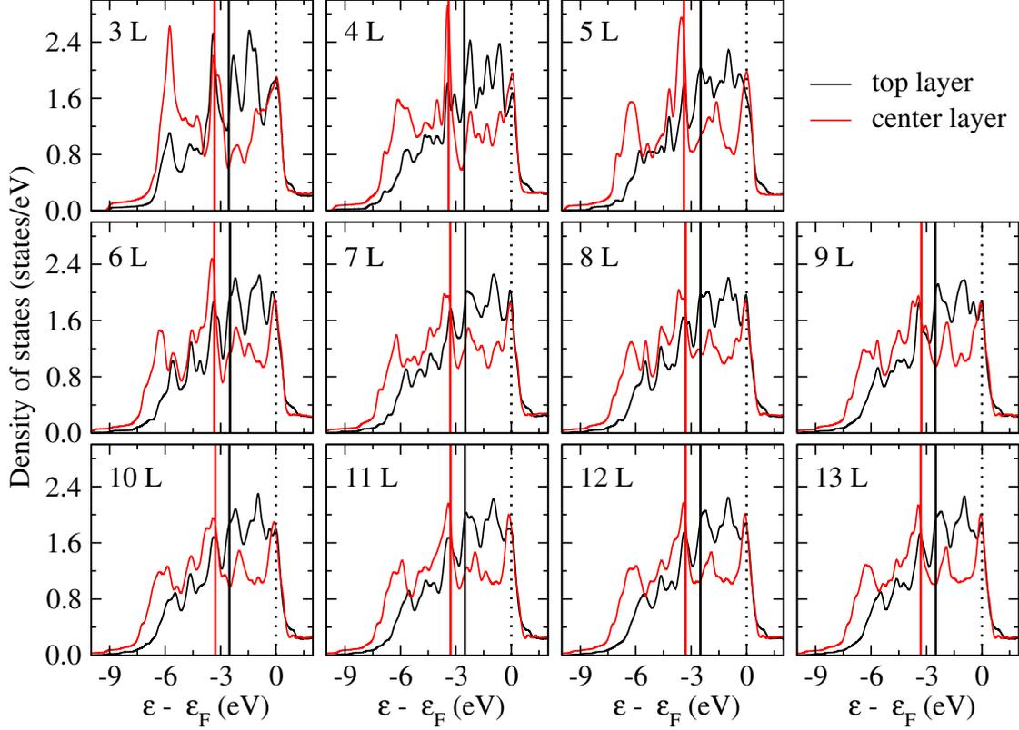
Figure S7: Density of states for the top and center layers of the Pt(100)-1 $\times$ 1 slab with  $N$  layers. The vertical solid lines indicates the  $d$ -band center for the respective layers and the dashed line indicates the Fermi level energy.
