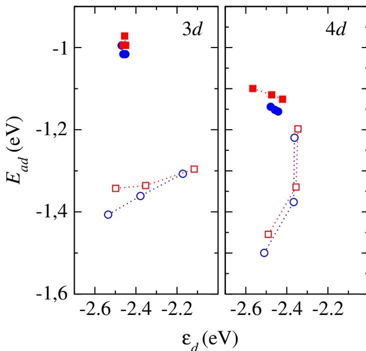
**Figure S20: Relationship between the adsorption energy  $E_{ad}$  and the average  $d$ -band center of the occupied  $d$ -states for TM atoms interacting with the molecule for the lowest energy configurations that differ in the number of atoms adsorbed on surfaces and in the two types of substrates (with the dopant positions on surface and subsurface).**
