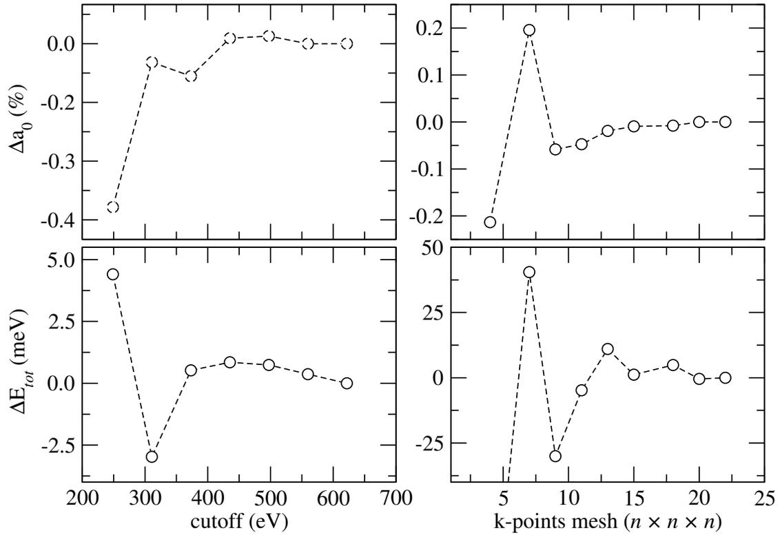
**Figure S1:** Convergence tests for the lattice parameter and total energy with respect to the plane-wave cutoff energy and  $\mathbf{k}$ -mesh for face-centered cubic Pt bulk.
