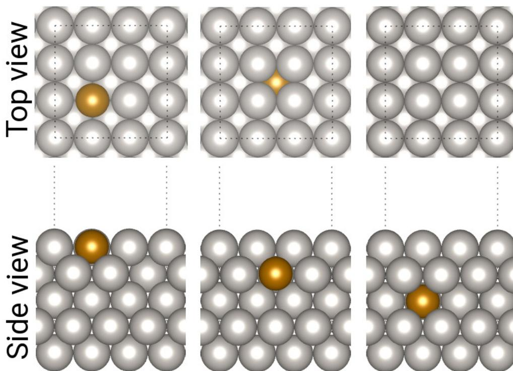
Figure S8: Configurations for clean PtFe(100) surface illustrating three positions studied for the TM dopants.
