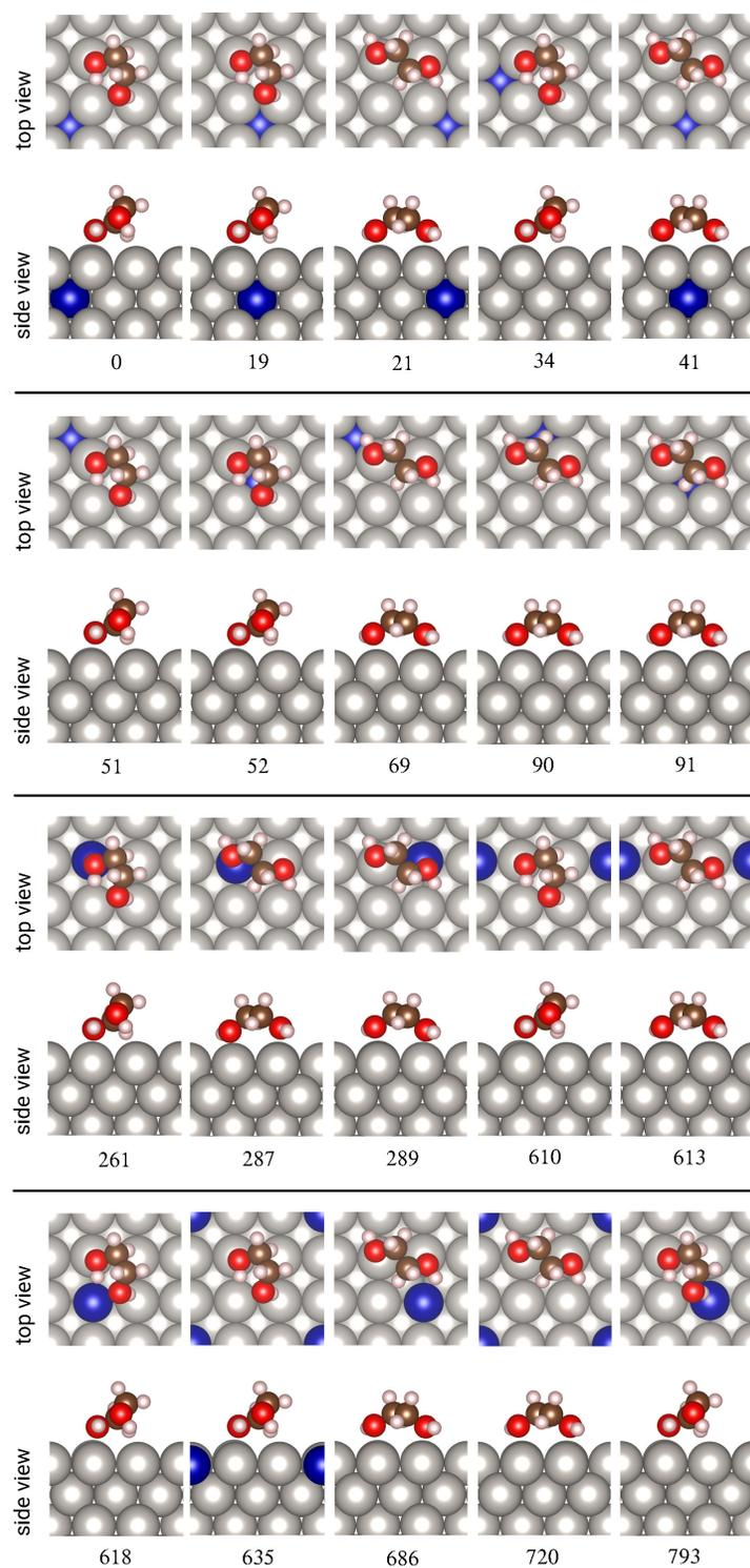
Figure S14: EG/Pt<sub>9</sub>/Pt<sub>8</sub>Co<sub>1</sub>/Pt(100) and EG/Pt<sub>8</sub>Co<sub>1</sub>/Pt<sub>9</sub>/Pt(100) configurations and their relative energies (meV) with respect to the lowest energy configuration.
