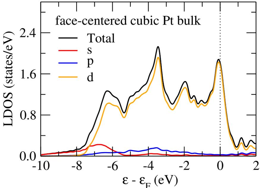
**Figure S2:** Local density of states (LDOS) for bulk Pt in the face-centered cubic structure. The total density of states (black line) is decomposed into *s*- (red line), *p*- (blue line) and *d*-states (orange line). The Fermi energy is indicated by the vertical dashed line.
