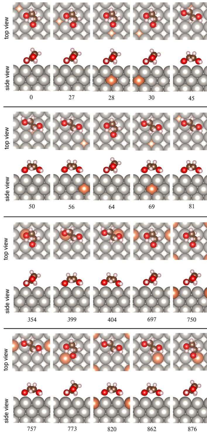
Figure S16: EG/Pt<sub>9</sub>/Pt<sub>8</sub>Ru<sub>1</sub>/Pt(100) and EG/Pt<sub>8</sub>Ru<sub>1</sub>/Pt<sub>9</sub>/Pt(100) configurations and their relative energies (meV) with respect to the lowest energy configuration.
