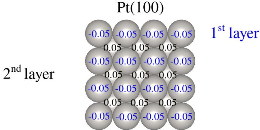
**Figure S10: Top view of the Pt(100) surface showing the effective Bader charges of each atom for the two topmost layers of the Pt(100) slab.**
