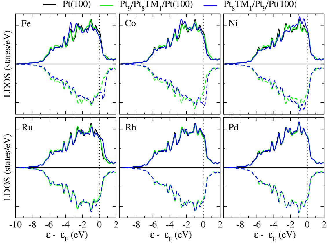
Figure S9: Local density of states (LDOS) for the topmost layer of the clean Pt(100), Pt<sub>9</sub>/Pt<sub>8</sub>TM<sub>1</sub>/Pt(100) and Pt<sub>8</sub>TM<sub>1</sub>/Pt<sub>9</sub>/Pt(100) surfaces. For Pt(100), the LDOS curve of the topmost layer is divided by 2 because is a no spin polarization calculation. The vertical dashed lines indicate the Fermi level.
