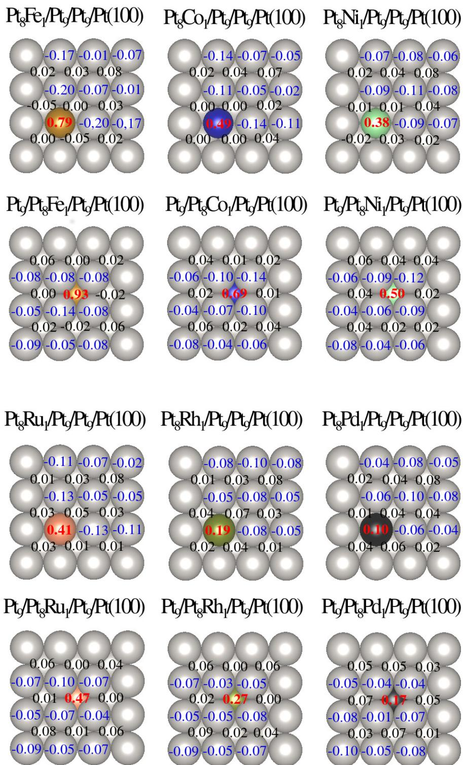
Figure S11: Top view of the surface slabs showing the effective charges for the clean  $\text{Pt}_9/\text{Pt}_8\text{TM}_1/\text{Pt}(100)$  and  $\text{Pt}_8\text{TM}_1/\text{Pt}_9/\text{Pt}(100)$  surface and subsurface layers.
