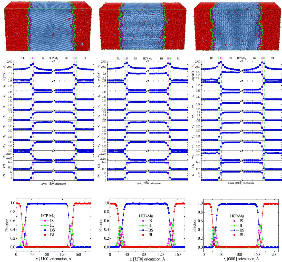
**Figure S6.** Three representative snapshots of HCP-Mg with the CBS layer-wise profiles of atom number  $N_a$ ; the density  $\rho$ ; BOO parameters (i.e.  $q_4$ ,  $q_6$ ,  $w_4$ , and  $w_6$ ); ABOO parameters (i.e.  $aq_4$ ,  $aq_6$ ,  $aw_4$  and  $aw_6$ ); coordinate number (CN); and Frenkel number (FN). Also exhibited are the fraction distributions of four atom types.
