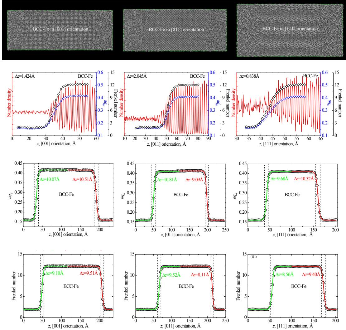
**Figure S2.** Three representative snapshots, the decaying oscillation of number density, and the slice-wise profiles of  $aq_6$  and FN and their hyperbolic tangent fittings of BCC-Fe based on the framework of “layering and in-plane ordering”.
