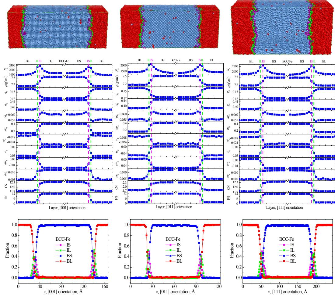
**Figure S5.** Three representative snapshots of BCC-Fe with the CBS layer-wise profiles of atom number  $N_a$ ; the density  $\rho$ ; BOO parameters (i.e.  $q_4$ ,  $q_6$ ,  $w_4$ , and  $w_6$ );
