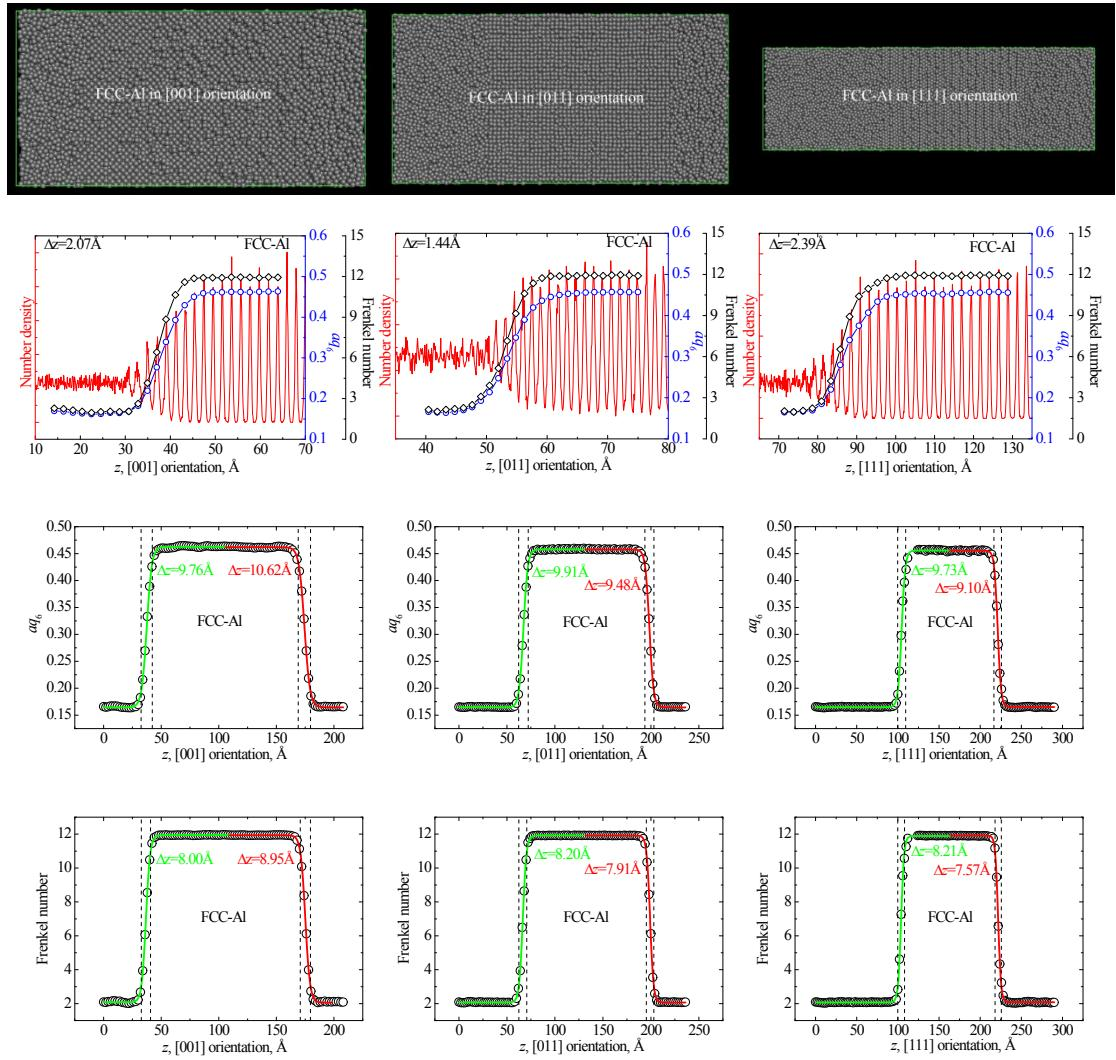
**Figure S1.** Three representative snapshots, the decaying oscillation of number density, and the slice-wise profiles of  $aq_6$  and FN and their hyperbolic tangent fittings of FCC-Al based on the framework of “layering and in-plane ordering”.
