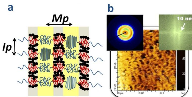
**Figure S5.** (a) Schematic representation of the lamellar stacking of ionic and nonionic domains, indicating the matrix ( $M_p$ ) and ionomer ( $I_p$ ); and (b) AFM phase image of commercial extruded Nafion (N115) film surface in the  $150 \times 150 \text{ nm}^2$  window. The insets show the N115 weak anisotropic 2D pattern alongside the Fourier Transform of the topography.
