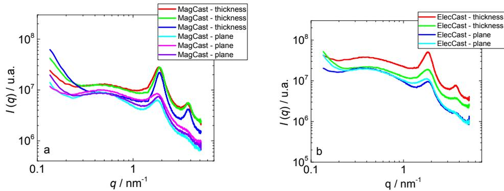
**Figure S3.** SAXS plots of dry Nafion-H<sup>+</sup> prepared by magnetic (a) and electric (b) field assisted casting.
