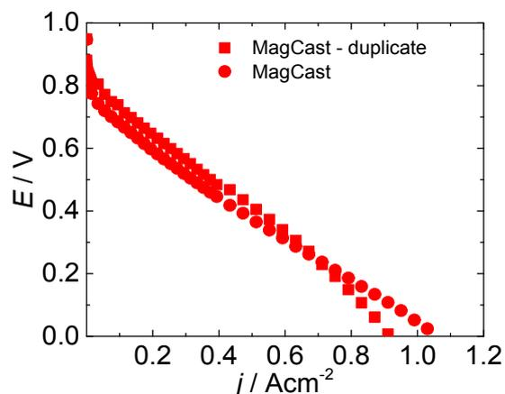
**Figure S9.**  $H_2/O_2$  polarization curve for MagCast in duplicate at 80 °C and RH = 100%
