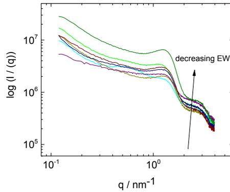
**Figure S2.** SAXS plots of hydrated Nafion-Cs<sup>+</sup> with increasing EW.
