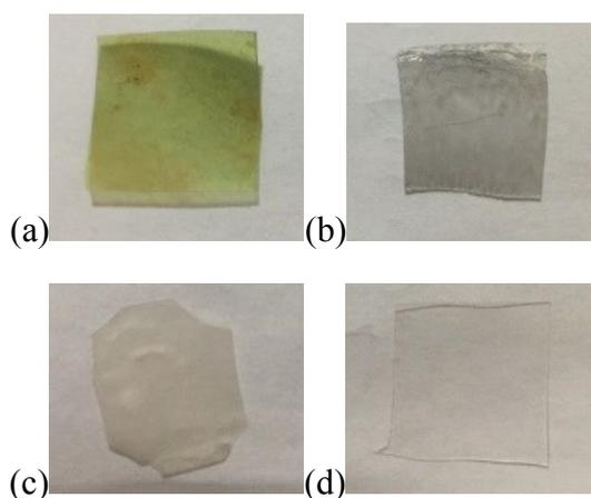
**Figure S10.** ElecCast (a), MagCast (b), Cast (c) and extruded Nafion 115 (d).
