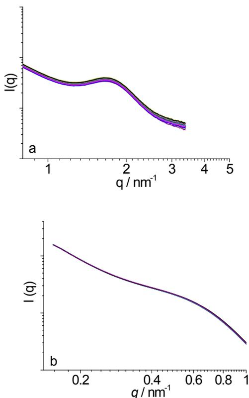
**Figure S1.** Time-resolved SAXS measurements of Nafion in 50 frames of 200s: (a) ionomer and (b) matrix peaks.
