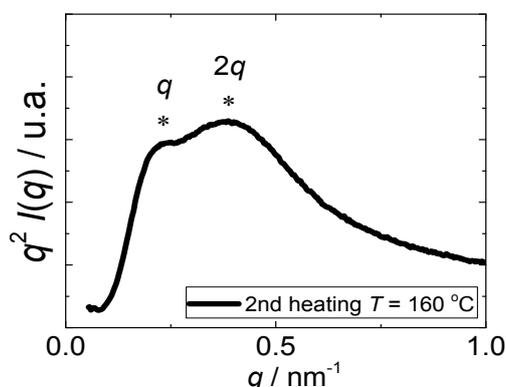
**Figure S4.** Kratky plot of **Fig. 2d** SAXS plot at 160 °C.
