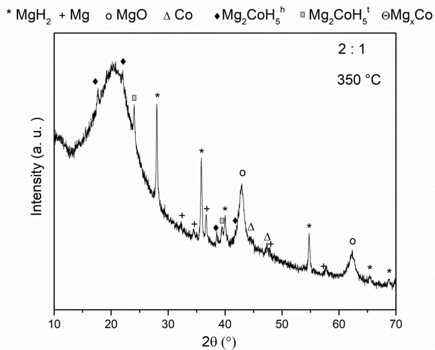
Figure S6: XRPD profile of the sample MgH<sub>2</sub>-10%wt Co after thermal treatment under CO<sub>2</sub> at 350°C, 24 h (molar ratio MgH<sub>2</sub>:CO<sub>2</sub> of 2:1).
