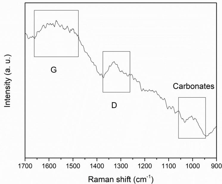
Figure S1: Raman spectrum of MgH<sub>2</sub> after thermal treatment with CO<sub>2</sub> at 400°C for 24 h (molar ratio of 2:1).
