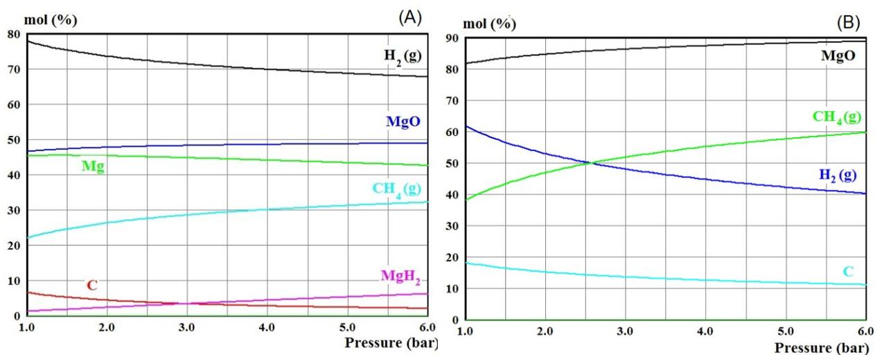
Figure S8: Equilibrium composition (mol%) as a function of pressure at  $450^\circ\text{C}$  for a molar ratio  $\text{MgH}_2:\text{CO}_2$  of 4:1 (A) and 2:1 (B).
