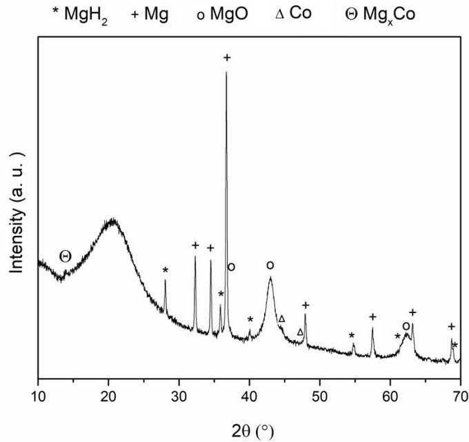
Figure S5: XRPD pattern of the sample  $\text{MgH}_2$ -10%wt Co with a molar ratio  $\text{MgH}_2$ : $\text{CO}_2$  of 4:1 (Co milled during the last 10 minutes).
