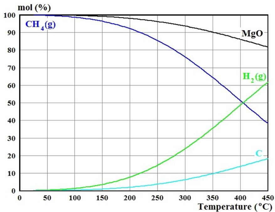
Figure S9: Equilibrium composition (mol %) as a function of temperature at 1bar for molar ratio MgH<sub>2</sub>:CO<sub>2</sub> of 2:1.
