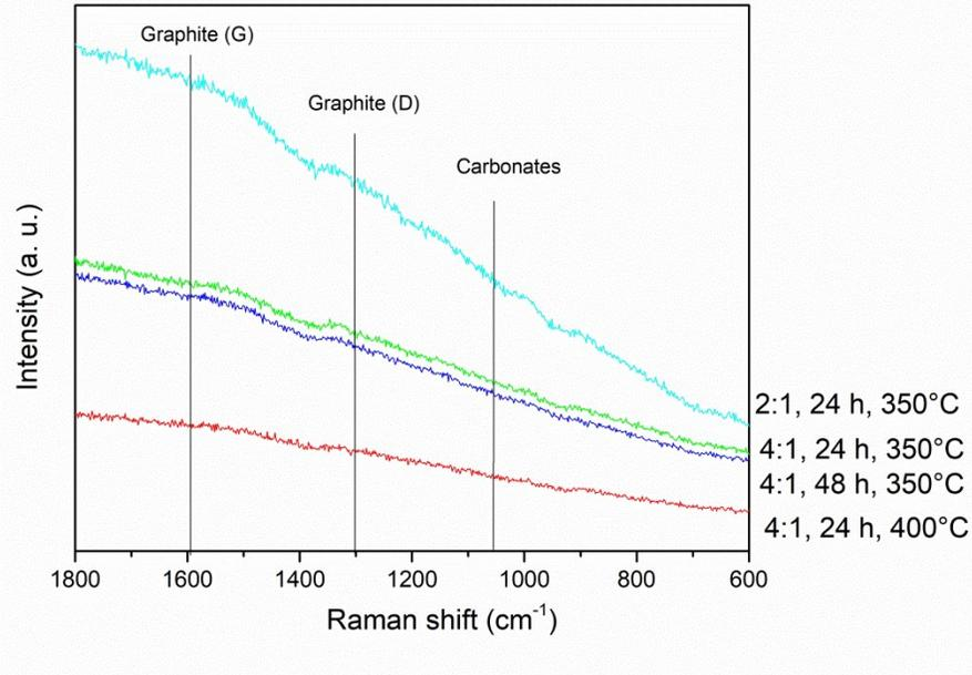
Figure S4: Raman spectra of  $\text{MgH}_2$ -10%Co after reaction with  $\text{CO}_2$  considering different experimental conditions.
