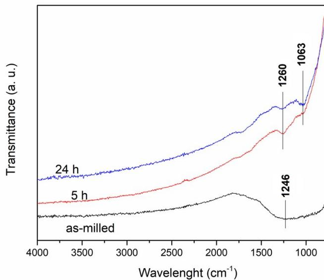
Figure S3: Solid-state FTIR profiles for the as milled MgH<sub>2</sub>-10%Co and after thermal treatment (400°C, 5 and 24h) under CO<sub>2</sub> (molar relation of 4:1).
