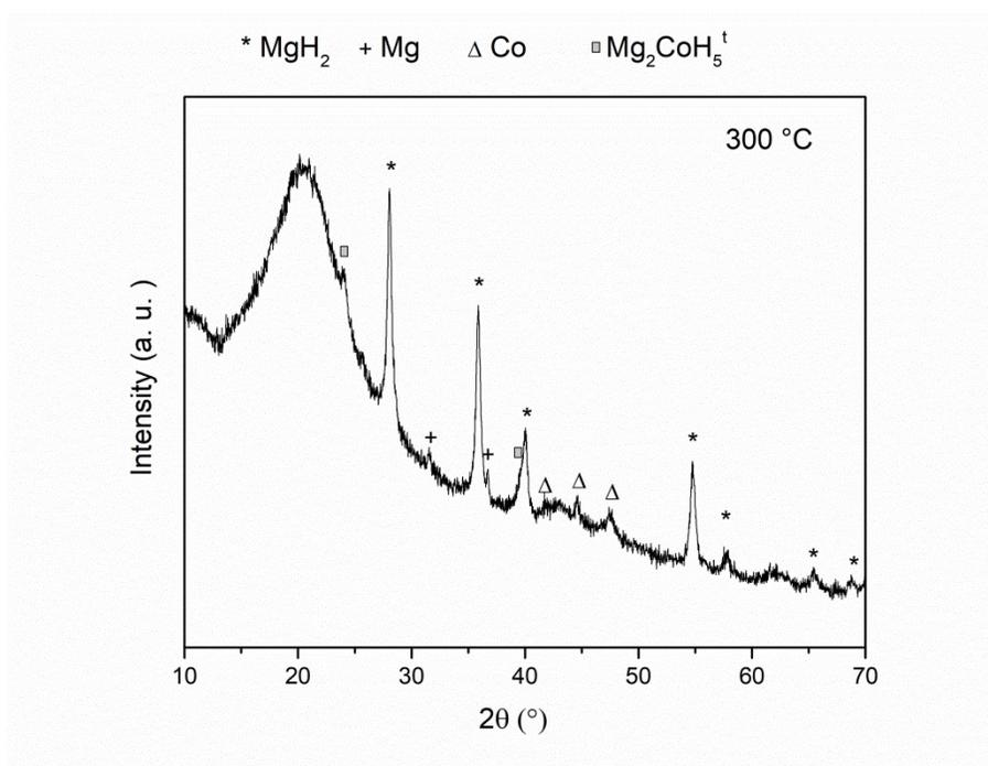
Figure S7: XRPD profile of the sample  $\text{MgH}_2$ -10%wt Co at  $300^\circ\text{C}$  with a molar ratio  $\text{MgH}_2:\text{CO}_2$  of 4:1.
