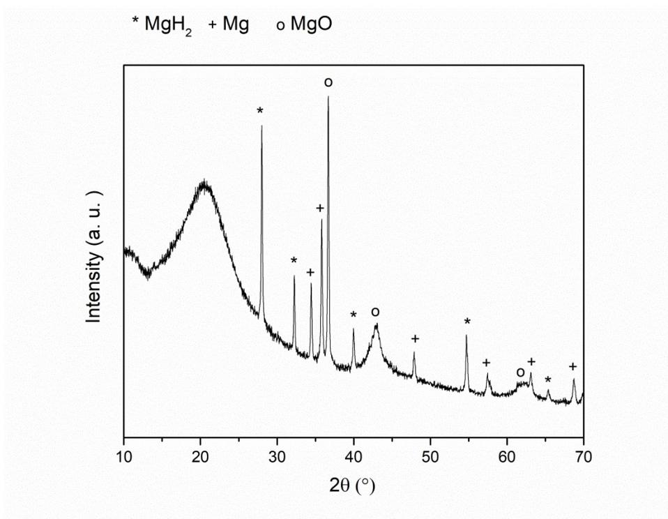
Figure S2: XRPD pattern of MgH<sub>2</sub> after thermal treatment with CO<sub>2</sub> at 350°C for 24 h (molar relation of 2:1).
