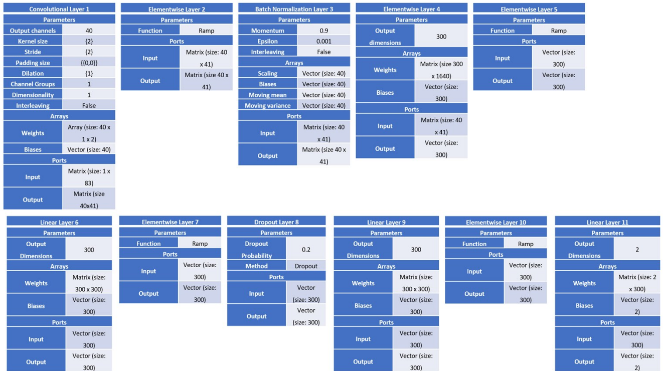
Figure S9. Au absorber specific NN architecture as implemented in Mathematica 12. The layers are connected sequentially from 1 to 11.
