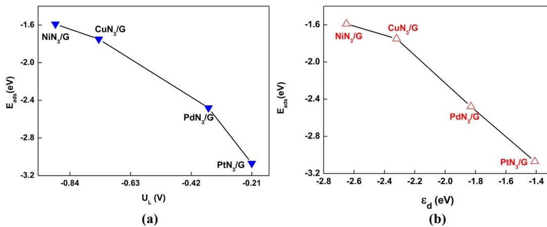
**Fig. S3.** Calculated adsorption energy ( $E_{\text{ads}}$ ) plotted versus (a) limiting potential ( $U_L$ ) and (b) d-band center ( $\epsilon_d$ ).
