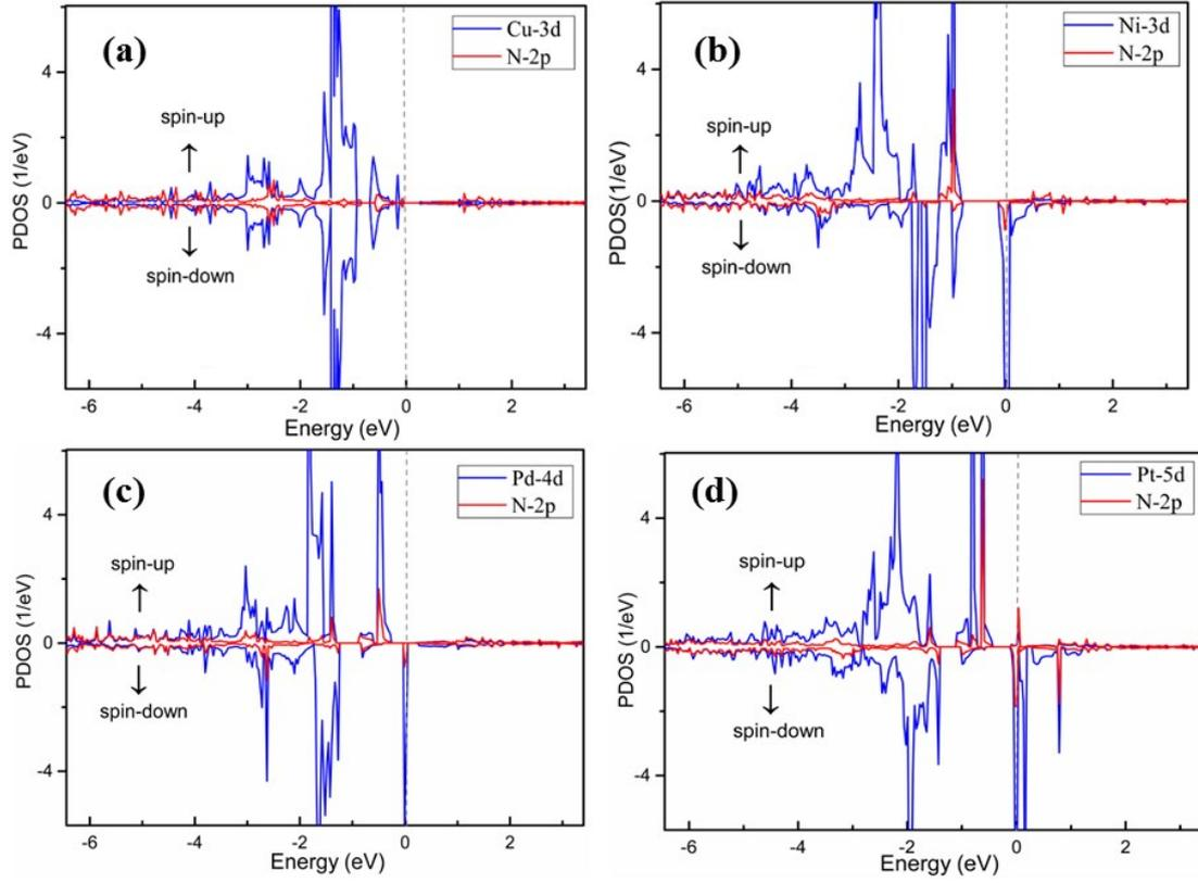
**Fig. S1.** The computed projected density of states (PDOSs) of (a) CuN<sub>3</sub>/G, (b) NiN<sub>3</sub>/G, (c) PdN<sub>3</sub>/G, and (d) PtN<sub>3</sub>/G. The Fermi level was set to zero.
