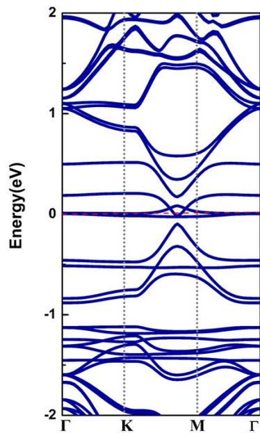
**Fig. S5.** The computed band structure of PtN<sub>3</sub>/G. The Fermi level is set to zero in red dashed line.
