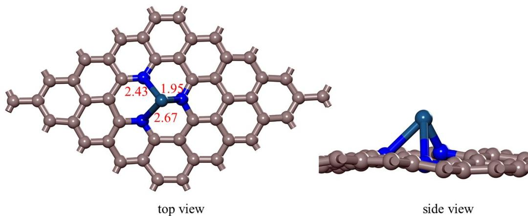
**Fig. S4.** Snapshots of PtN<sub>3</sub>/G equilibrium structure at 500 K after 10 ps MD simulations.
