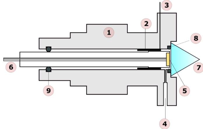
Figure S1: Schematic representation of the cell used to perform in situ FT-IR spectra. 1) Body of the cell, shaped to fit the holder. 2) Pt foil counter electrode. 3) Counter-electrode contact made of Pt wire. 4) Aperture for the reference electrode. 5) Au working electrode. 6) Screw as contact for the Au electrode. 7)  $\text{CaF}_2$  prism as the window. 8) and 9) O-rings.
