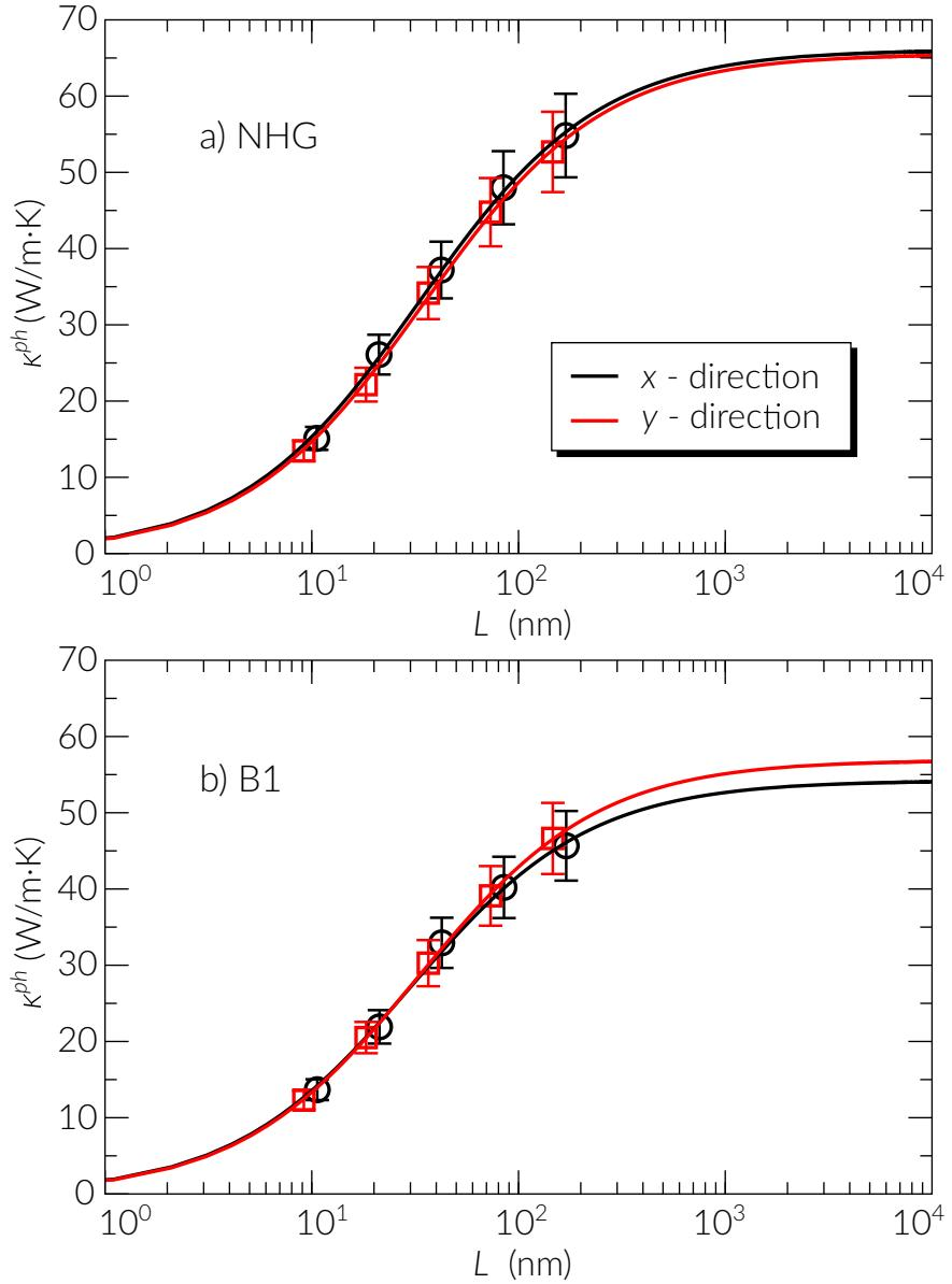
FIG. 2. Size dependence of the thermal conductivity obtained from molecular dynamics simulations.
