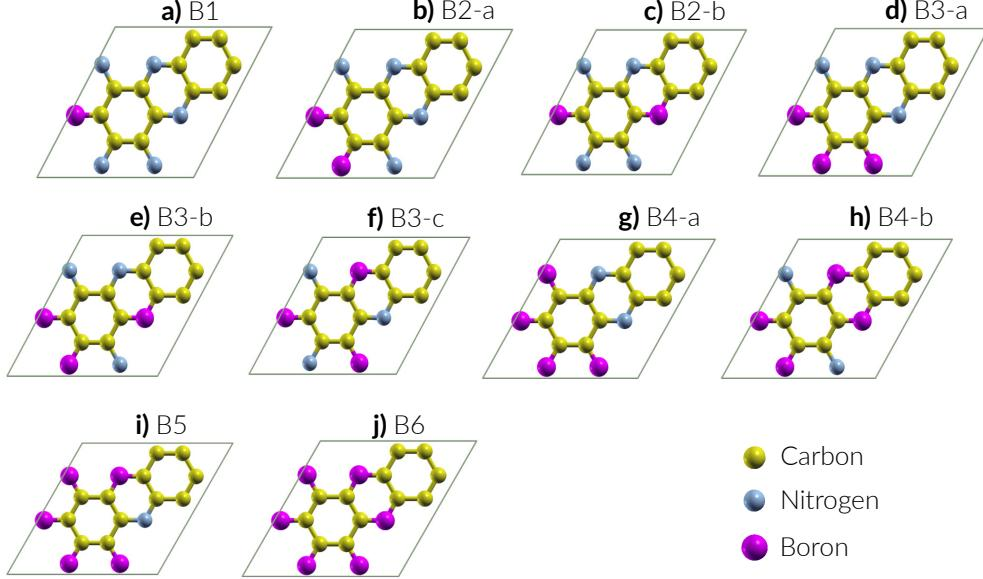
FIG. 1. Unit cell of the boron doped NHG monolayers. The number of boron substitutions ranges from 1 to 6.
