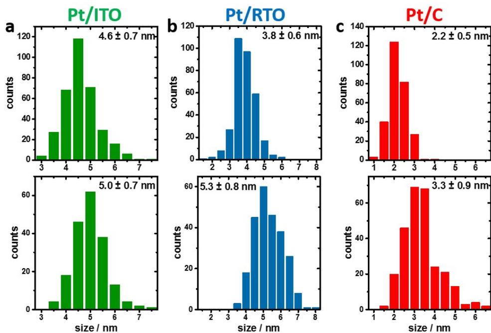
**Figure S3** Histograms of mean particle diameter for Pt supported on (a) ITO (green), (b) RTO (blue) and (c) carbon (red) support. Top row shows the average particle diameter measured along their shortest particle axis and bottom row along their longest particle axes.
