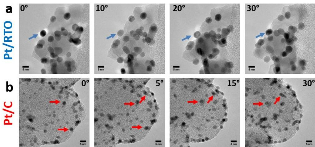
**Figure S4** Morphology of Pt nanoparticles on a) RTO (blue) and b) carbon (red) support in a TEM tilting study from 0-30°.
