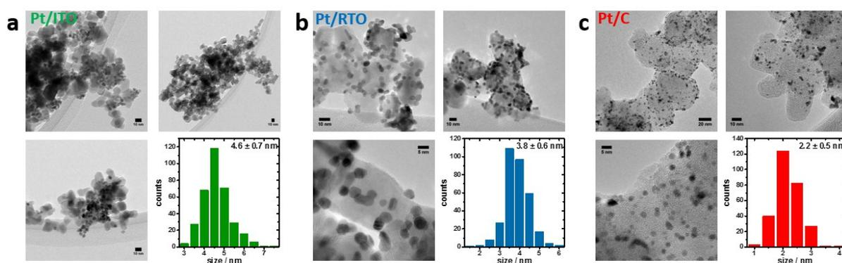
**Figure S2** Morphology of Pt nanoparticles on a) ITO (green), b) RTO (blue) and c) carbon (red) support and corresponding histograms showing mean particle diameter as determined by transmission electron microscopy. The particle size histogram was determined from analyzing > 200 particles along their shortest particle axes.
