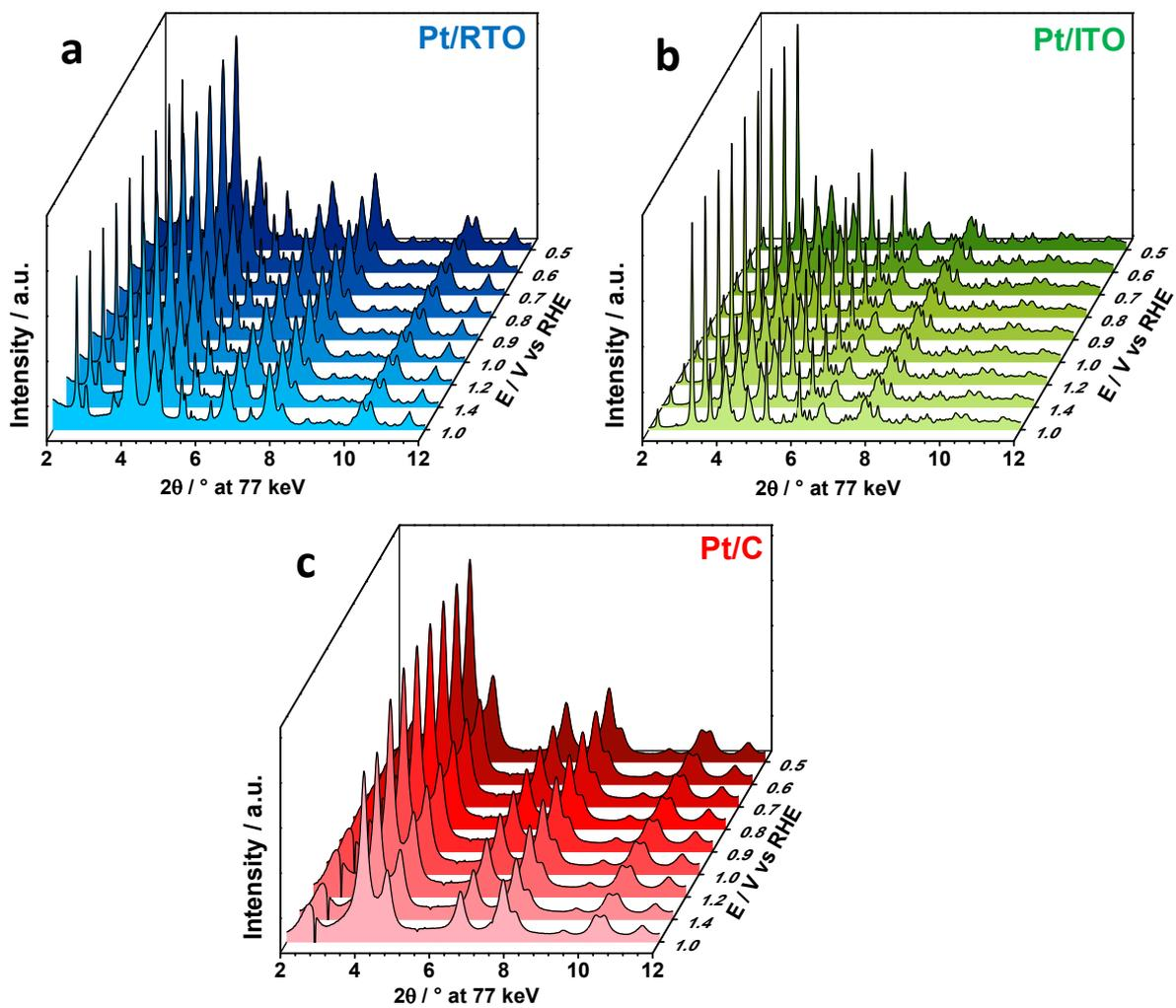
**Figure S6** *In situ* high-energy X-ray diffraction patterns of Pt nanoparticles supported on ITO (green, a), RTO (blue, b) and carbon (red, c) as recorded during the electrochemical oxidation of Pt.
