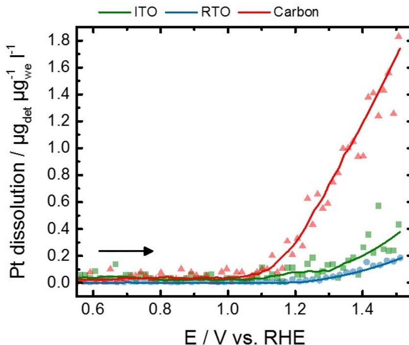
**Figure S9** Evolution of mass-normalized Pt dissolution rate as determined by SFC-ICP-MS measurements during the initial anodic potential sweep from 0.05-1.5 V for Pt nanoparticles supported on ITO (green), RTO (blue), and carbon (red).
