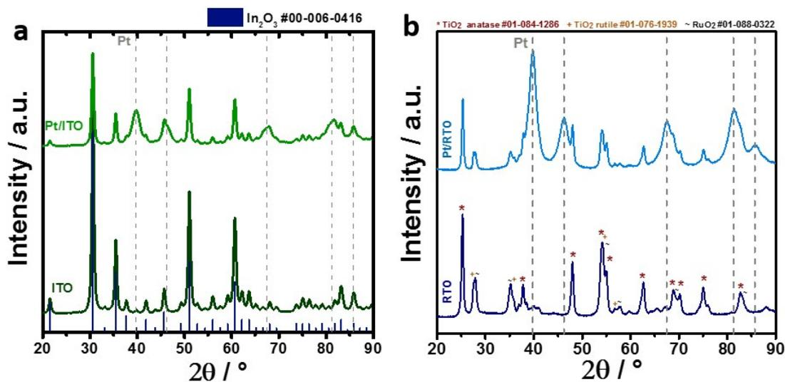
**Figure S1** X-ray diffractograms of (a) ITO and Pt/ITO with solid blue lines indicating In<sub>2</sub>O<sub>3</sub> reference pattern and (b) RTO and Pt/RTO with symbols indicating TiO<sub>2</sub> anatase and rutile and RuO<sub>2</sub>. Vertical dashed lines denote reference powder diffraction patterns of fcc Pt (PDF#00-004-0802). XRDs were obtained using Cu K<sub>α</sub> radiation.
