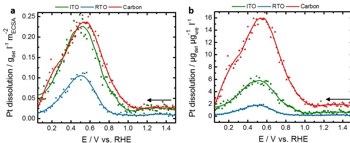
**Figure S10**  $H_{\text{upd}}$ -ECSA-normalized (a) and mass-normalized (b) Pt dissolution rate of electrochemically-oxidized Pt nanoparticles supported on ITO (green), RTO (blue), and carbon (red) as determined by SFC-ICP-MS measurements during the cathodic potential sweep from 1.5-0.05 V after initial anodic potential sweep up to 1.5 V.
