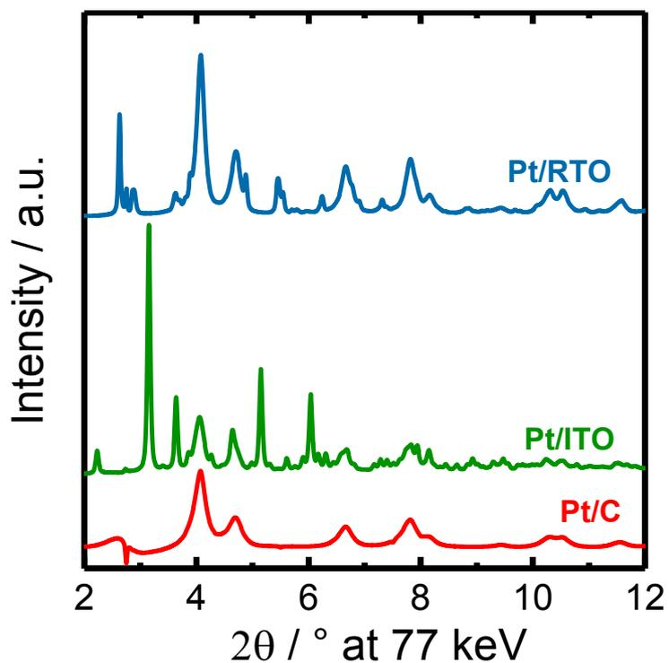
**Figure S5** High energy XRD patterns of Pt/RTO (blue), Pt/ITO (green) and Pt/C (red) in the as-prepared state.
