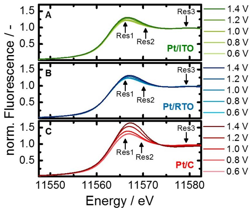
**Figure S7** Normalized *in situ* Pt  $L_3$ -edge X-ray near-edge absorption spectra for Pt nanoparticles supported on ITO (green, a), RTO (blue, b) and carbon (red, c) for potentials from 0.6 – 1.4 V of electrochemical oxidation of Pt. The positions of the Pt  $L_3$  resonances applied in the fit procedure are denoted.
