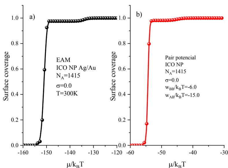
Figure S1: Adsorption isotherms for a clean ICO NP simulated with EAM Panel (a) and pairwise model (b)
