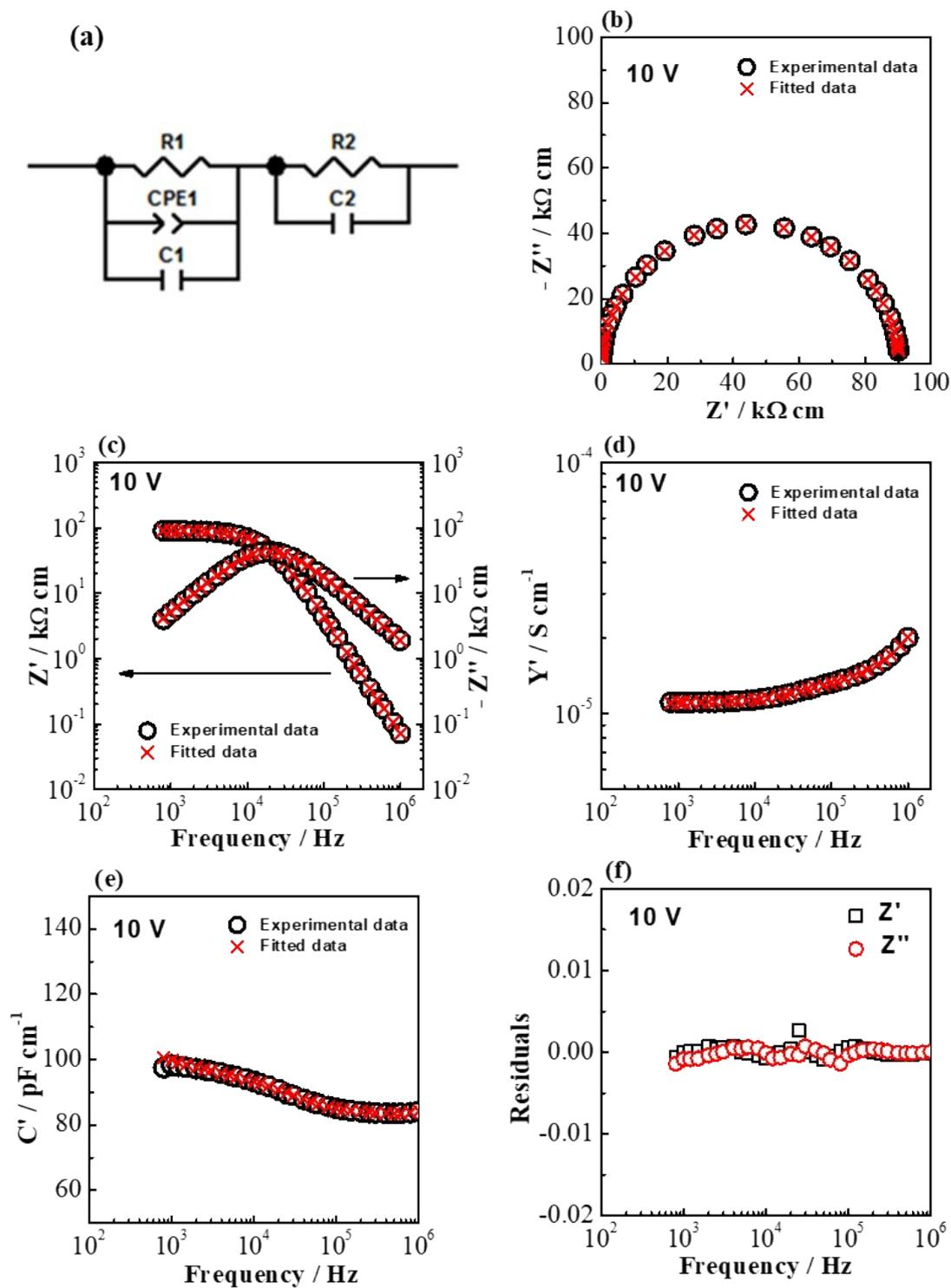
Figure S5. (a) Equivalent circuit used to fit impedance spectra of  $\text{NB}_{0.51}\text{T}$  under dc bias for 30 minutes; (b)- (e) impedance and fitting results presented in different formats: (b)  $Z^*$ , (c)  $Z'$ - $\log f$  and  $Z''$ - $\log f$ , (d)  $Y'$ - $\log f$  and (e)  $C'$ - $\log f$ ; (f) impedance residuals showing the quality of fit. Measurement was carried out at 600 °C in air.
