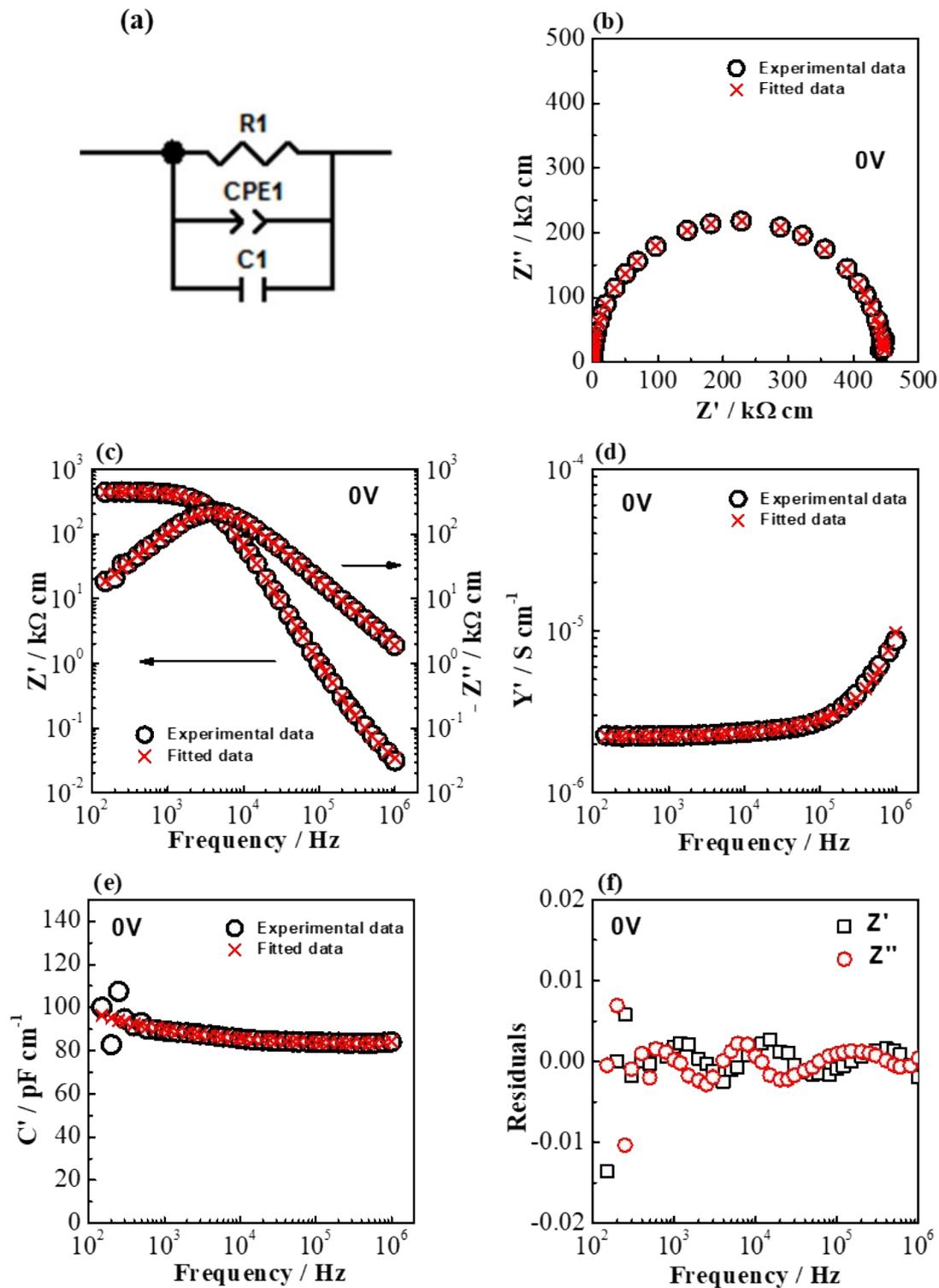
Figure S4. (a) Equivalent circuit used to fit impedance spectra of  $\text{NB}_{0.51}\text{T}$  without dc bias; (b)-(e) impedance and fitting results presented in different formats: (b)  $Z^*$ , (c)  $Z'$ - $\log f$  and  $Z''$ - $\log f$ , (d)  $Y'$ - $\log f$  and (e)  $C'$ - $\log f$ ; (f) impedance residuals showing the quality of fit. Measurement was carried out at  $600\text{ }^\circ\text{C}$  in air.
