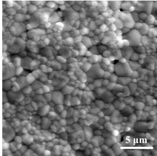
Figure S2. An SEM image of a thermally-etched surface of an  $\text{NB}_{0.51}\text{T}$  ceramic.
