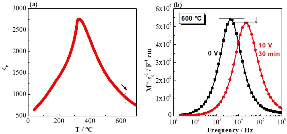
Figure S3. (a) Temperature dependence of permittivity of  $\text{NB}_{0.51}\text{T}$  at 1 MHz. The arrow in the figure indicates a decrease of permittivity with a temperature rise from 600 to 630 °C. (b) Comparison of the  $M''$  peak height before and after applying a 10 V dc bias for 30 min.
