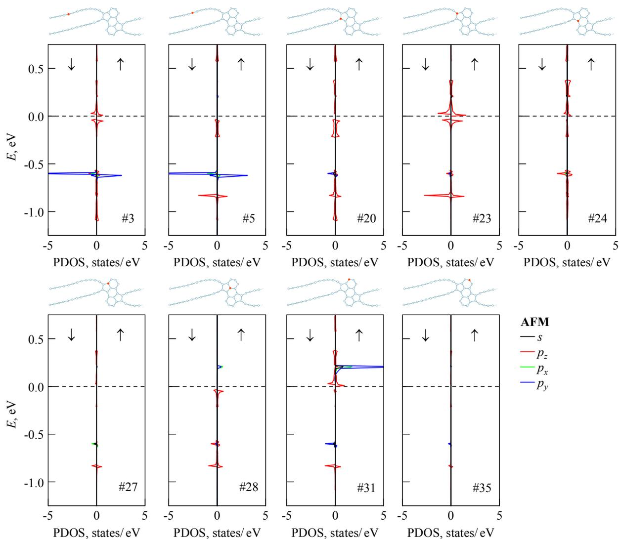
**Figure S3.** Calculated projected densities of states for selected atoms of the 1D nanoobject with D1 polycyclic regions (as indicated in the atomistic structures) in the antiferromagnetic state. The energies in eV are given relative to the Fermi level. The results for  $s$ ,  $p_z$ ,  $p_x$  and  $p_y$  orbitals are shown by black, red, green and blue lines, respectively.
