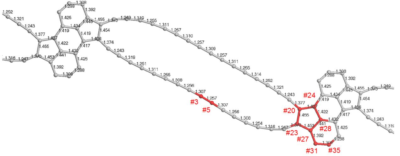
**Figure S2.** Geometrically optimized structure of the 1D nanoobject with D1 polycyclic regions obtained by the DFT calculations. The bond lengths (in Å) are indicated in grey. The atoms for which the partial densities of states are computed are shown in red.
