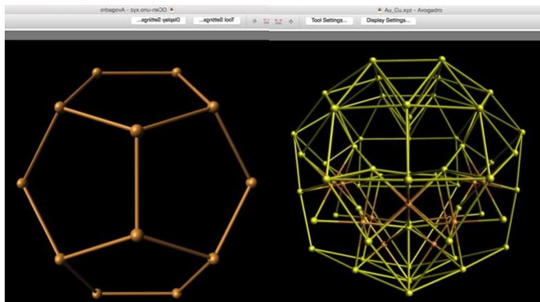
**Figure S1.** Centre of 12 octahedra forming an arrangement of four pentagonal rings fused as in the dodecahedron. To the right is depicted the distribution of the octahedral blocks in the total structure of the  $2+ \text{Au}_{60}$  cluster.
