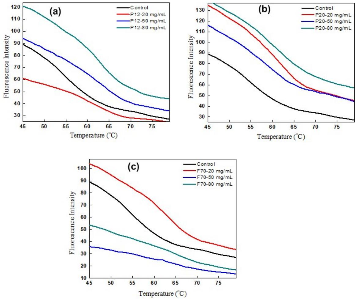
**Fig. S6.** The thermal transition curve of BSA in absence and presence of varying concentrations of (a) P12, (b) P20 and (c) F70 in phosphate buffer of pH 7.
