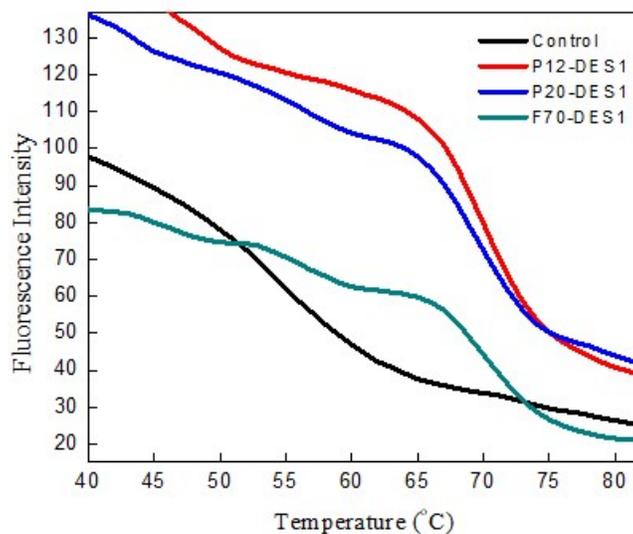
**Fig. S7.** The thermal transition curve of BSA in absence and presence of mixture of DES1 with different crowders (50 mg/mL each) in phosphate buffer of pH 7.
