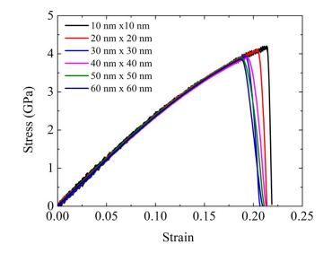
**FIGURE S1.** Demonstartion of tensile properties of beta bismuthene along with armchair direction considering different system size size at 300K at a strain rate of  $10^9$  (s<sup>-1</sup>)
