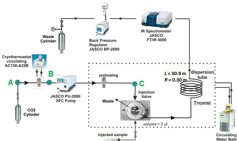
FIG. S1. Schematic of the high pressure Taylor dispersion apparatus.
