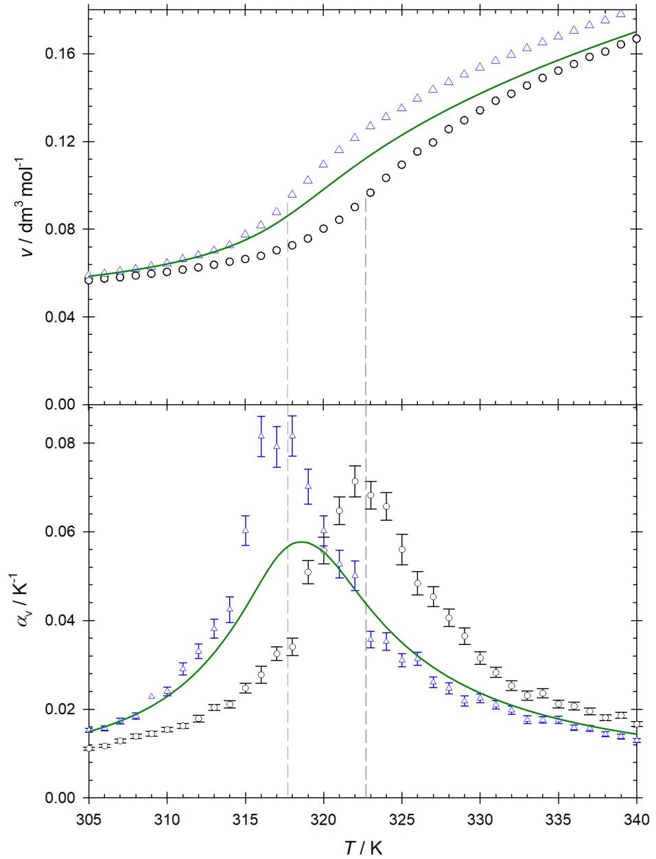
FIG. S3. Specific volume  $v$  and thermal expansion  $\alpha_v$  of  $\text{CO}_2$  (blue) and the mixture  $\text{CO}_2 + \text{ethanol}$  (black) along the isobar  $p = 10 \text{ MPa}$ . The green line represents the properties of pure  $\text{CO}_2$  calculated with the Span-Wagner equation of state [2].
