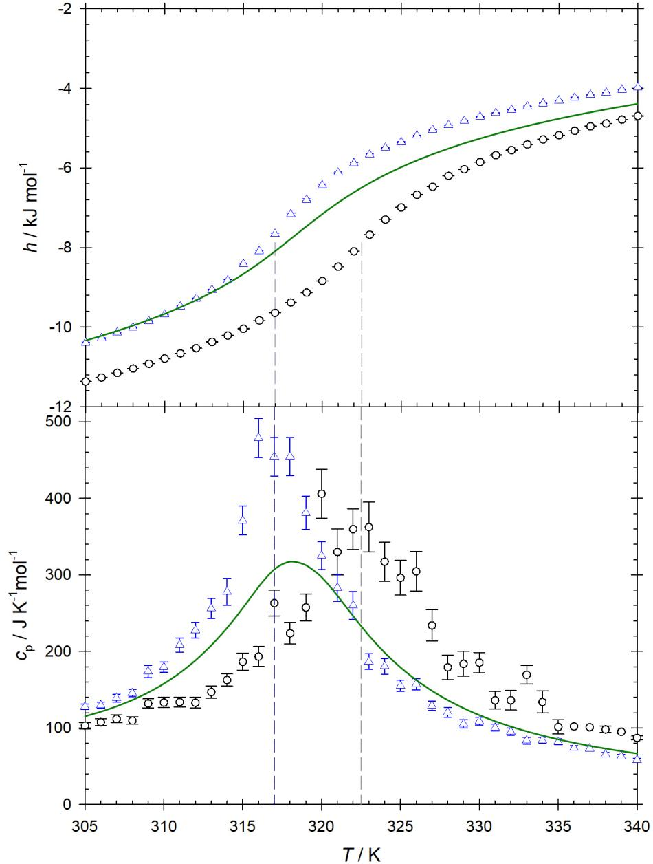
FIG. S2. Enthalpy  $h$  and isobaric heat capacity  $c_p$  of  $\text{CO}_2$  (blue) and the mixture  $\text{CO}_2 + \text{ethanol}$  (black) along the isobar  $p = 10$  MPa. The green line represents the properties of pure  $\text{CO}_2$  calculated with the Span-Wagner equation of state [2].
