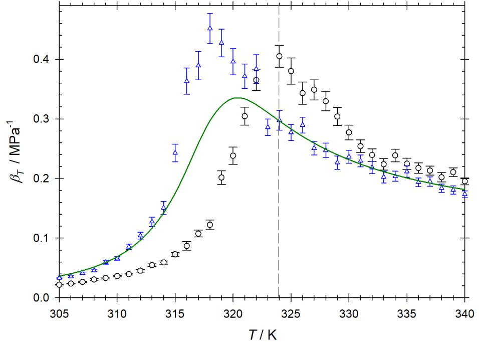
FIG. S4. Isothermal compressibility  $\beta_T$  of  $\text{CO}_2$  (blue) and the mixture  $\text{CO}_2 + \text{ethanol}$  (black) along the isobar  $p = 10 \text{ MPa}$ . The green line represents the isothermal compressibility of pure  $\text{CO}_2$  calculated with the Span-Wagner equation of state [2].
