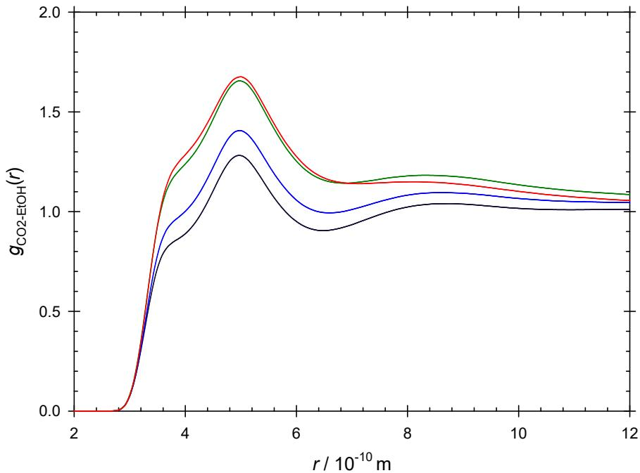
FIG. S5.  $\text{CO}_2$ -ethanol radial distribution function at  $T = 310 \text{ K}$  (black),  $320 \text{ K}$  (blue),  $330 \text{ K}$  (green) and  $340 \text{ K}$  (red) along the isobar  $p = 10 \text{ MPa}$ .
