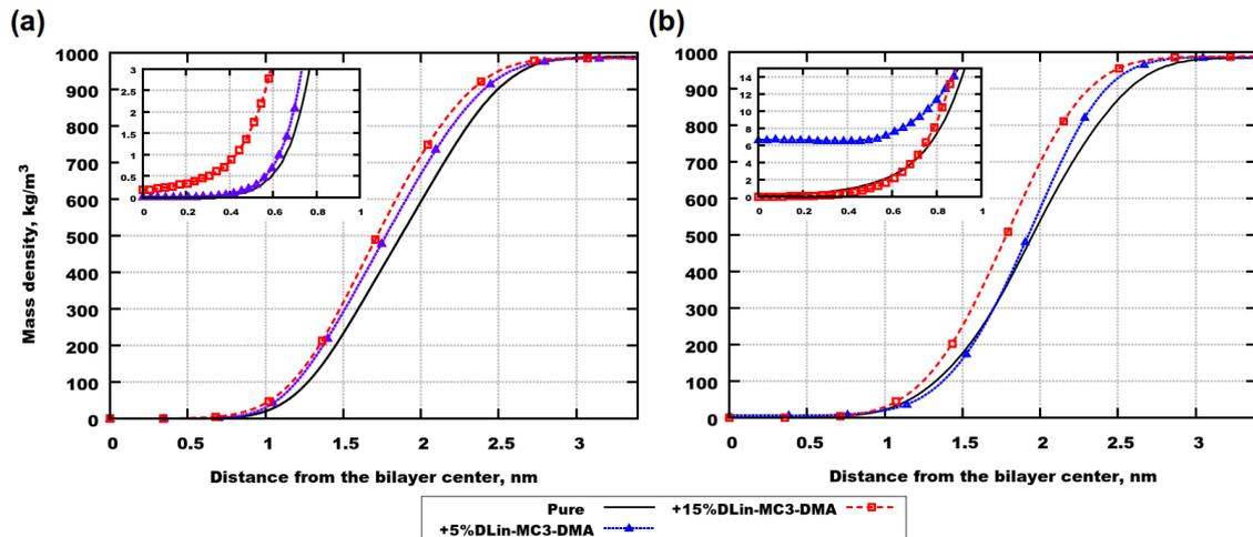
Figure S6: Mass density profiles for water molecules in the following systems: (a) DOPC (b) DOPE. Labels: "Pure" stands for lipid bilayers containing only phospholipids, +5% DLin-MC3-DMA means that it was 5% of the ionizable lipid and +15% DLin-MC3-DMA means that it was 15% of the ionizable lipid.
