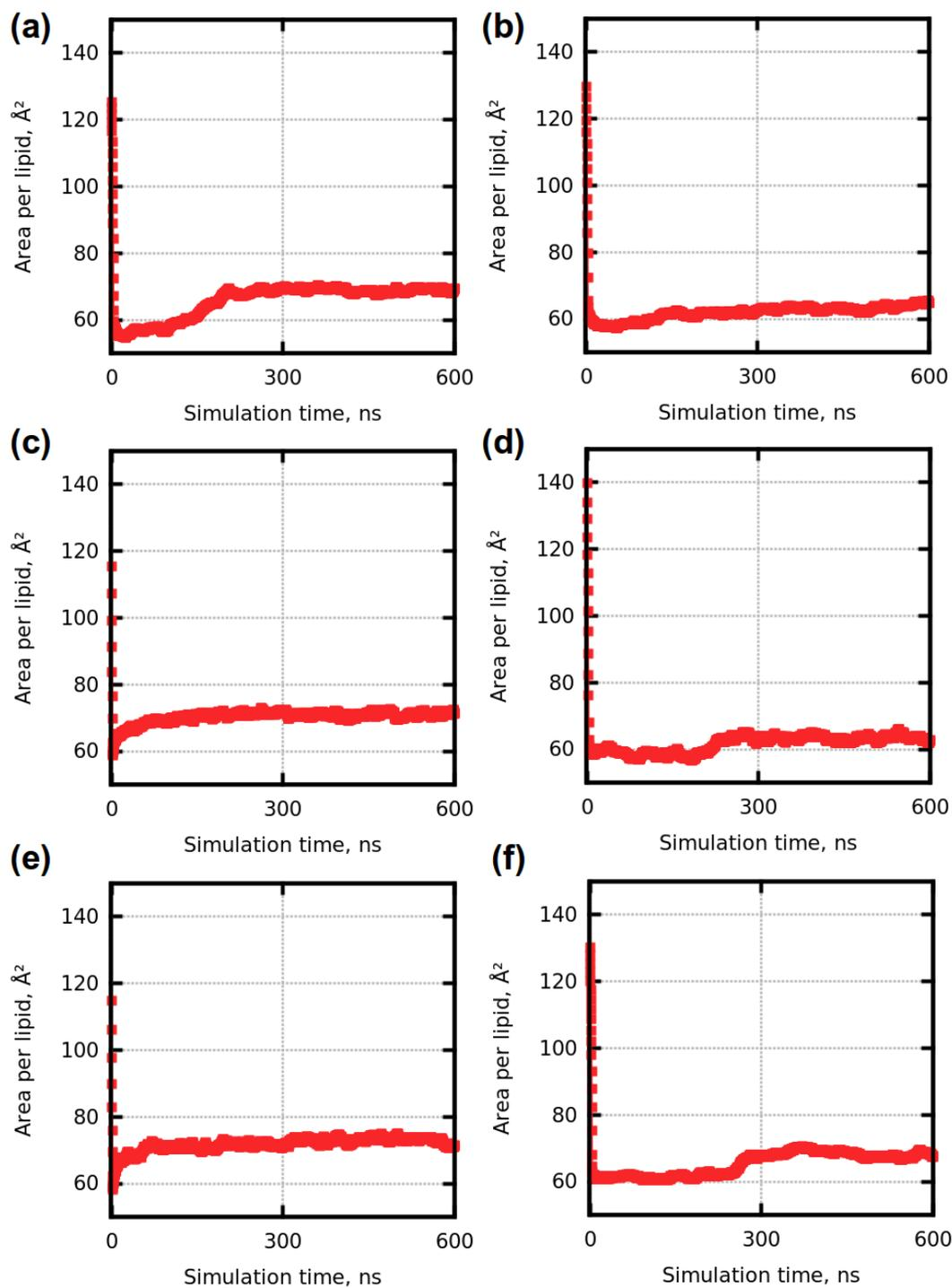
Figure S5: The area per lipid during the simulation time (a) DOPC (pure) (b) DOPE (pure) (c) DOPC with 5% of DLin-MC3-DMA (d) DOPE with 5% of DLin-MC3-DMA (e) DOPC with 15% of DLin-MC3-DMA (f) DOPE with 15% of DLin-MC3-DMA
