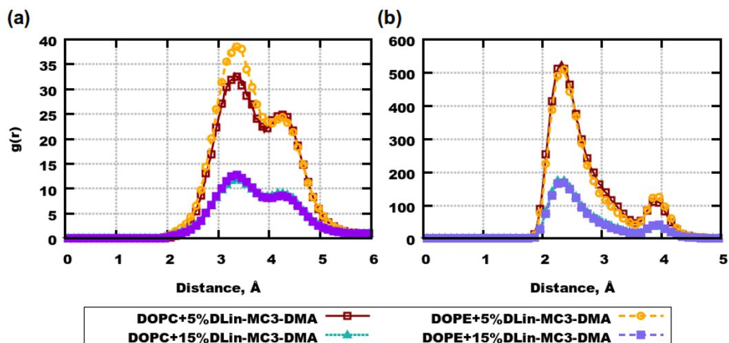
Figure S9: RDFs between pairs of atoms in the DLin-MC3-DMA head-group. (a) RDFs between hydrogens from the CH<sub>2</sub>-group labeled as "a" and oxygens. (b) RDFs between hydrogens from the CH<sub>3</sub>-group labeled as "b" and oxygens. Parts of the DLin-MC3-DMA lipid were colored in a following way: light gray color - hydrogen, dark gray - carbon, blue - nitrogen, red - oxygen.
