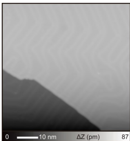
Figure S1 STM topography of an atomically clean Au(111) surface after cyclic Ar + sputtering for 10 min and annealing at 750 K for 15 min. This image was taken before depositing molecules. Measurement parameters: V = 200 mV and I = 10 pA.
