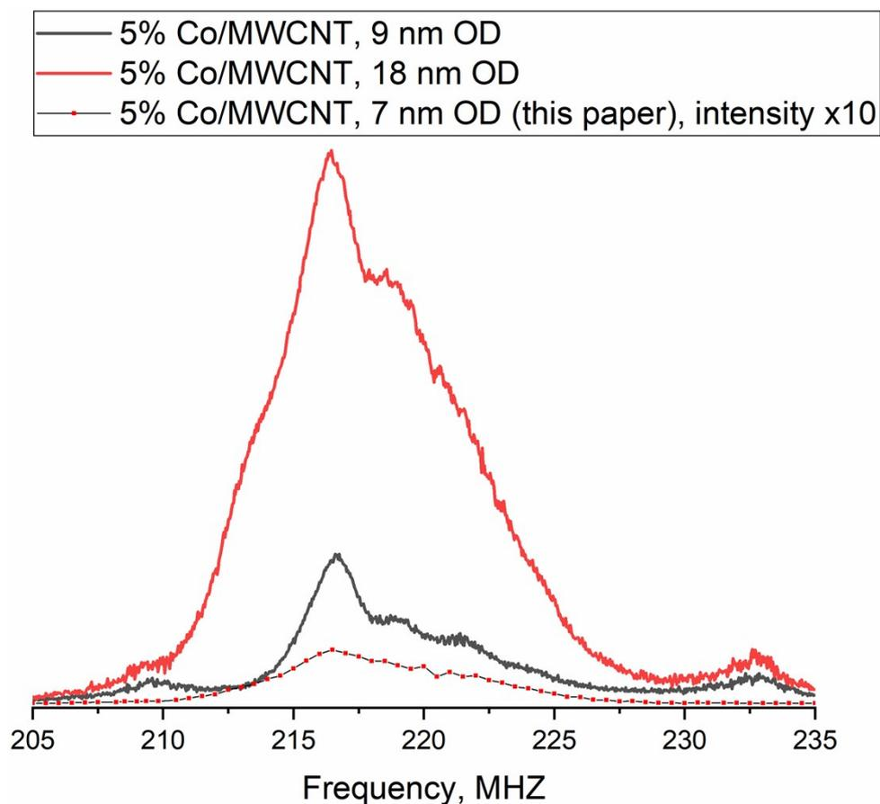
Figure S2. Comparison between room-temperature  $^{59}\text{Co}$  IF NMR spectra of Co/MWCNT composites with similar Co weight content supported on nanotubes with different morphology (outer diameter of nanotubes is shown in the legend)
