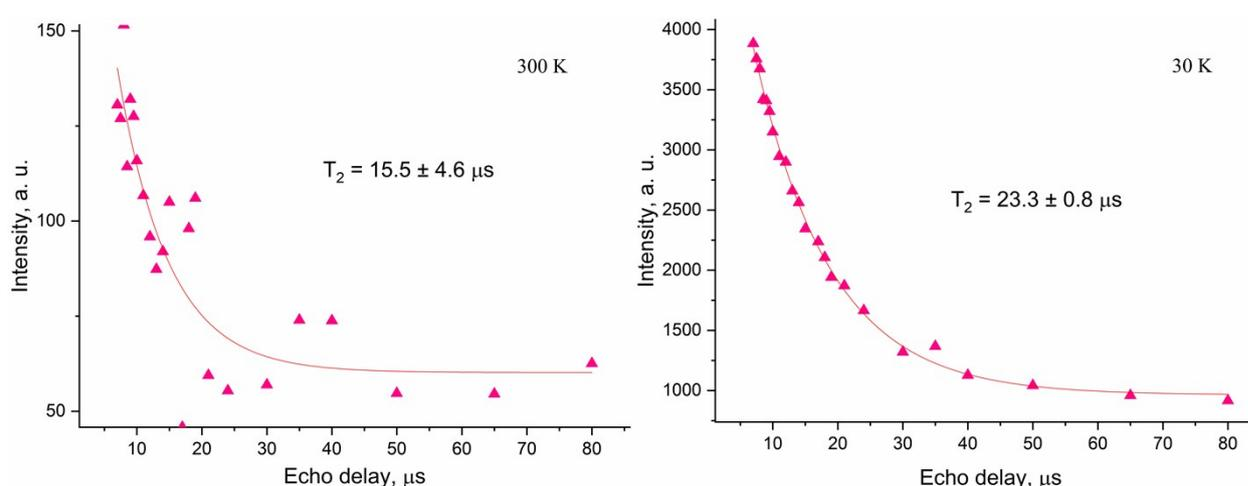
Figure S1. T<sub>2</sub> relaxation constant measurement results for 300 K (left) and 30 K (right) experiments. Experimental points are shown with symbols; the exponential decay approximation results are shown with solid red lines.
