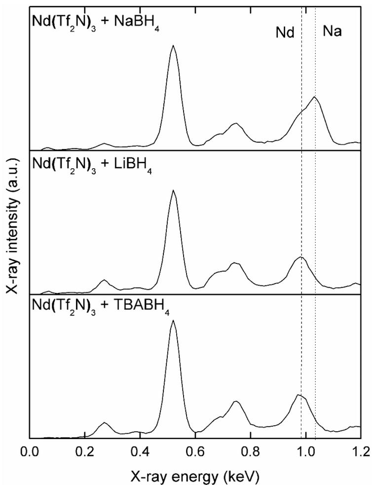
**Figure S9.** EDX spectra in the energy range 0–1.2 keV of neodymium deposits prepared in  $0.1 \text{ mol L}^{-1} \text{ Nd}(\text{Tf}_2\text{N})_3 + 4$  molar equivalents of  $\text{NaBH}_4$ ,  $\text{LiBH}_4$ , or  $\text{TBABH}_4$ , recorded at an acceleration voltage of 20 kV. The dashed and dotted lined indicate the characteristic X-ray lines of neodymium ( $\text{M}\alpha = 0.98 \text{ keV}$ ) and sodium ( $\text{K}\alpha = 1.04 \text{ keV}$ ), respectively.
