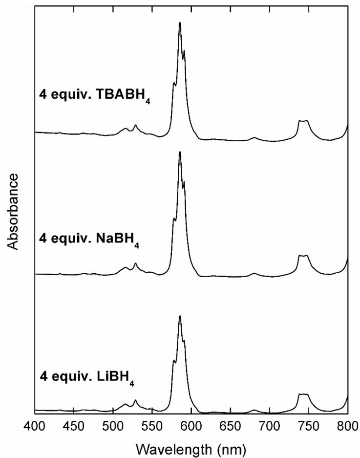
**Figure S1.** UV-Vis absorption spectra of  $0.1 \text{ mol L}^{-1} \text{ Nd}(\text{Tf}_2\text{N})_3$ , and 4 molar equivalents of TBABH<sub>4</sub> (top), NaBH<sub>4</sub> (middle), and LiBH<sub>4</sub> (bottom) in DME..
