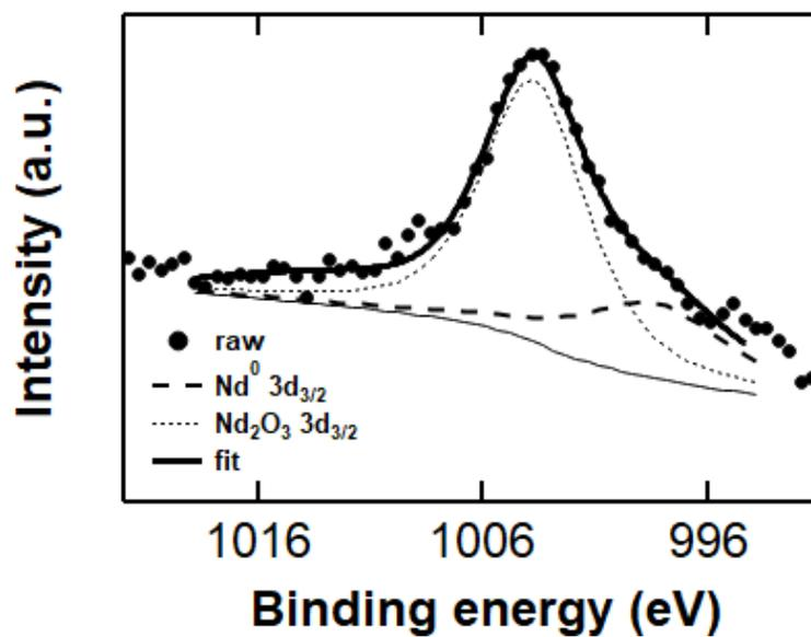
**Figure S11.** Curve-fitted Nd 3d<sub>3/2</sub> XPS spectra (surface) from deposits with a thickness of approx. 1 μm, obtained from potentiostatic deposition in Nd(Tf<sub>2</sub>N)<sub>3</sub> + TBABH<sub>4</sub> electrolytes at -3.4 V vs. Fc<sup>+</sup>/Fc.
