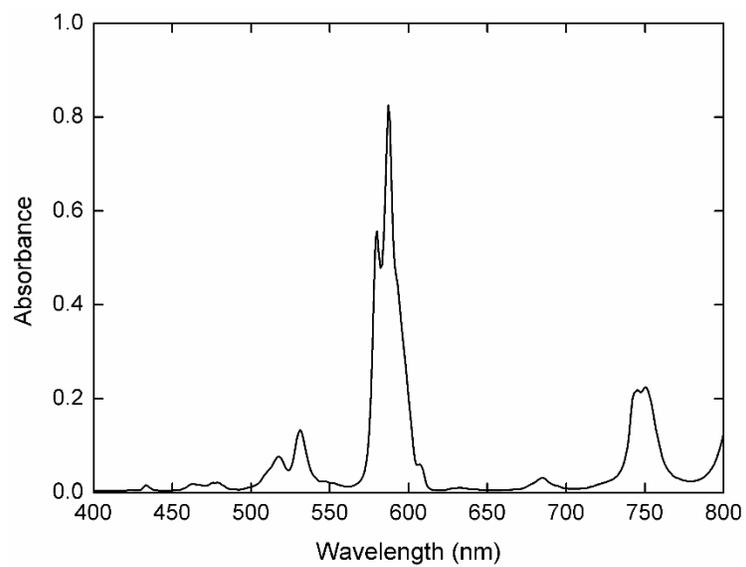
**Figure S3.** UV-Vis absorption spectrum of  $0.1 \text{ mol L}^{-1} \text{ Nd}_2\text{Cl}_6(\text{DME})_4$ , and 4 molar equivalents of  $\text{LiBH}_4$  in MeTHF.
