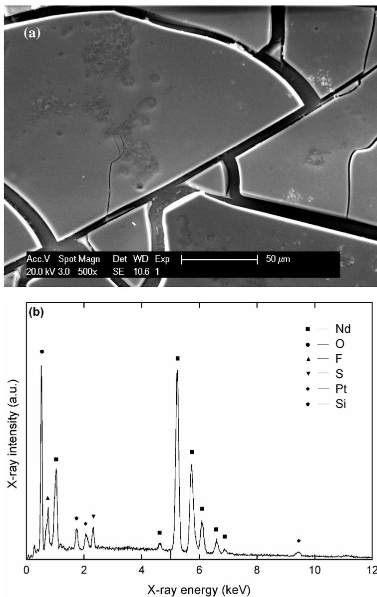
**Figure S7.** (a) Scanning electron micrograph of a deposit prepared at a constant potential of  $-3.1$  V vs.  $\text{Fc}^+/\text{Fc}$  in a stirred solution of  $0.1 \text{ mol L}^{-1}$   $\text{Nd}(\text{Tf}_2\text{N})_3$  + 4 molar equivalents of  $\text{NaBH}_4$  in DME at X500 magnification. (c) EDX spectrum of the deposit in the energy range 0–12 keV, recorded at an acceleration voltage of 20 kV with assignment of the major lines.
