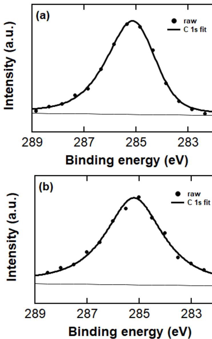
**Figure S10.** Curve-fitted C 1s XPS spectra (surface) from Nd (a) and Dy (b) deposits with a thickness of approx. 1  $\mu\text{m}$ , obtained from potentiostatic deposition in  $\text{Nd}(\text{Tf}_2\text{N})_3$  or  $\text{Dy}(\text{Tf}_2\text{N})_3 + \text{TBABH}_4$  electrolytes at  $-3.4 \text{ V vs. Fc}^+/\text{Fc}$ . The C 1s peak was shifted to 285.2 eV (mainly C–H bonds) for calibration of the spectra.
