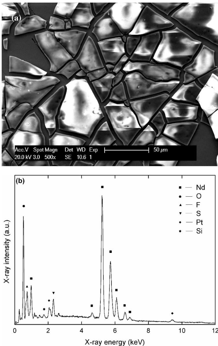
**Figure S8.** (a) Scanning electron micrograph of a deposit prepared at a constant potential of  $-3.1$  V vs.  $\text{Fc}^+/\text{Fc}$  in a stirred solution of  $0.1 \text{ mol L}^{-1} \text{ Nd}(\text{Tf}_2\text{N})_3 + 4$  molar equivalents of  $\text{LiBH}_4$  in DME at X500 magnification. (c) EDX spectrum of the deposit in the energy range 0–12 keV, recorded at an acceleration voltage of 20 kV with assignment of the major lines.
