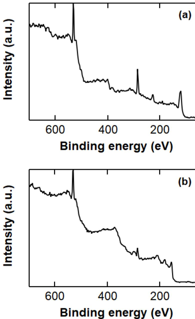
**Figure S12.** XPS survey scans in the range 60–700 eV, of Nd (a) and Dy (b) deposits with a thickness of approx. 1  $\mu\text{m}$ , obtained from potentiostatic deposition in  $\text{Nd}(\text{Tf}_2\text{N})_3$  or  $\text{Dy}(\text{Tf}_2\text{N})_3$  +  $\text{TBABH}_4$  electrolytes at  $-3.4$  V vs.  $\text{Fc}^+/\text{Fc}$ .
