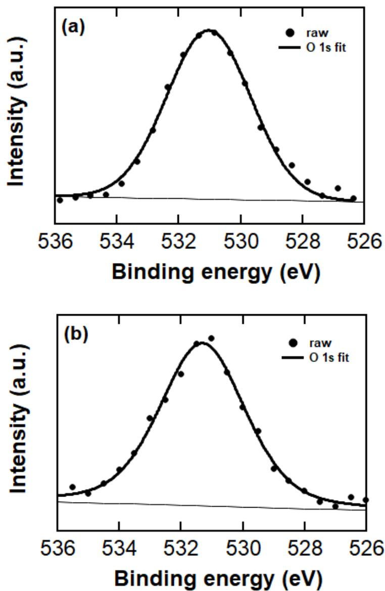
**Figure S13.** Curve-fitted O 1s XPS spectra (surface) from Nd (a) and Dy (b) deposits with a thickness of approx. 1  $\mu\text{m}$ , obtained from potentiostatic deposition in  $\text{Nd}(\text{Tf}_2\text{N})_3$  or  $\text{Dy}(\text{Tf}_2\text{N})_3 + \text{TBABH}_4$  electrolytes at  $-3.4 \text{ V vs. Fc}^+/\text{Fc}$ .
