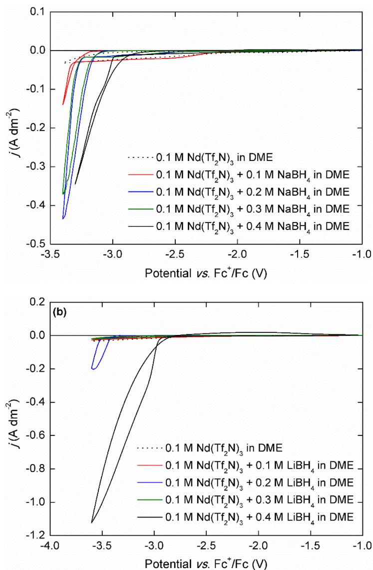
**Figure S5.** CVs (first cycle) of 0.1 mol L<sup>-1</sup> Nd(Tf<sub>2</sub>N)<sub>3</sub> + 0 to 4 molar equivalents of (a) NaBH<sub>4</sub>, and (b) LiBH<sub>4</sub>, recorded at a scan rate of 10 mV s<sup>-1</sup>. The working and counter electrodes were pieces of platinum-coated silicon wafers with a surface area of 0.003 dm<sup>2</sup> and 0.01 dm<sup>2</sup>, respectively. The reference electrode was Fc<sup>+</sup>/Fc (0.005 mol L<sup>-1</sup> each) dissolved in [BMP][Tf<sub>2</sub>N].
