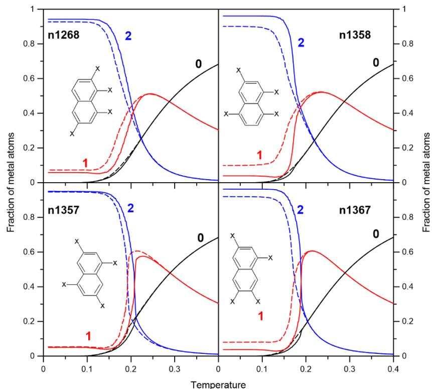
**Figure S14.** Effect of temperature on the fraction of metal atoms connected to zero, one and two naphthalene linkers, calculated for the enantiopure (*R*, solid lines) and racemic (*R+S*, dashed lines) overlays comprising the isomers **n1268**, **n1357**, **n1358** and **n1367** ( $N_l = 400$ ,  $N_m = 800$ ,  $L = 200$ ).
