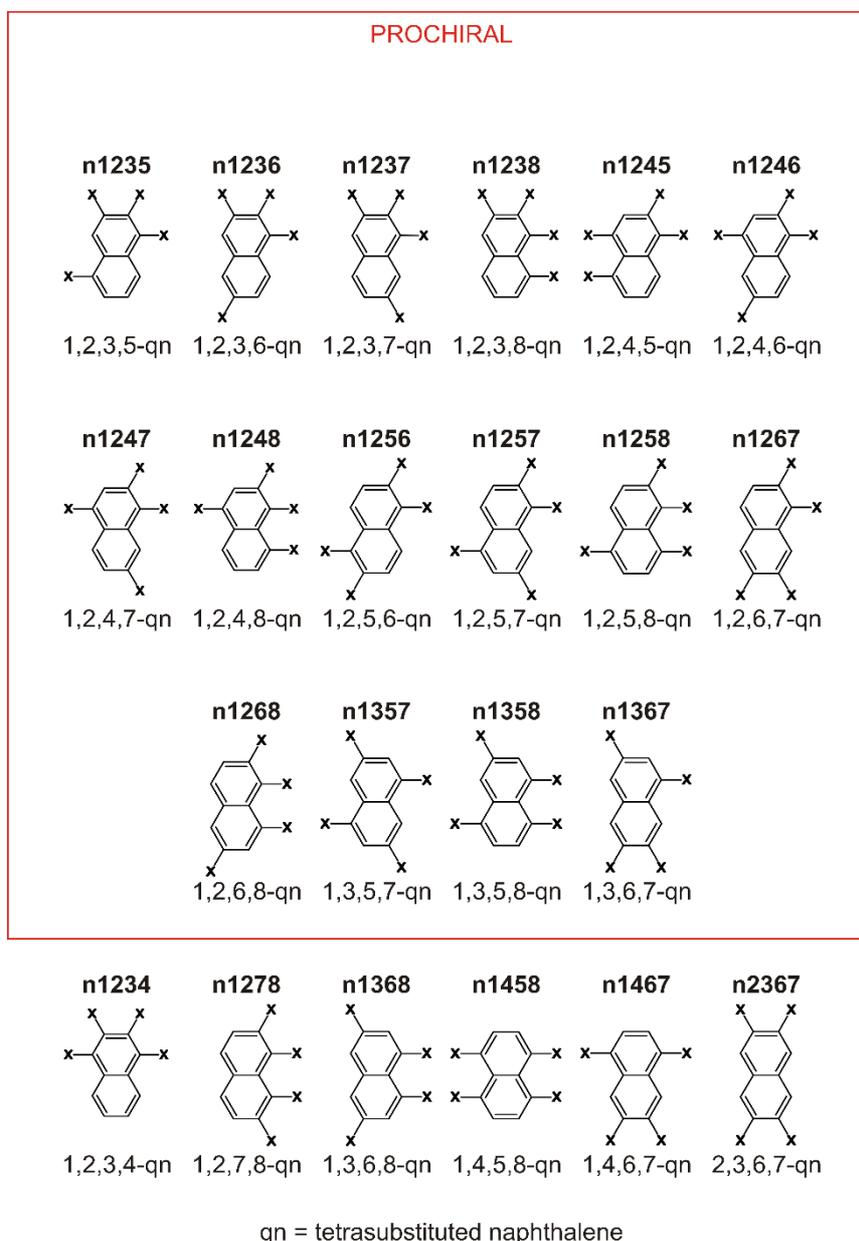
**Figure S1.** Schematic structures of the 22 possible tetrasubstituted isomers of naphthalene. The sixteen prochiral molecules, able to adopt mirror-image configurations when adsorbed, are grouped inside the red frame. The remaining six achiral molecules are shown below the frame.
