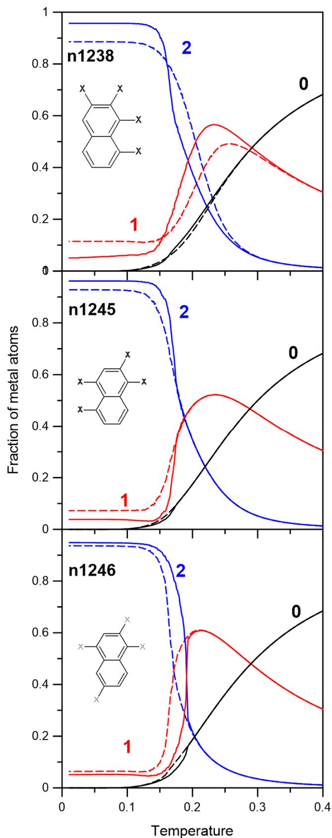
**Figure S8.** Effect of temperature on the fraction of metal atoms connected to zero, one and two naphthalene linkers, calculated for the enantiopure (*R*, solid lines) and racemic (*R+S*, dashed lines) overlayers comprising the isomers **n1238**, **n1245** and **n1246** ( $N_l = 400$ ,  $N_m = 800$ ,  $L = 200$ ).
