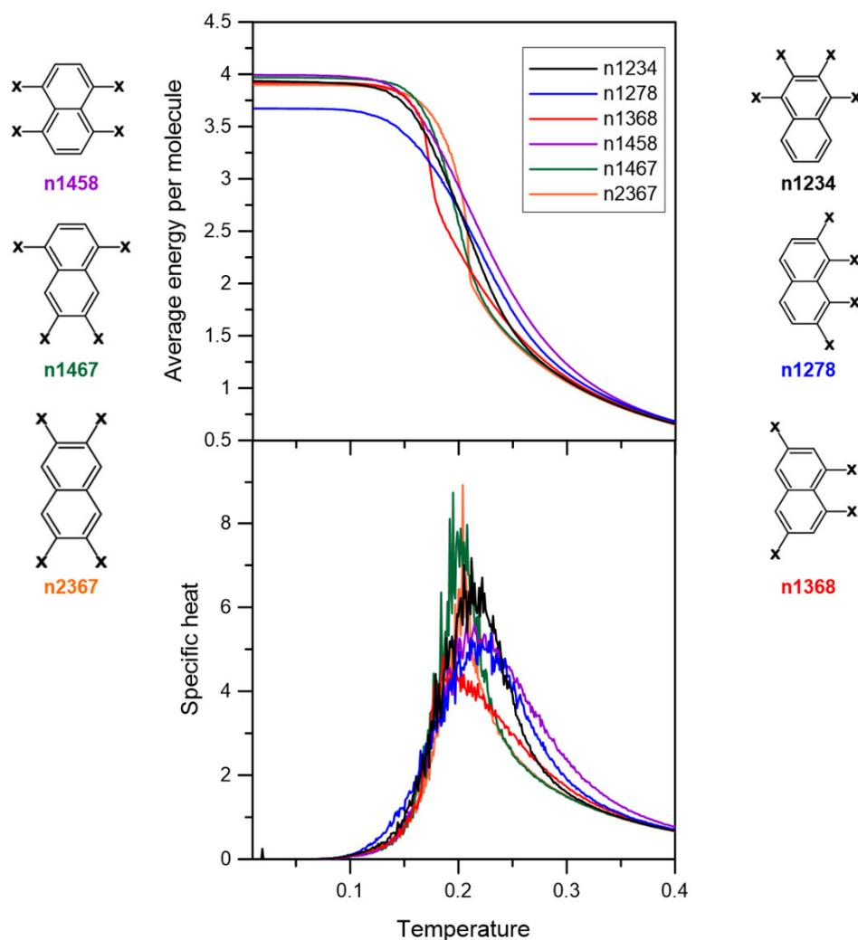
**Figure S3.** Effect of temperature on the average interaction energy per molecule (top) and specific heat capacity (bottom) calculated for the achiral isomers of **n** shown in the figure. The calculated temperature dependencies are averages over ten independent system replicas, each comprising 800 metal atoms and 400 molecules **n** ( $L = 200$ ).
