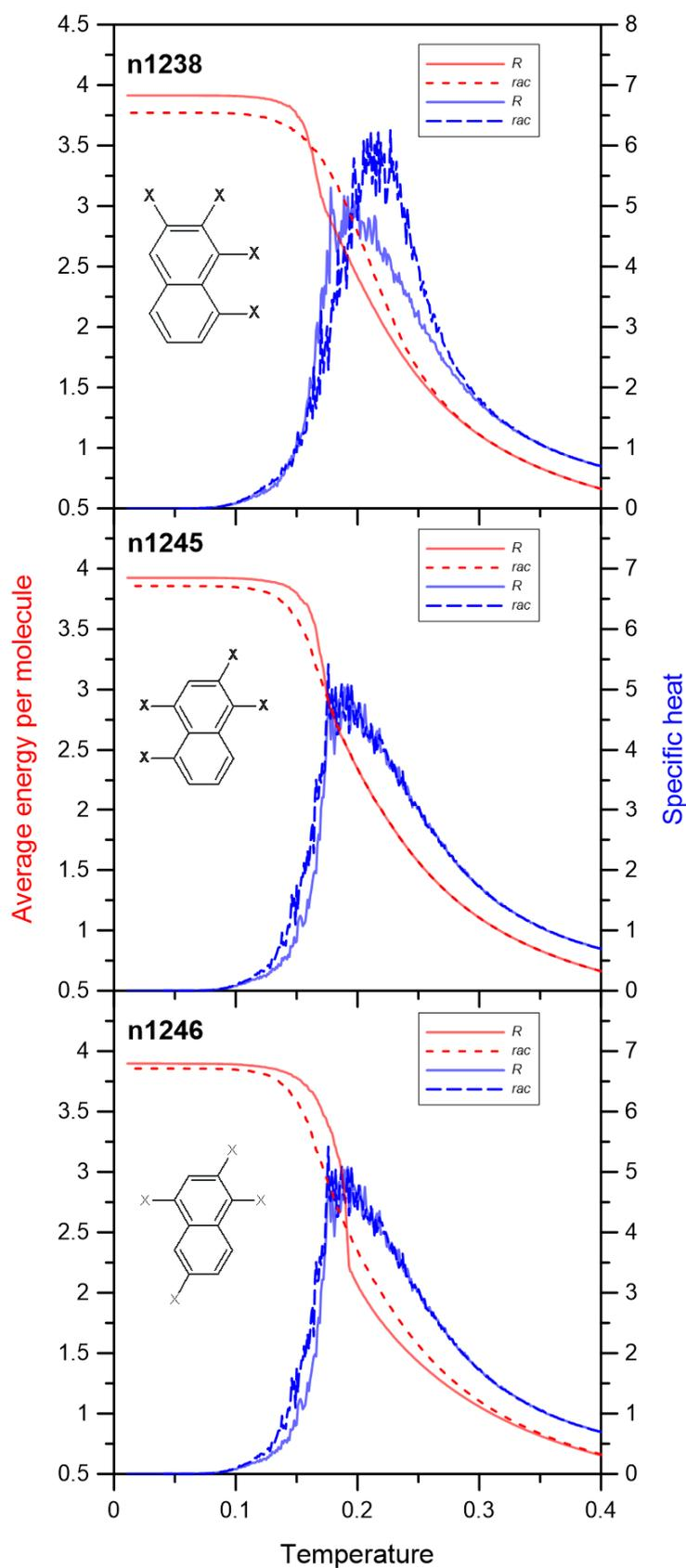
**Figure S7.** Effect of temperature on the mean molecular energy and specific heat capacity calculated for the enantiopure (*R*) and racemic (*R+S*) overlays comprising the isomers **n1238**, **n1245** and **n1246** ( $N_l = 400$ ,  $N_m = 800$ ,  $L = 200$ ).
