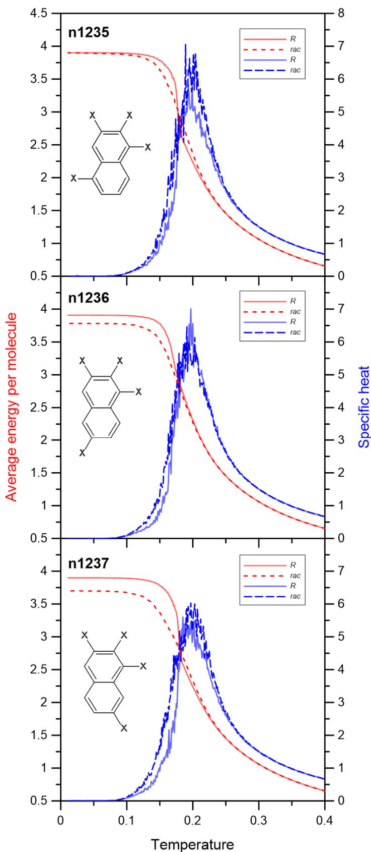
**Figure S5.** Effect of temperature on the mean molecular energy and specific heat capacity calculated for the enantiopure (*R*) and racemic (*R*+*S*) overlayers comprising the isomers **n1235**, **n1236** and **n1237** ( $N_l = 400$ ,  $N_m = 800$ ,  $L = 200$ ).
