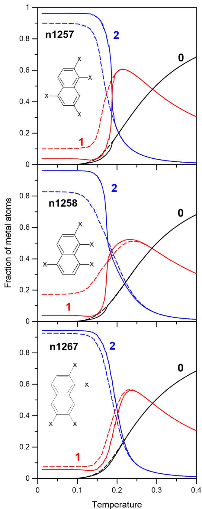
**Figure S12.** Effect of temperature on the fraction of metal atoms connected to zero, one and two naphthalene linkers, calculated for the enantiopure (*R*, solid lines) and racemic (*R+S*, dashed lines) overlayers comprising the isomers **n1257**, **n1258** and **n1267** ( $N_l = 400$ ,  $N_m = 800$ ,  $L = 200$ ).
