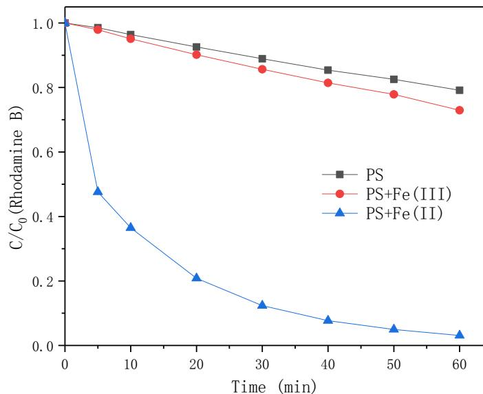
38 **Fig.S1 Variation of RhB concentration ( $C/C_0$ ) with reaction time in different
