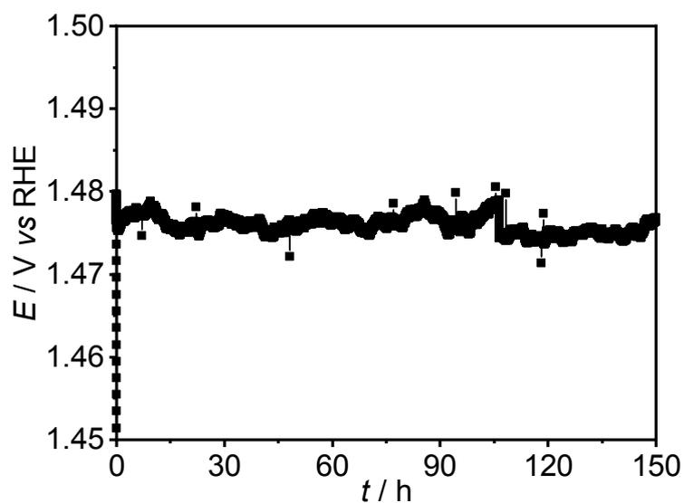
**Figure S6** Controlled-current ( $10 \text{ mA cm}^{-2}$ ) OER over **AlCoP** foam electrocatalyst conducted in 1.0 M KOH.
