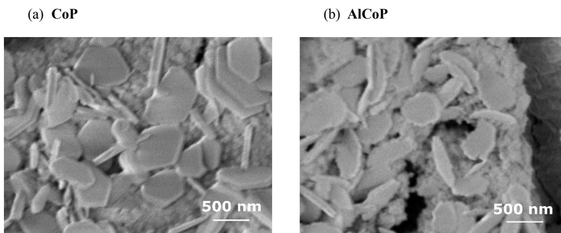
**Figure S7** SEM of (a) **CoP** and (b) **AlCoP** after electrochemical OER testing in 1 M KOH (up to 1.45 V vs. RHE for 10 mins).
