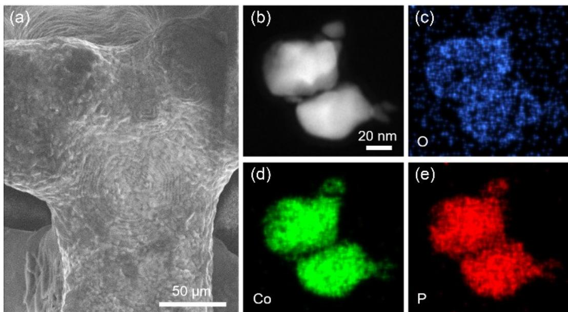
**Figure S2** (a) SEM image of as-synthesised **CoP** foam anode. (b) HAADF-STEM image of representative particles. STEM-EDX elemental maps of (c) O, (d) Co and (e) P.
