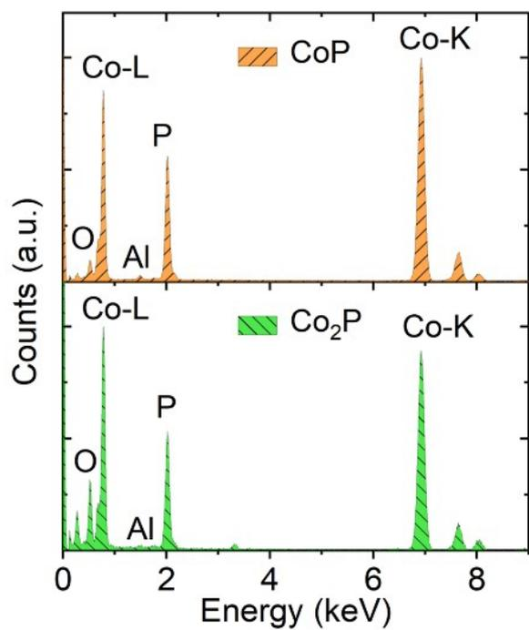
**Figure S3** Representative EDX spectra collected from **AlCoP**, confirming the expected **CoP** and **Co<sub>2</sub>P** phase composition.
