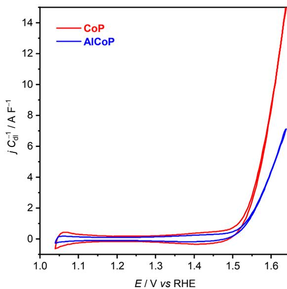
**Figure S5** Cyclic voltammetry data presented in Figure 2a, with currents normalised to double layer capacitance calculated in Figure 2c.
