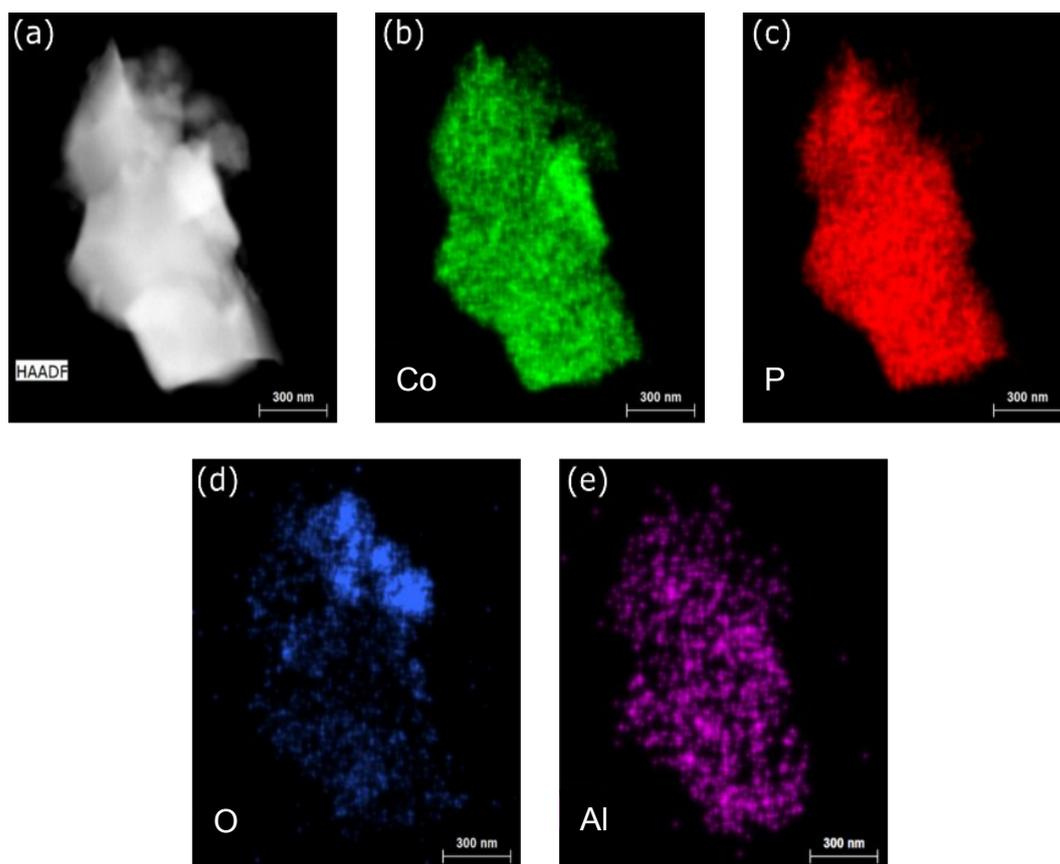
**Figure S8** (a) HAADF-STEM image of representative AlCoP particle after 150 h stability testing and STEM-EDX elemental maps of (b) Co, (c) P, (d) O and (e) Al.
