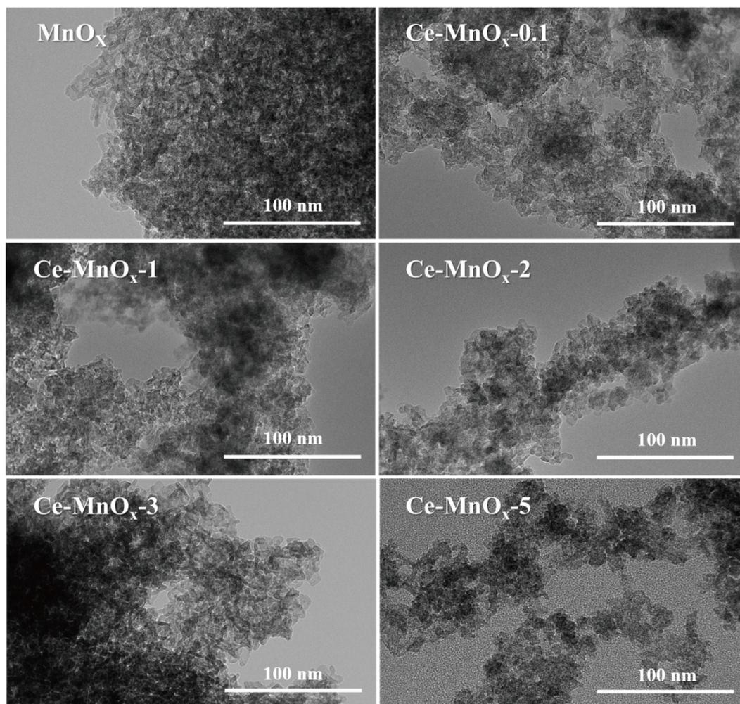
**Fig. S5** TEM images of the undoped  $\text{MnO}_x$  and  $\text{Ce-MnO}_x$ .
