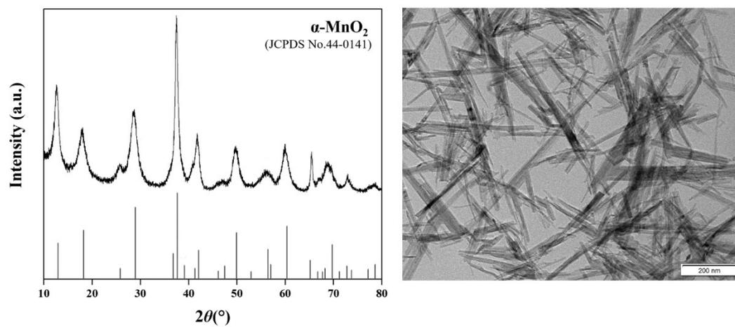
**Fig. S1** The XRD pattern and TEM image of  $\alpha\text{-MnO}_2$  nanorods synthesized by hydrothermal method.
