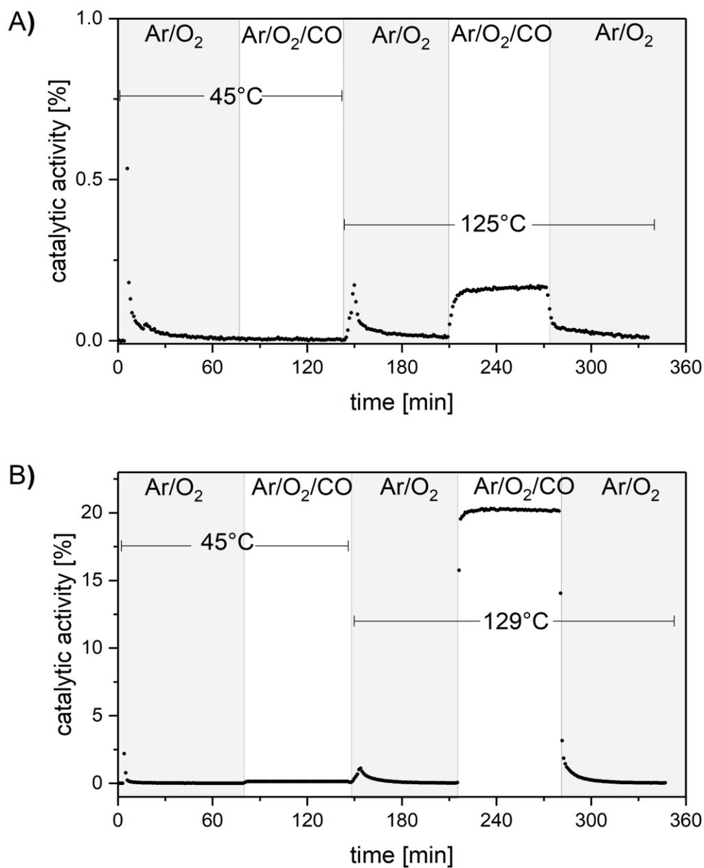
**Figure S5:** Catalytic activity during CO oxidation over **A)** CeO<sub>2</sub> nanocubes at 45 °C and 125 °C, and **B)** 0.3 wt% Au/CeO<sub>2</sub> nanocubes at 45 °C and 129 °C. The samples were exposed to a CO/O<sub>2</sub>/Ar stream (2% CO, 25% O<sub>2</sub>, Ar; 100 mL/min) under reaction conditions and to an O<sub>2</sub>/Ar stream (25% O<sub>2</sub>, Ar; 100 mL/min) prior to and after reaction conditions, respectively.
