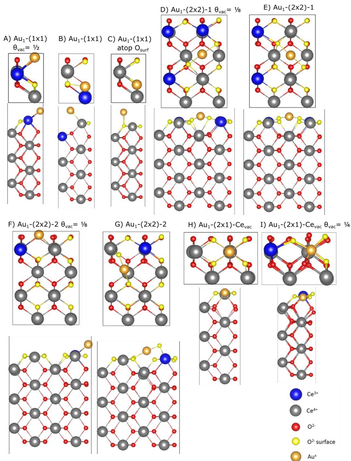
**Figure S10:** CeO<sub>2</sub>(110) unit cells with top and side view of the most stable gold species on CeO<sub>2</sub>(110) and CeO<sub>2-x</sub>(110), respectively ((A) to G)). H) and I) show structures in which one cerium atom is substituted by a gold atom. The corresponding periodicities are indicated. Atoms correspond to Ce<sup>3+</sup> (blue), Ce<sup>4+</sup> (grey), O<sup>2-</sup> (red), surface O<sup>2-</sup> (yellow) and Au<sup>x</sup> (gold).
