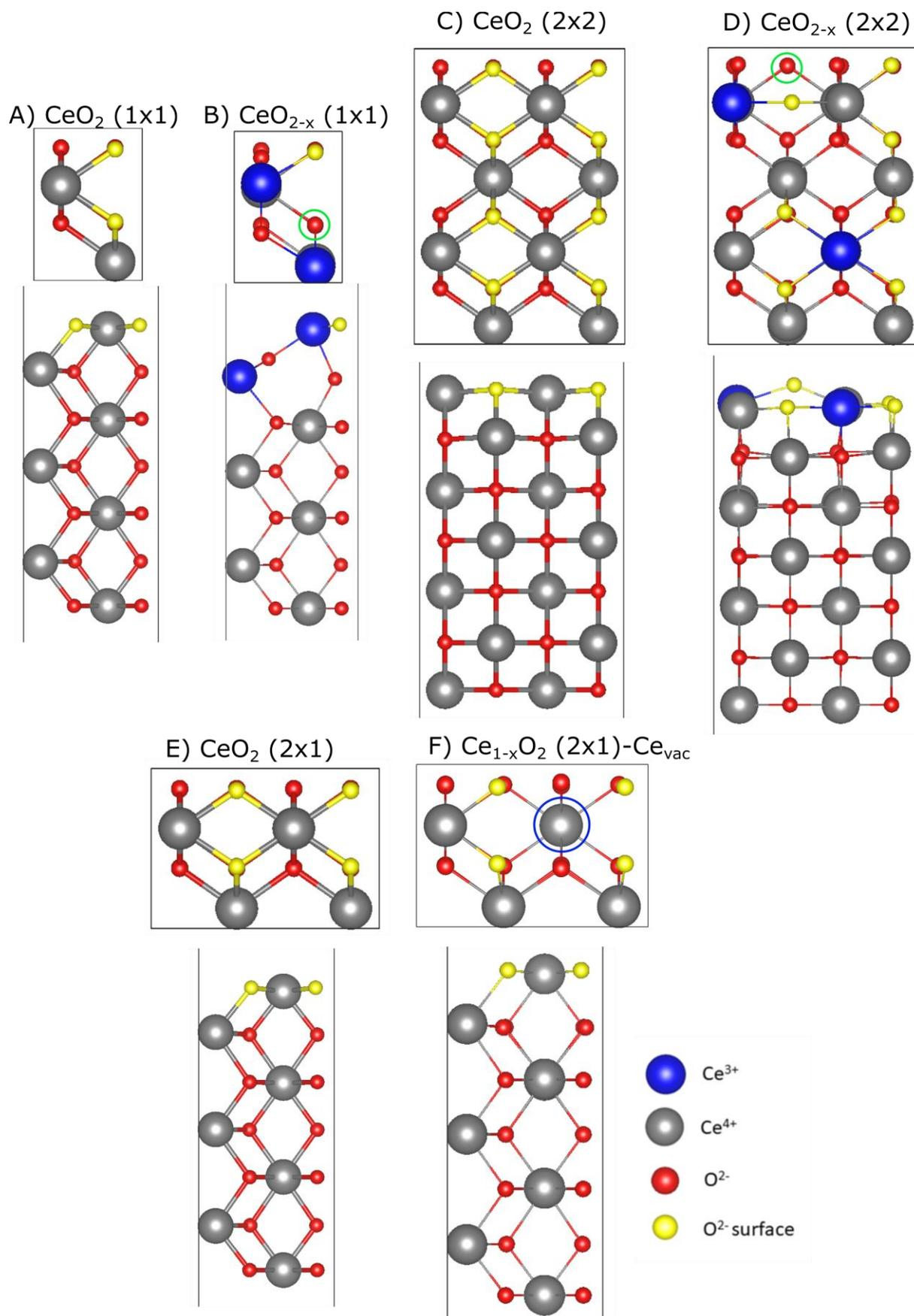
**Figure S9:**  $\text{CeO}_2(110)$  unit cells with top and side view of the bare  $\text{CeO}_2(110)$  and defective  $\text{CeO}_{2-x}(110)$  as well as  $\text{Ce}_{1-x}\text{O}_2(110)$  with  $(1 \times 1)$ ,  $(2 \times 1)$  and  $(2 \times 2)$  periodicity, respectively. Atoms correspond to  $\text{Ce}^{3+}$
