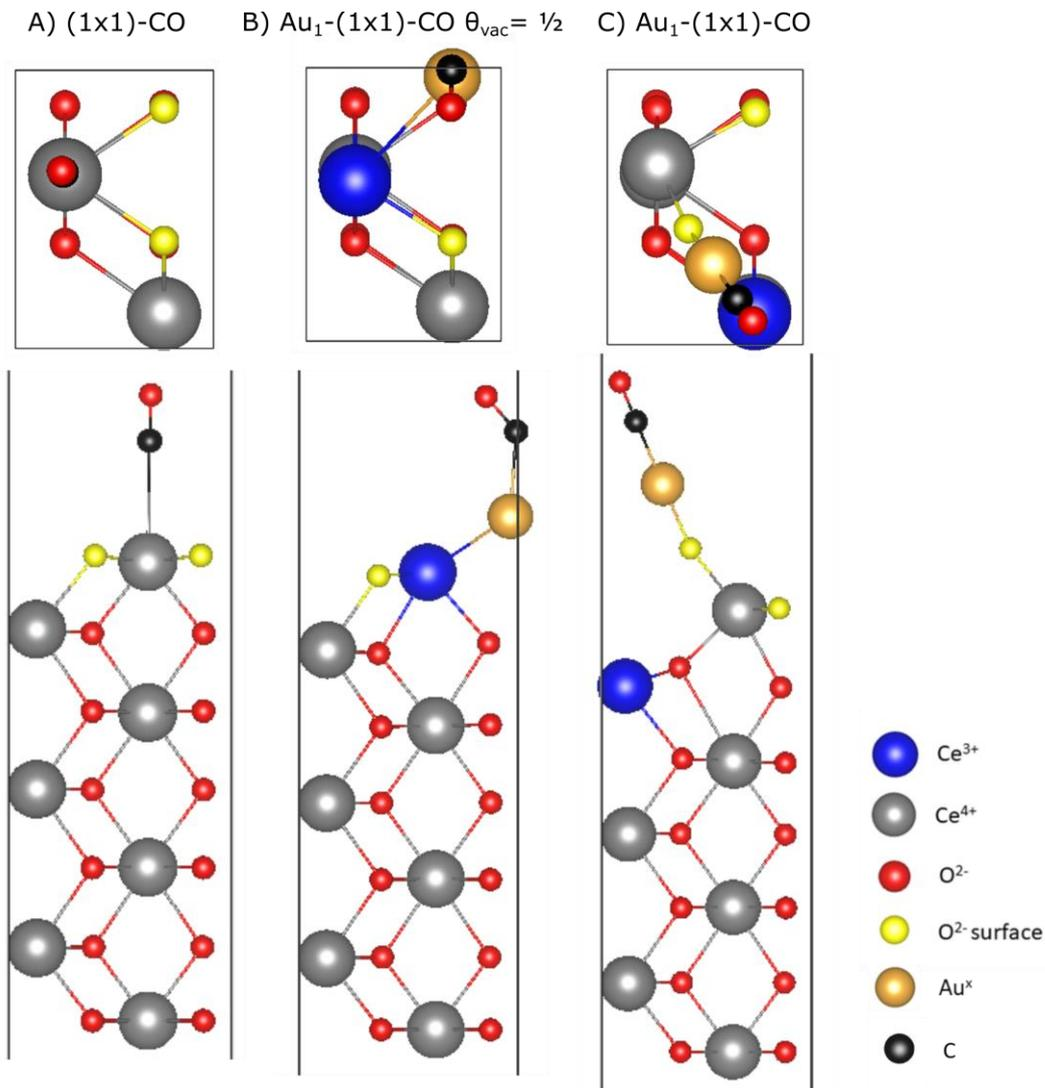
**Figure S12:** CO-Au<sub>1</sub>/CeO<sub>2</sub>(110) and CO-Au<sub>1</sub>/CeO<sub>2-x</sub>(110) unit cells with top and side view with (1×1) periodicity. Atoms correspond to Ce<sup>3+</sup> (blue), Ce<sup>4+</sup> (grey), O<sup>2-</sup> (red), surface O<sup>2-</sup> (yellow) Au<sup>x</sup> (gold) and C (black).
