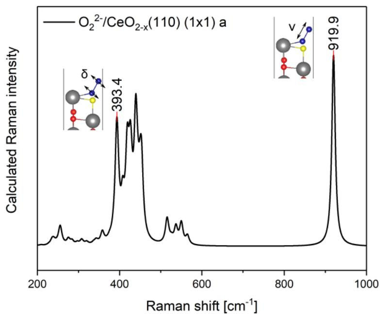
**Figure S7:** Calculated Raman spectrum for  $\text{O}_2/\text{CeO}_{2-x}(110)$  with  $(1 \times 1)$  periodicity. The band positions of the peroxide vibrations are indicated together with the corresponding symmetry.
