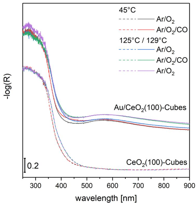
**Figure S6:** *Operando* UV-Vis spectra of the bare ceria cubes (at the bottom, dashed lines) and the gold-loaded cubes (at the top, solid lines). The spectra were recorded at the temperatures indicated, at a total flow rate of 100 mL/min, and feed compositions of 2% CO / 25% O<sub>2</sub> / Ar and 25% O<sub>2</sub> / Ar for reactive and oxidative conditions, respectively. Spectra of the gold-loaded samples were offset for clarity.
