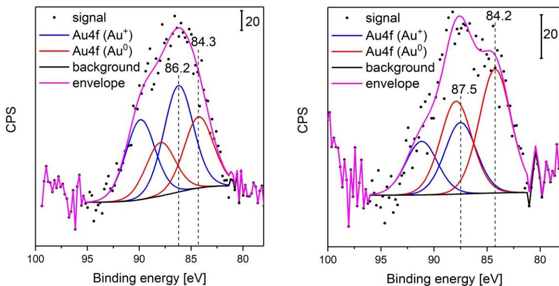
**Figure S4:** Au4f photoemission of the gold loaded cubes (left) and rods (right). Data is represented by black dots, and the background by a black line and the envelope of all contributions in shown in magenta. Blue curves correspond to the signal of cationic gold and red curves to the signal of metallic gold. The positions of the Au4f<sub>7/2</sub> signals are indicated.
