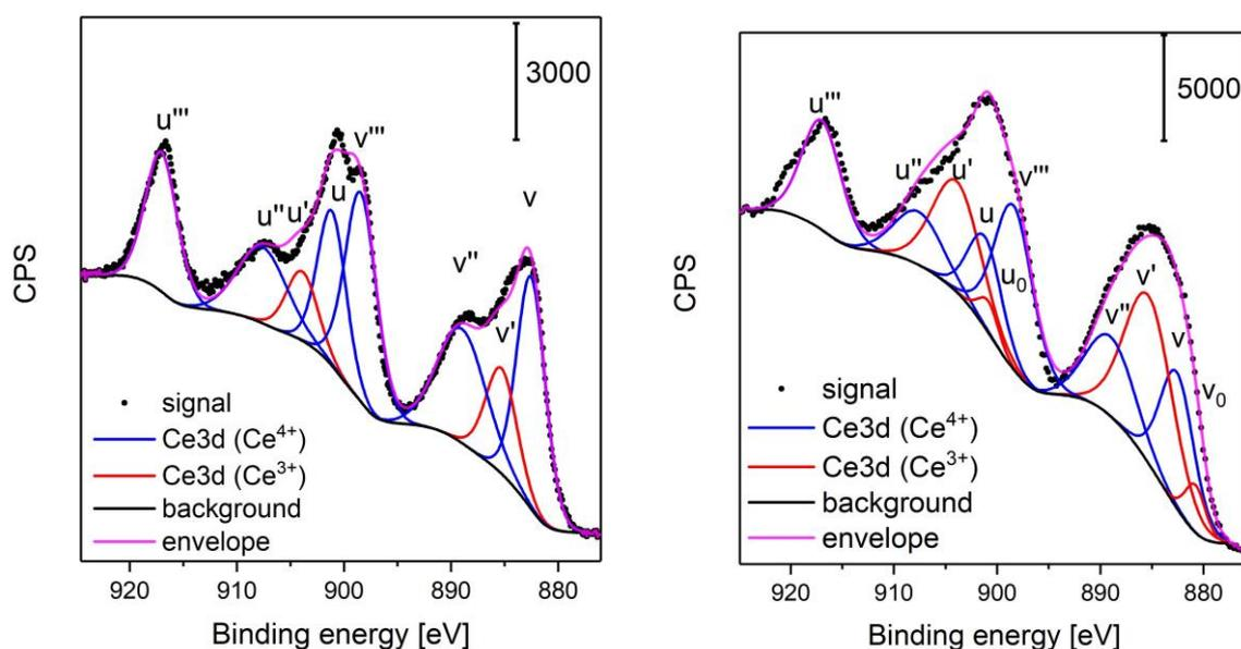
**Figure S3:** Ce3d photoemission of the bare ceria rods (left) and of the gold loaded rods (right). Data is represented by black dots, and the background by a black line. A fitting analysis yields  $\text{Ce}^{3+}$  (red) and  $\text{Ce}^{4+}$  (blue) contributions as indicated. The envelope of all contributions in shown in magenta.
