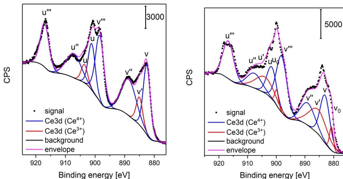
**Figure S2:** Ce3d photoemission of the bare ceria cubes (left) and the gold loaded cubes (right). Data is represented by black dots, and the background by a black line. A fitting analysis yields  $\text{Ce}^{3+}$  (red) and  $\text{Ce}^{4+}$  (blue) contributions as indicated. The envelope of all contributions in shown in magenta.
