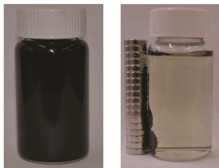
Figure S1: Iron oxide magnetic nanoparticles (MNPs) before and after applying an external magnetic field.
