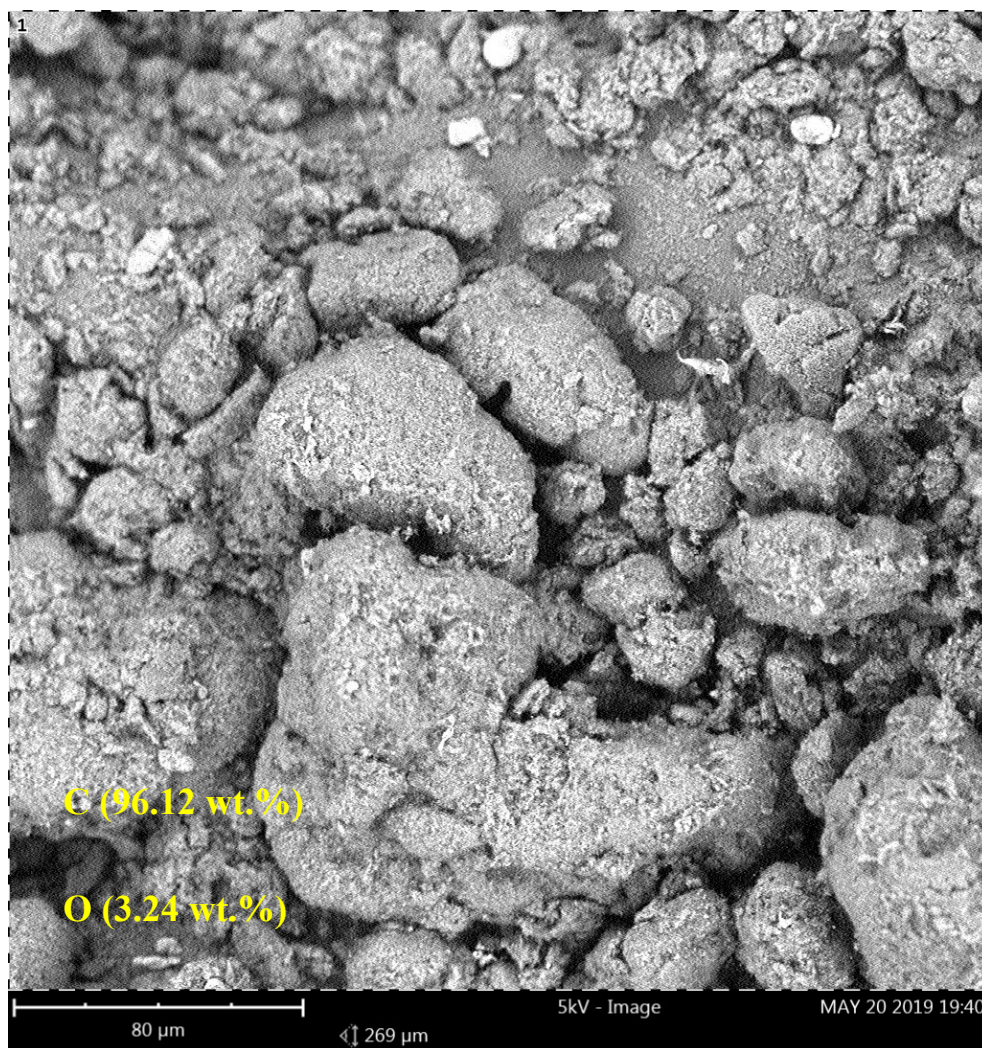
Fig. S22 SEM image of CALB/MWCNT-PTFE(1.00 wt.%) support with results of EDS analysis.
