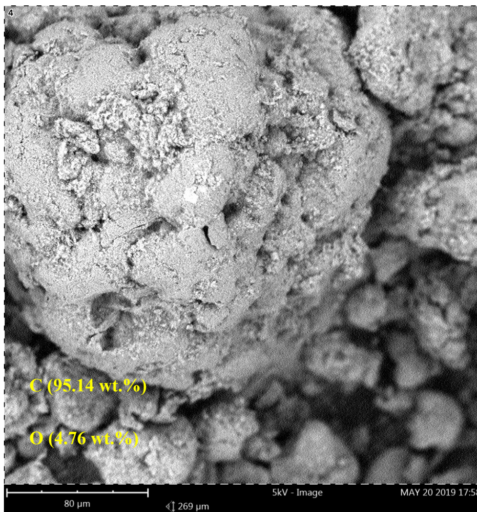
Fig. S20 SEM image of CALB/MWCNT-PTFE(0.01 wt.%) support with results of EDS analysis.
