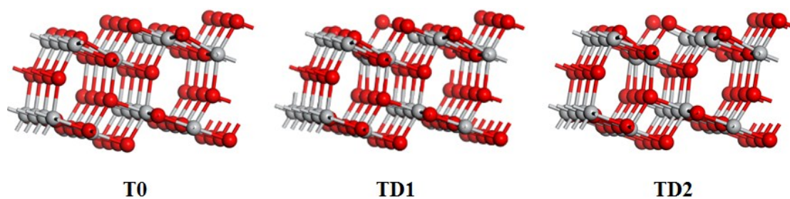
Fig. S4 Three different configurations: pure anatase \text{TiO}_2 (101) surface (T0), defective \text{TiO}_2 with one oxygen vacancy (TD1) and defective \text{TiO}_2 with two oxygen vacancies (TD2). The light gray and red balls represent Ti and O atoms, respectively.
