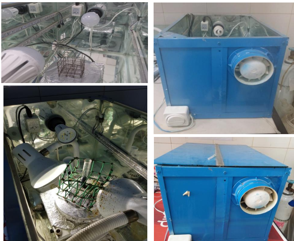
Figure S1. The box containing 14 W blue LED lamp ( \lambda > 410 nm) and the reaction setup up.
