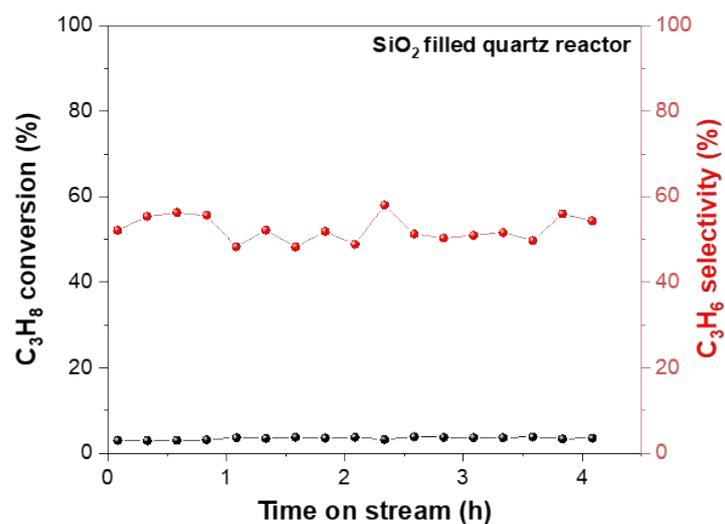
Figure S3. Propane dehydrogenation over blank quartz reactor filled with SiO<sub>2</sub> support at 600°C, atmospheric pressure and 50 mL/min of 20 vol.% C<sub>3</sub>H<sub>8</sub>/He flow. The conversion of propane was stable at 3% while selectivity to propylene was close to 53%. This activity can be rationalized by thermal dehydrogenation of propane.
