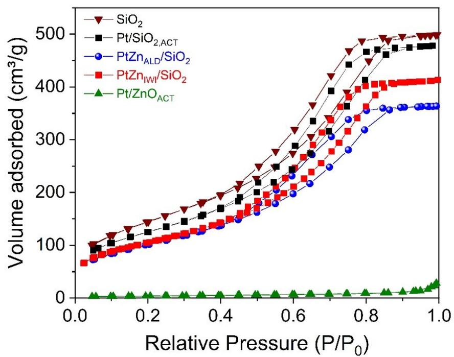
Figure S1. N<sub>2</sub> sorption isotherm of activated catalysts.
