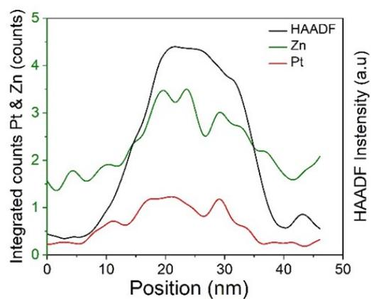
Figure S8. EDX mapping and line scan analysis on  $\text{Pt}_1\text{Zn}_1$  nanoalloy particles in  $\text{PtZn}_{\text{ALD}}/\text{SiO}_2$ , sitting at edge and in middle of support where the effect of Zn from ZnO under-layer can be seen.
