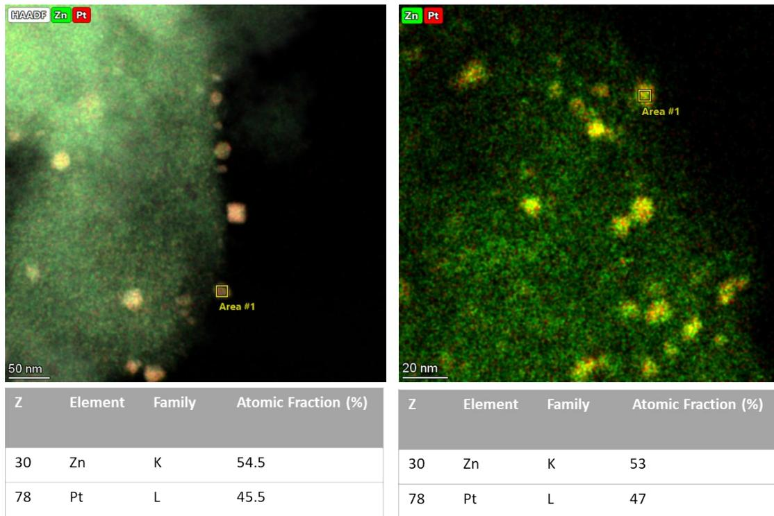
Figure S7. STEM EDX and elemental mapping of PtZn<sub>ALD</sub>/SiO<sub>2</sub> after reaction, indicating the atomic fraction of Pt and Zn, in agreement with the formation of Pt<sub>1</sub>Zn<sub>1</sub> alloy.
