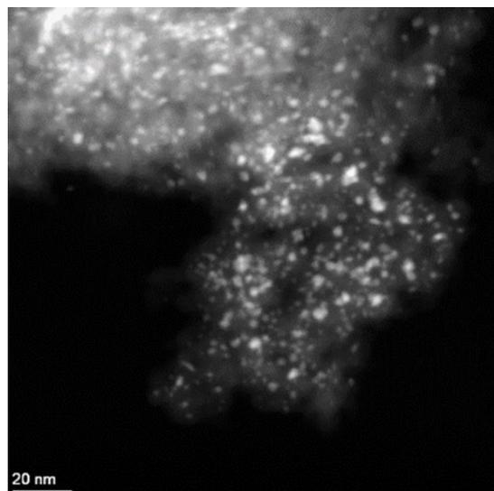
Figure S6. HAADF-STEM image of the spent Pt/SiO<sub>2</sub> catalyst.
