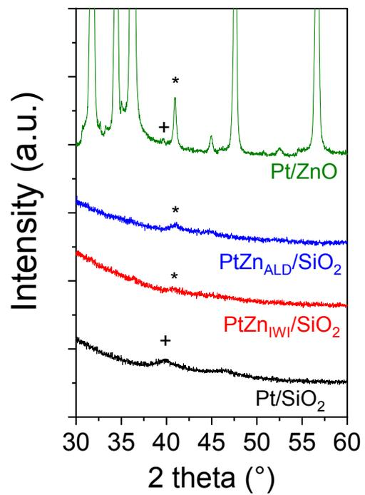
Figure S5. XRD analysis of spent catalyst. (+: Pt and \* Pt<sub>1</sub>Zn<sub>1</sub>)
