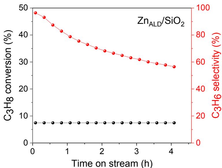
Figure S4. Propane dehydrogenation over Zn<sub>ALD</sub>/SiO<sub>2</sub>, (prepared via 1 cycle of ZnO ALD onto SiO<sub>2</sub>) measured at 600°C, atmospheric pressure and 50 mL/min of 20 vol.% C<sub>3</sub>H<sub>8</sub>/He flow.
