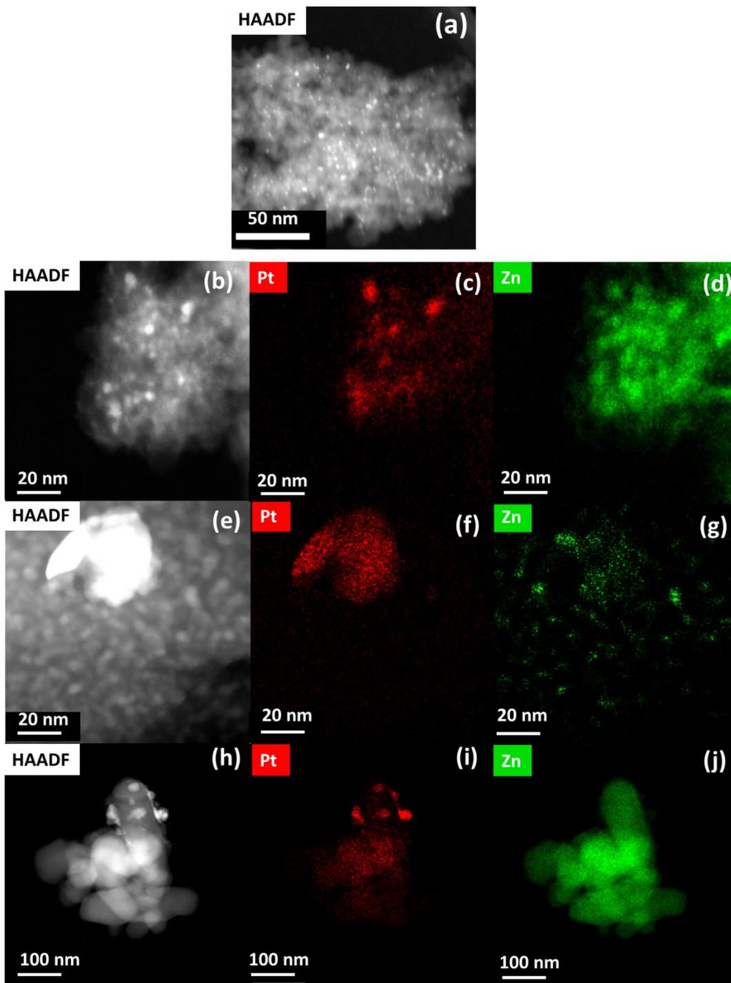
Figure S2. HAADF-STEM images and EDX maps of Pt and Zn in as synthesized (a) Pt/SiO<sub>2</sub>, (b-d) Pt/ZnO<sub>ALD</sub>/SiO<sub>2</sub>, (e-g) Pt/ZnO<sub>IWI</sub>/SiO<sub>2</sub> and (h-j) Pt/ZnO
