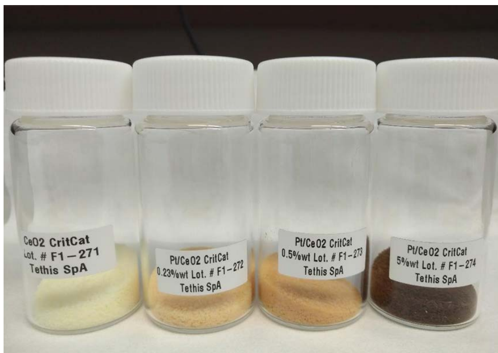
Fig. S1 Image showing color change as a function of Pt loading for the catalysts as-synthesized by FSP.
