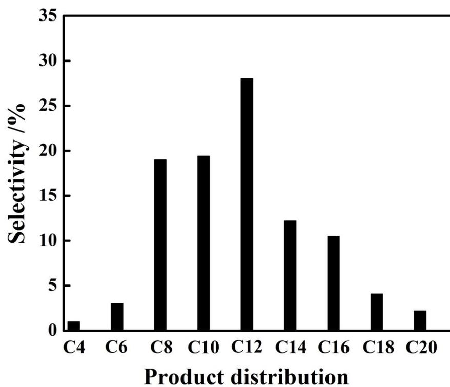
**Fig. S1** The detailed product distribution of ethylene oligomerization on the N<sub>2</sub>-Ni/ASA catalyst. Reaction conditions: 60 °C, 3.0 MPa, 0.5 g catalyst, 50% C<sub>2</sub>H<sub>4</sub> - 50% N<sub>2</sub> with a flowrate of 15 mL min<sup>-1</sup>.
