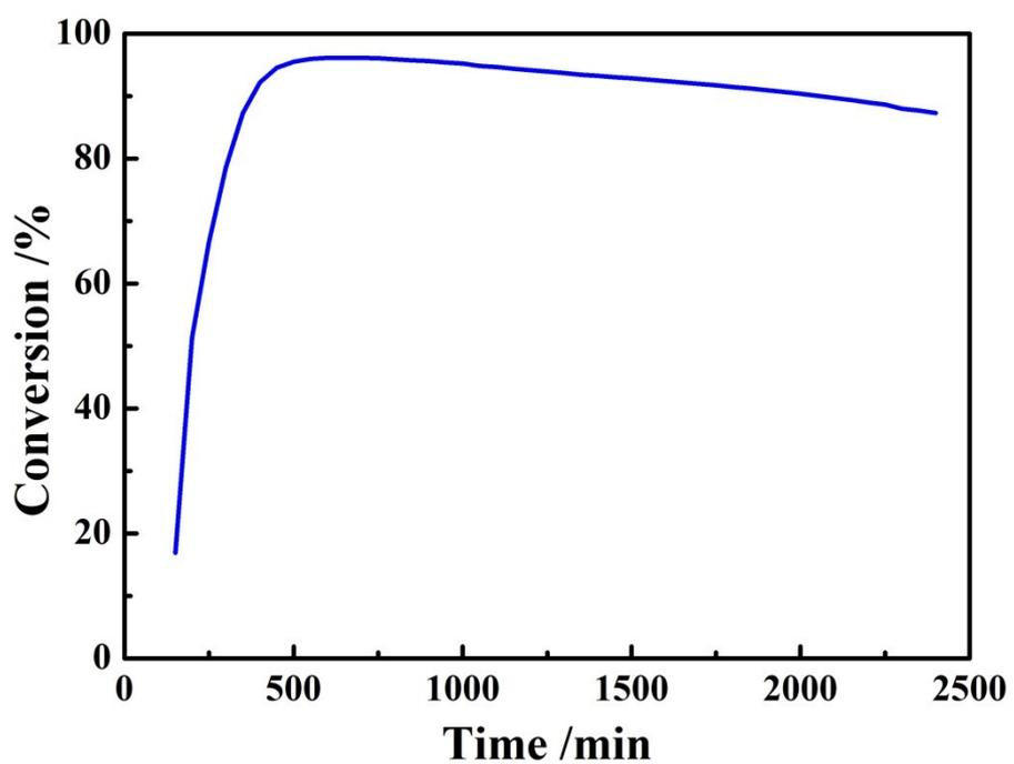
**Fig. S3** The stability testing of the N<sub>2</sub>-pretreated catalyst. Reaction condition: 0.5 g catalyst, reaction temperature is 60 °C, reaction pressure is 3 MPa, 50% C<sub>2</sub>H<sub>4</sub> - 50% N<sub>2</sub> with a flowrate of 15 mL min<sup>-1</sup>.
