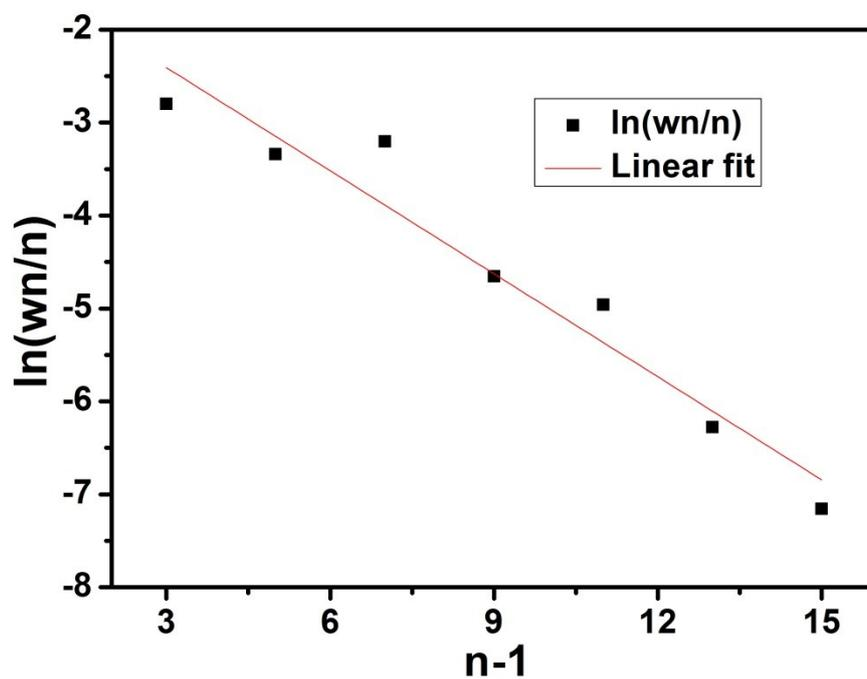
Fig. S5 The calculation of carbon chain growth probability. Reaction conditions: 60 °C, 3.0 MPa, 0.5 g catalyst, 50% C<sub>2</sub>H<sub>4</sub> - 50% N<sub>2</sub> with a flowrate of 15 mL min<sup>-1</sup>, MSHV = 2.25 h<sup>-1</sup>.
