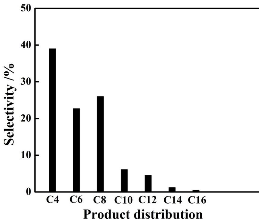
Fig. S4 The detailed product distribution of ethylene oligomerization on the  $N_2$ -Ni/ASA catalyst. Reaction conditions:  $60 \text{ }^\circ\text{C}$ ,  $3.0 \text{ MPa}$ ,  $0.5 \text{ g}$  catalyst,  $50\% \text{ C}_2\text{H}_4 - 50\% \text{ N}_2$  with a flowrate of  $15 \text{ mL min}^{-1}$ ,  $\text{MSHV} = 2.25 \text{ h}^{-1}$ .
