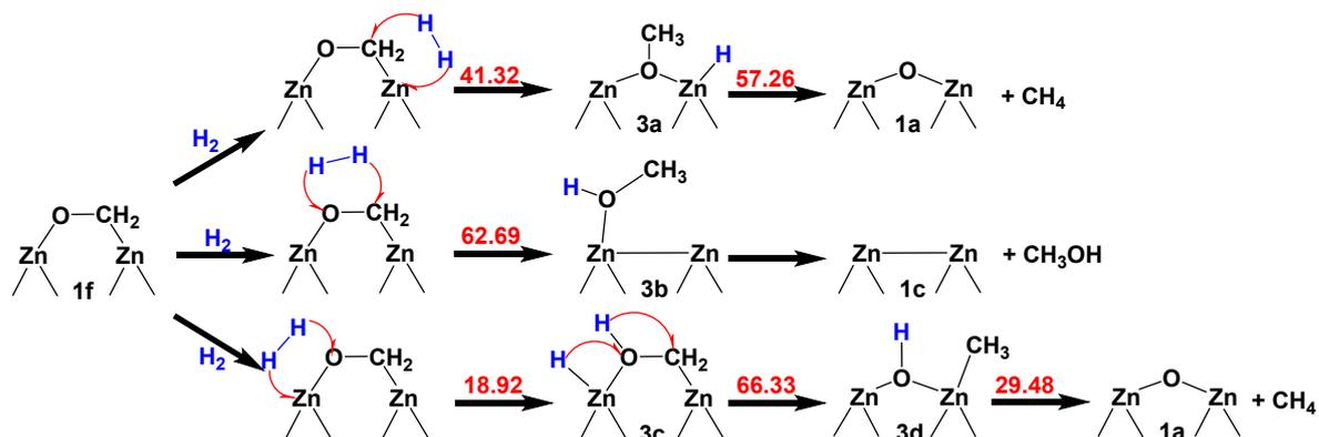
**Figure S2.** The reaction pathway and barriers of hydrogenation of 1f  $[\text{Zn-OCH}_2\text{-Zn}]^{2+}$ .
