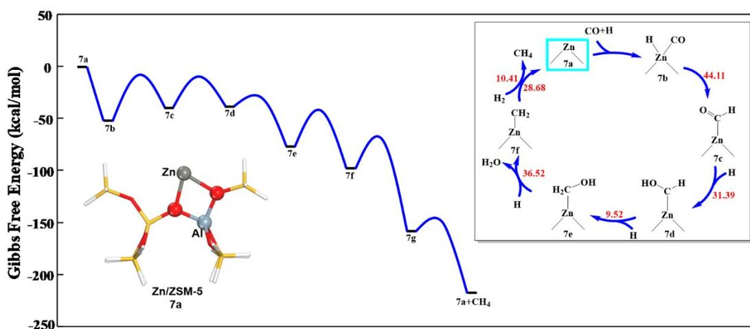
**Figure S6.** The single  $\text{Zn}^{2+}$  site graft on 8T ZSM-5 cluster model (Zn/ZSM-5), the Gibbs free energy and reaction cycle of CO hydrogenation to methane over Zn/ZSM-5. Values in red are the free energy barrier of each step.
