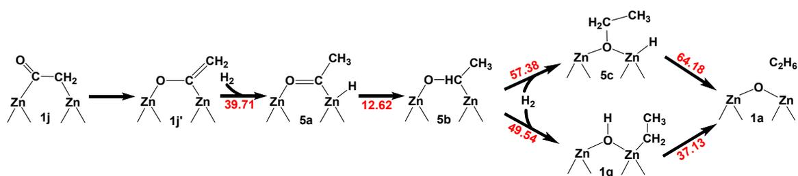
**Figure S5.** The other reaction pathways and barriers of 1j hydrogenation via 1j' (the isomer of 1j).
