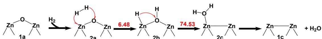
**Figure S1.** The reaction pathway and barriers of hydrogen reduction of  $[\text{Zn-O-Zn}]^{2+}$ .
