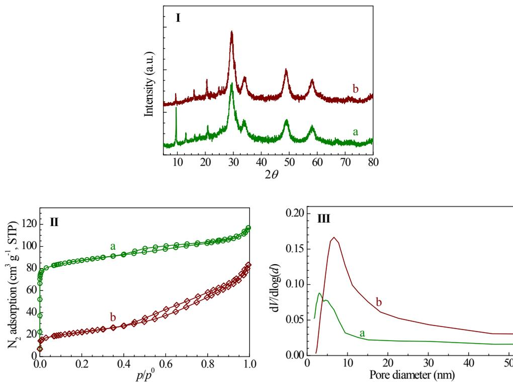
**Fig. S6.** XRD patterns (I),  $N_2$  adsorption-desorption isotherms (II) and corresponding pore size distribution curves (III) of the  $\text{Zn}_{0.5}\text{CeZrO}_x$ -glucose/SAPO-34 composite catalyst before (a, fresh) and after enduring the reaction of syngas to light olefins (b, spent).
