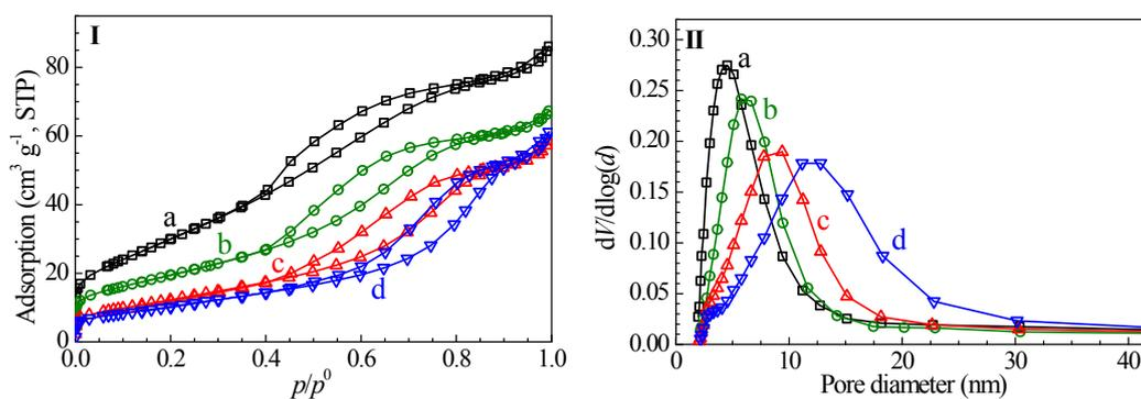
**Fig. S4.** N<sub>2</sub> adsorption-desorption isotherms (I) and corresponding pore size distribution curves (II) of the Zn<sub>0.5</sub>CeZrO<sub>x</sub>-glucose composite oxides (prepared with glucose as the complexing agent) calcined at different temperatures: (a) 400 °C; (b) 500 °C; (c) 600 °C; and (d) 700 °C.
