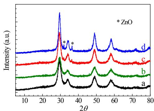
**Fig. S5.** XRD patterns of the Zn<sub>0.5</sub>CeZrO<sub>x</sub>-glucose composite oxides (prepared with glucose as the complexing agent) calcined at different temperatures: (a) 400 °C; (b) 500 °C; (c) 600 °C; and (d) 700 °C.
