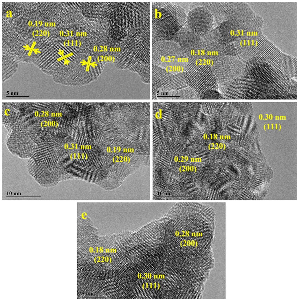
**Fig. S1.** HR-TEM images of the  $Zn_{0.5}CeZrO_x$  composite oxides prepared with different complexing agents: (a)  $Zn_{0.5}CeZrO_x$ -glucose, (b)  $Zn_{0.5}CeZrO_x$ -citric acid, (c)  $Zn_{0.5}CeZrO_x$ -tartaric acid, (d)  $Zn_{0.5}CeZrO_x$ -adipic acid, and (e)  $Zn_{0.5}CeZrO_x$ -L-alanine.
