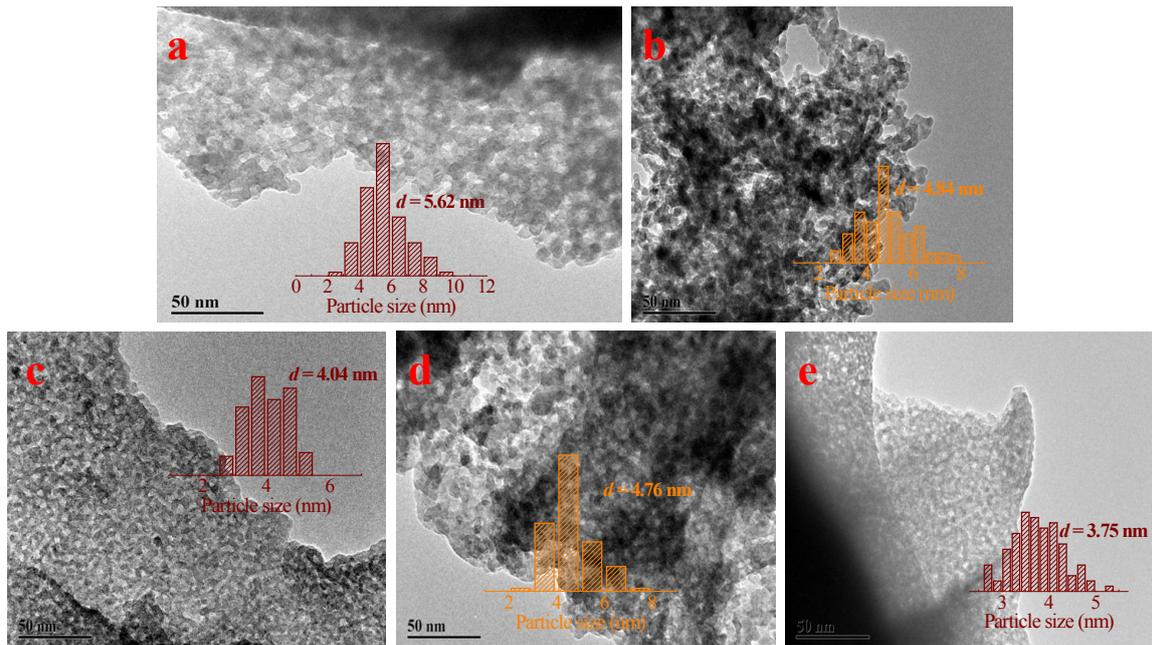
**Fig. S2.** TEM images and size distributions (estimated by counting more than 100 particles) of the  $\text{Zn}_{0.5}\text{CeZrO}_x$  composite oxides prepared with different complexing agents: (a)  $\text{Zn}_{0.5}\text{CeZrO}_x$ -glucose, (b)  $\text{Zn}_{0.5}\text{CeZrO}_x$ -citric acid, (c)  $\text{Zn}_{0.5}\text{CeZrO}_x$ -tartaric acid, (d)  $\text{Zn}_{0.5}\text{CeZrO}_x$ -adipic acid, and (e)  $\text{Zn}_{0.5}\text{CeZrO}_x$ -L-alanine.
