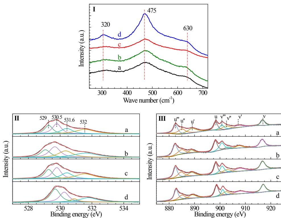
**Fig. S8.** Raman spectra **(I)**, O(1s) XPS spectra **(II)**, and Ce(3d) XPS spectra **(III)** of the Zn<sub>0.5</sub>CeZrO<sub>x</sub>-glucose composite oxides (prepared with glucose as the complexing agent) calcined at different temperatures: (a) 400 °C; (b) 500 °C; (c) 600 °C; and (d) 700 °C.
