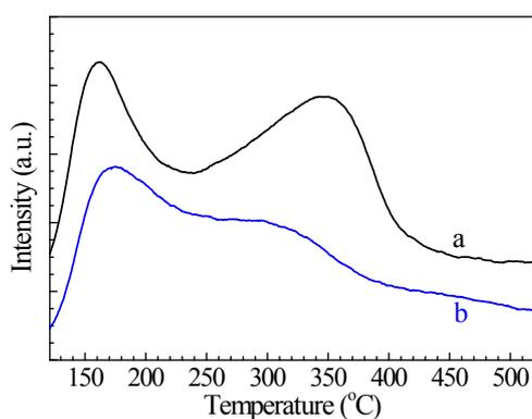
**Fig. S7.**  $\text{NH}_3$ -TPD profiles of the SAPO-34 molecular sieve (a) and the  $\text{Zn}_{0.5}\text{CeZrO}_x$ -glucose/SAPO-34 composite catalyst (b).
