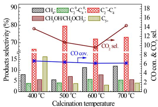
**Fig. S10.** CO conversion and products selectivity for the conversion of syngas over the  $\text{Zn}_{0.5}\text{CeZrO}_x$ -glucose/SAPO-34 bifunctional catalysts calcined at different temperatures (400, 500, 600 and 700 °C). Reaction conditions:  $\text{H}_2/\text{CO} = 2/1$ , 300 °C, 1.0 MPa, GHSV = 5400 mL/g·h, 30 h,  $\text{Zn}_{0.5}\text{CeZrO}_x/\text{SAPO-34} = 1$  (by mass); reported at a TOS of 30 h.
