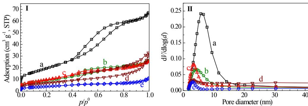
**Fig. S3.**  $\text{N}_2$  adsorption-desorption isotherms (I) and corresponding pore size distribution curves (II) of the  $\text{Zn}_{0.5}\text{CeZrO}_x$  composite oxides prepared with different complexing agents: (a)  $\text{Zn}_{0.5}\text{CeZrO}_x$ -glucose, (b)  $\text{Zn}_{0.5}\text{CeZrO}_x$ -citric acid, (c)  $\text{Zn}_{0.5}\text{CeZrO}_x$ -tartaric acid, (d)  $\text{Zn}_{0.5}\text{CeZrO}_x$ -adipic acid, and (e)  $\text{Zn}_{0.5}\text{CeZrO}_x$ -L-alanine.
