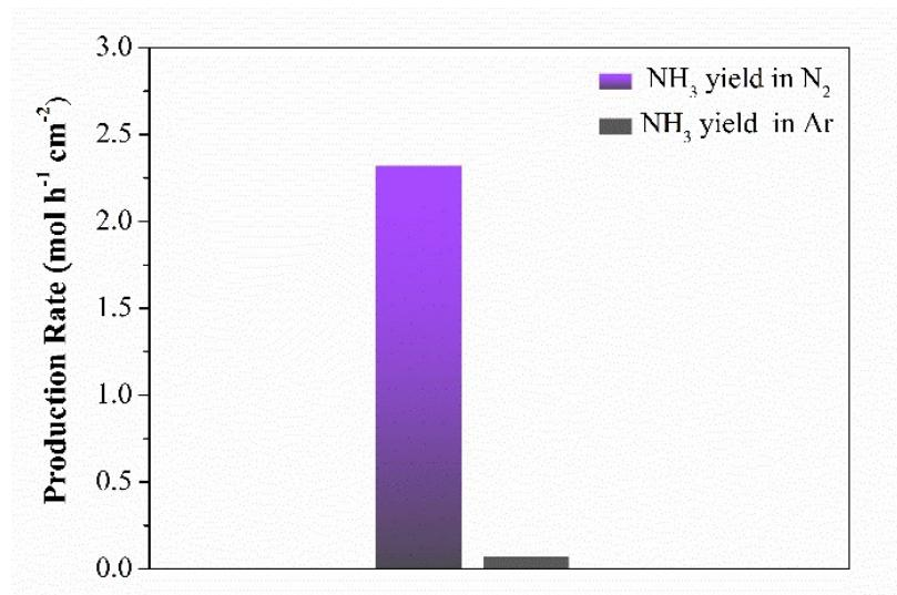
Fig. S7. Ammonia yield in N<sub>2</sub> and Ar environments at -0.4 V *vs.* RHE potential.
