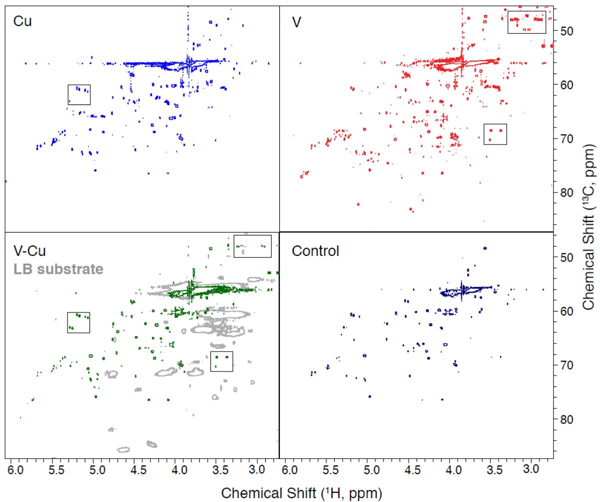
**Fig. S4** Comparison of  $^1\text{H}$ - $^{13}\text{C}$  HSQC NMR spectra of the LB substrate and the bio-oils obtained upon Cu, V and V-Cu catalysis in comparison to the bio-oil obtained in the control reaction. Reaction conditions: 150 °C, 10 min, 5 bar initial O<sub>2</sub>, 60 mL of 25 g/L lignin in 2 M NaOH. Amounts and ratios of the respective catalysts are given in Table S1 (ESI). The figure is an enlarged version of Fig. 7.
