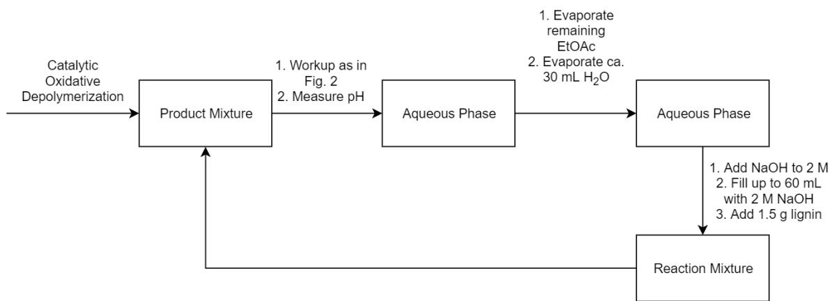
**Fig. S12** Workup procedure for the catalyst recycling experiment.
