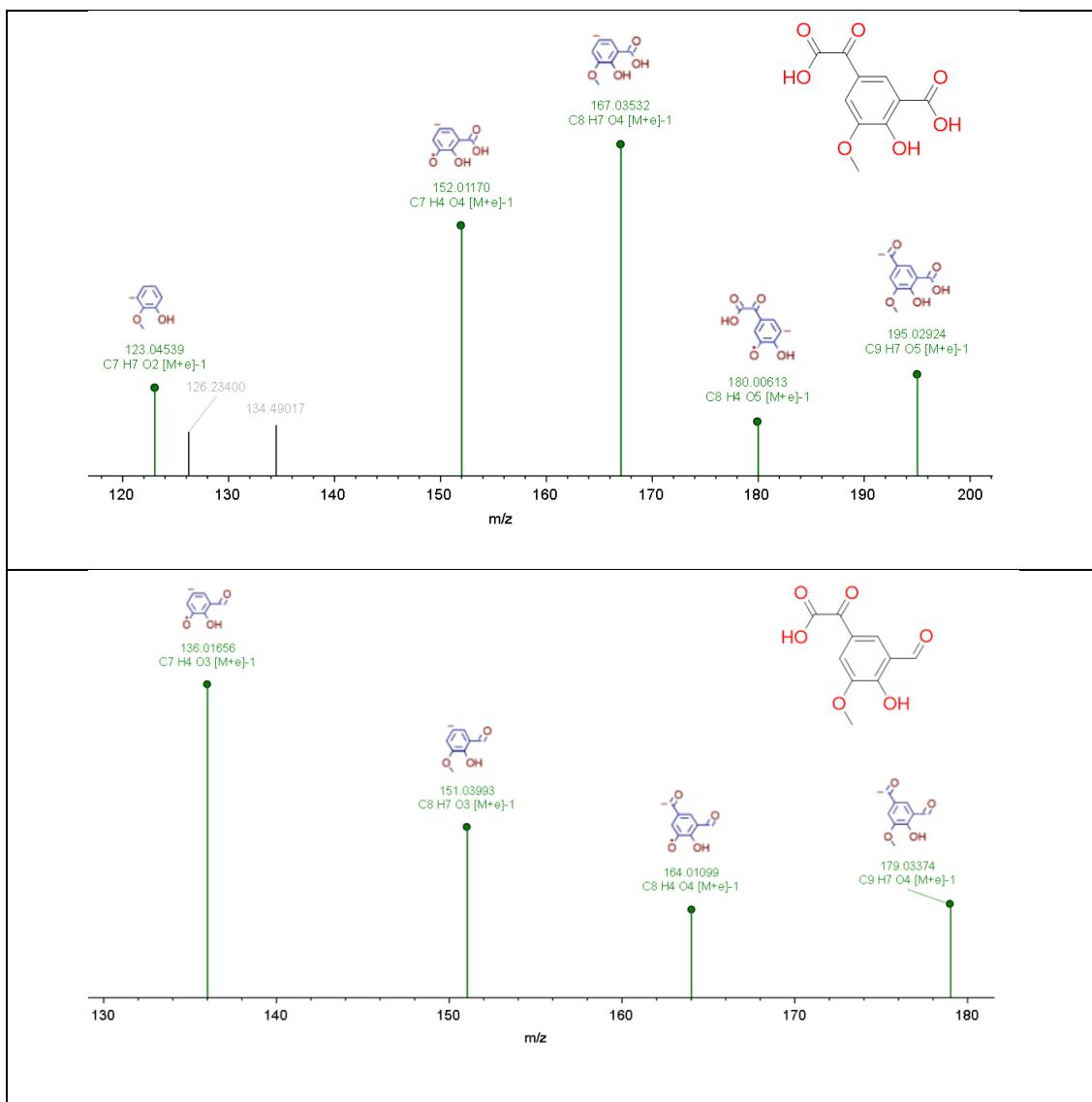
**Fig. S10** Fragmentation patters of collision-induced dissociation by HRMS of tentative structures, explained using the FiSH algorithm.
