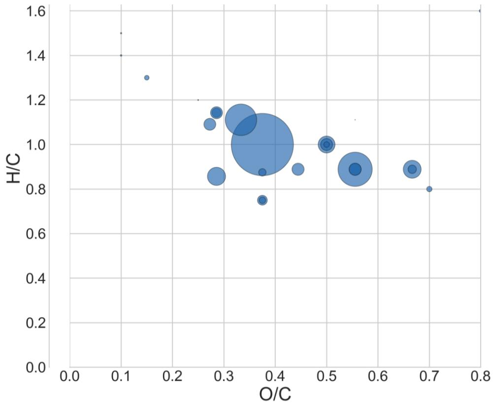
**Fig. S8** Van Krevelen analysis of the statistically indistinguishable species obtained from volcano plot of V-Cu catalyzed vs. control organic sample.
