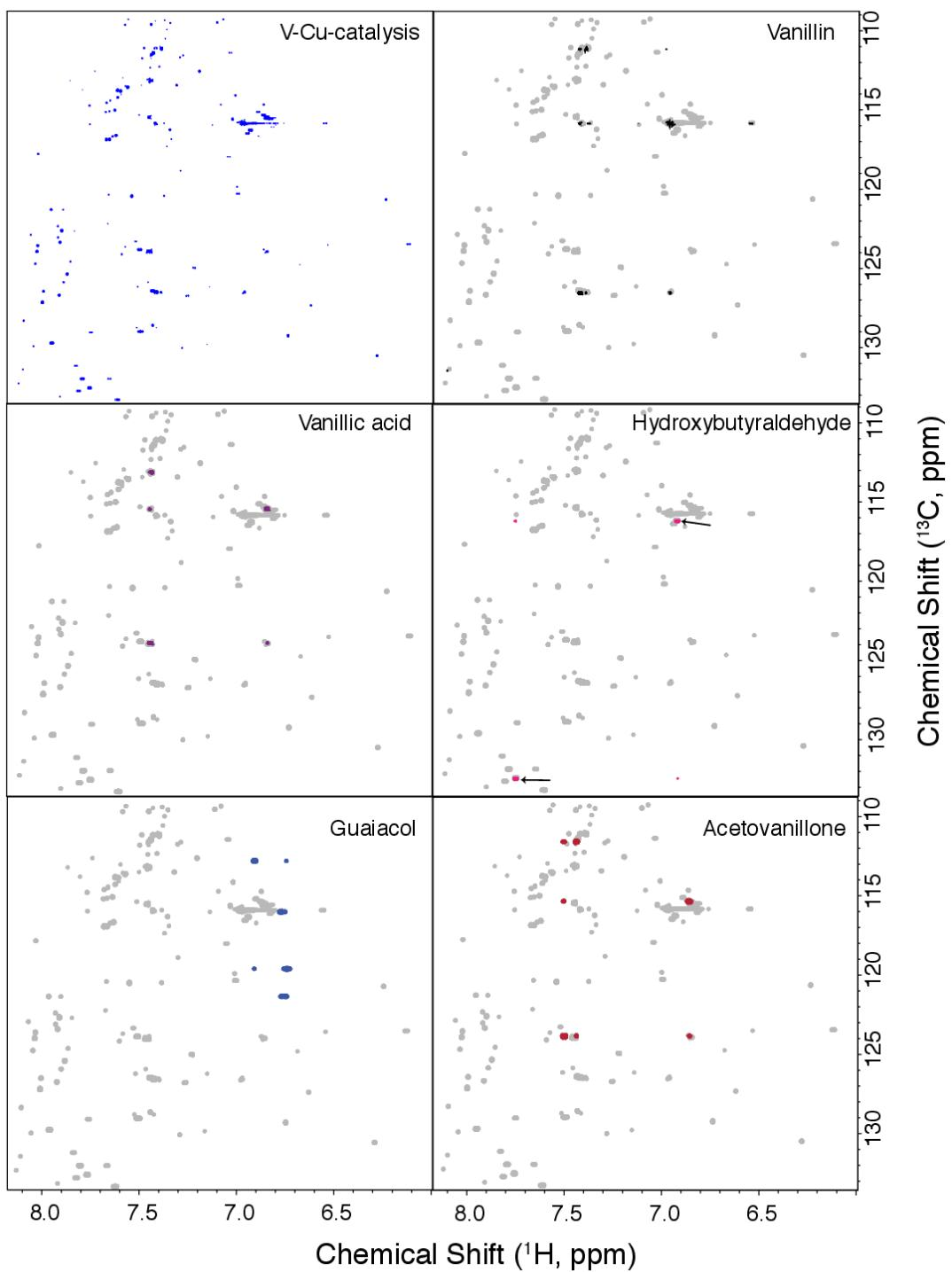
**Fig. S2**  $^1\text{H}$ - $^{13}\text{C}$  HSQC NMR spectra of the bio-oil obtained upon V-Cu catalysis and the spectra of selected compounds which were used for identification and quantification. Reaction conditions: 150 °C, 10 min, 5 bar initial O<sub>2</sub>, 60 mL of 25 g/L lignin in 2 M NaOH, 1.4 mmol VO(acac)<sub>2</sub>-Cu(OAc)<sub>2</sub> (V:Cu ratio = 0.75).
