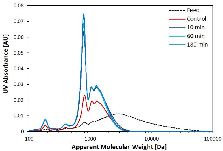
**Fig. S11** Molecular weight distributions of the feed, the control and the V-Cu-catalyzed samples (10, 60 and 180 min). Reaction conditions: 150 °C, 10 min, 5 bar initial O<sub>2</sub>, 60 mL of 25 g/L lignin in 2 M NaOH, 1.4 mmol VO(acac)<sub>2</sub>-Cu(OAc)<sub>2</sub> (V:Cu = 0.75).
