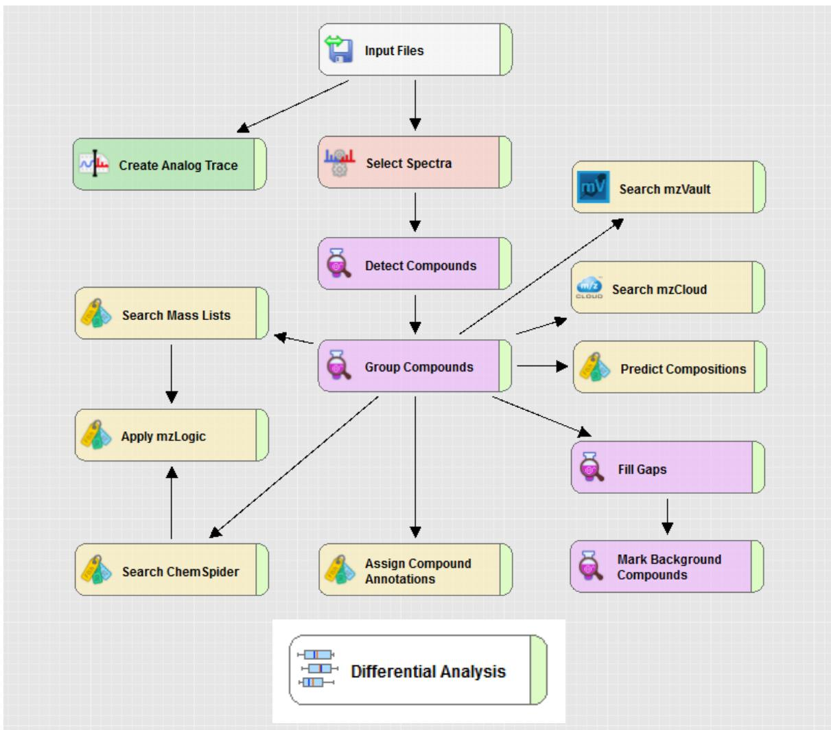
**Fig. S1** Compound Discoverer untargeted workflow used for deconvolution and processing of the obtained high-resolution mass spectrometry data.
