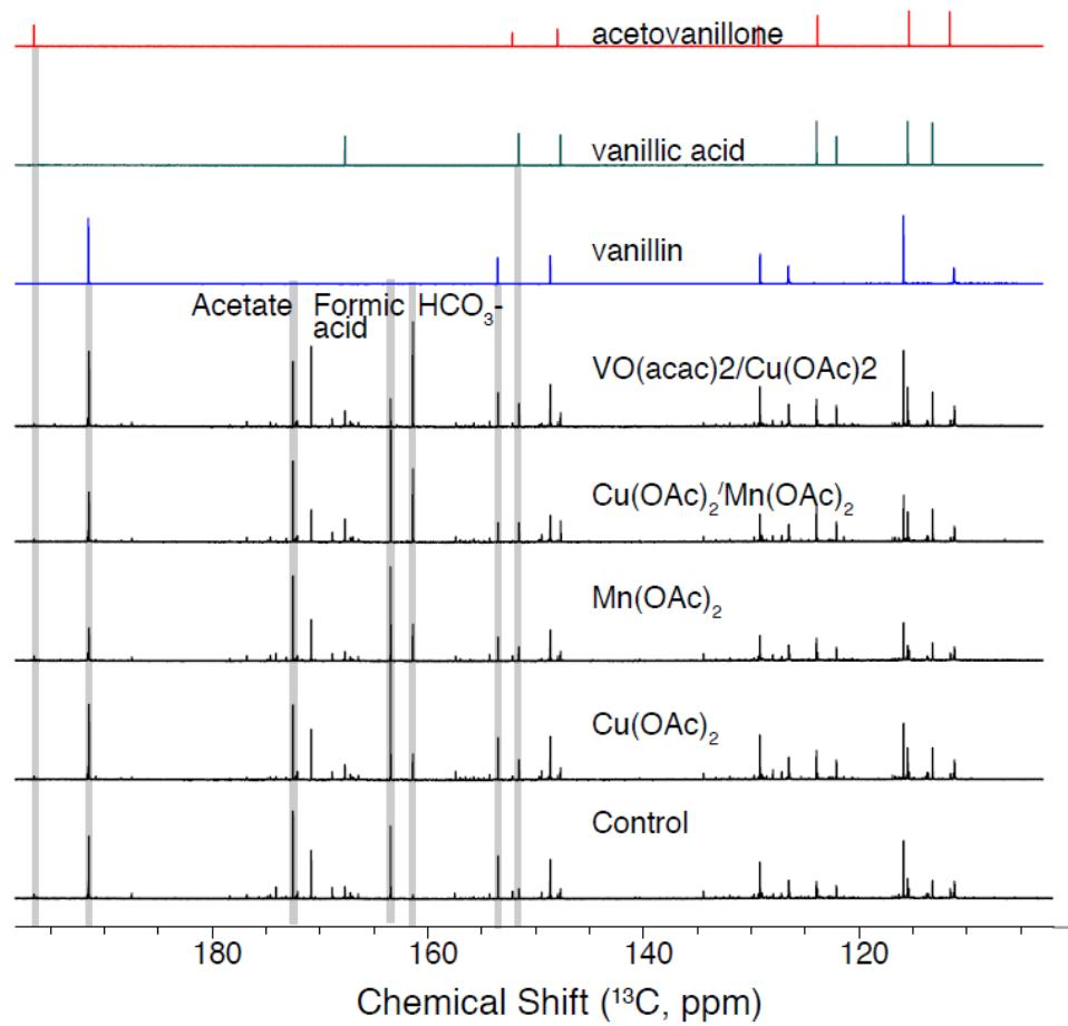
**Fig. S3**  $^{13}\text{C}$  NMR spectra of the prepared standards for vanillin, vanillic acid, acetovanillone compared to the bio-oil obtained by various catalyzed and control experiments.
