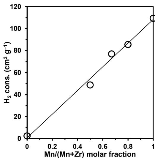
**Fig. S2** H<sub>2</sub> consumption during TPR *versus* the molar fraction of Mn in the  $\text{Mn}_1\text{Zr}_x\text{O}_y$  catalysts.
