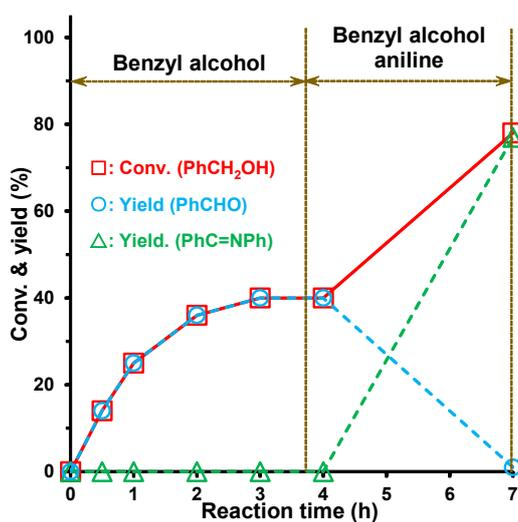
**Fig. S4** Time course for aerobic oxidation of benzyl alcohol with or without aniline. Reaction conditions: benzyl alcohol, 1 mmol; aniline, 1.5 mmol;  $\text{Mn}_1\text{Zr}_{0.5}\text{O}_y$ , 60 mg; toluene, 5 mL; air, 1 atm; temperature, 80 °C.
