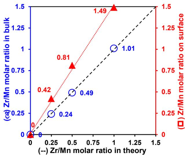
**Fig. S1** Zr/Mn molar ratio of the  $\text{Mn}_1\text{Zr}_x\text{O}_y$  catalysts obtained from bulk by ICP-MS and from surface by XPS as a function of the theoretical ratio.
