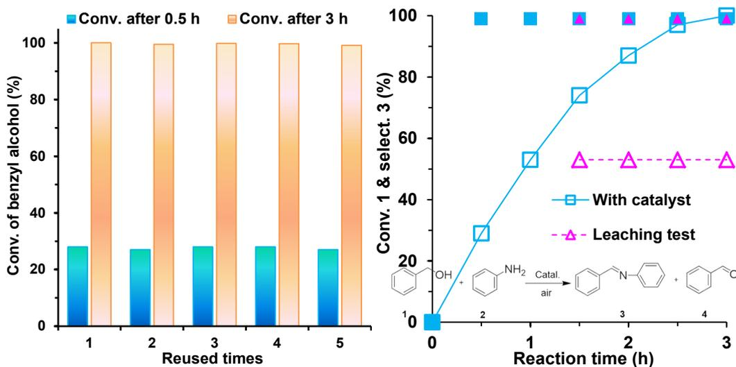
**Fig. S3** (left) Recycling test of the  $\text{Mn}_1\text{Zr}_{0.5}\text{O}_y$  catalyst for oxidative coupling of benzyl alcohol with aniline within the kinetic-controlled region and under the optimized conditions. (right) Leaching test of metals in the  $\text{Mn}_1\text{Zr}_{0.5}\text{O}_y$  catalyst during oxidative coupling of benzyl alcohol with aniline. Reaction conditions: benzyl alcohol, 1 mmol; aniline, 1.5 mmol; catalyst, 60 mg; toluene, 5 mL; air, 1 atm; temperature, 80 °C.
