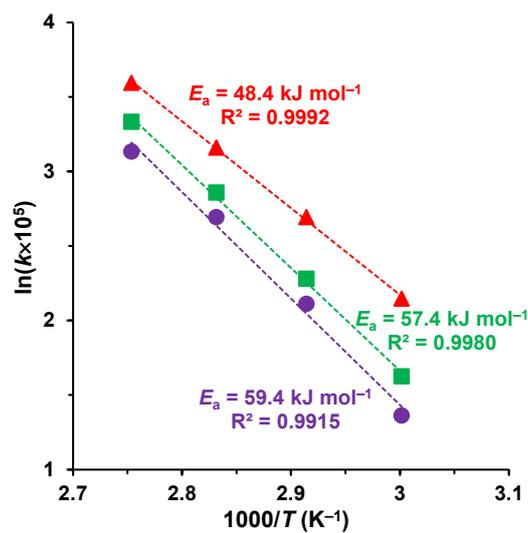
**Fig. S5** Arrhenius plot for conversion of benzyl alcohol during oxidative coupling of benzyl alcohol with aniline over the (●)  $\text{Mn}_1\text{Zr}_{0.25}\text{O}_y$ , (■)  $\text{Mn}_1\text{Zr}_{0.5}\text{O}_y$  and (⊗)  $\text{Mn}_1\text{Zr}_1\text{O}_y$  catalysts. Reaction conditions: benzyl alcohol, 1 mmol; aniline, 1.5 mmol; catalyst, 60 mg; toluene, 5 mL; air, 1 atm; temperature, 60–90 °C; time, 1.5 h.
