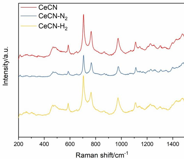
Fig. S8 The Raman spectra of the CeO<sub>2</sub>/g-C<sub>3</sub>N<sub>4</sub> samples.
