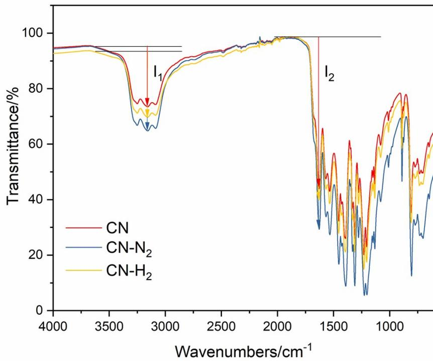
Fig. S5 FT-IR spectra of g-C<sub>3</sub>N<sub>4</sub> under different atmosphere treatment.
