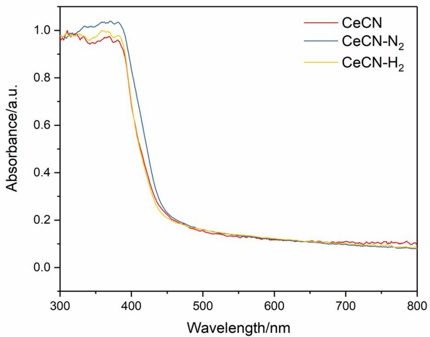
Fig. S6 UV-vis absorption spectra of CeO<sub>2</sub>/g-C<sub>3</sub>N<sub>4</sub> samples.
