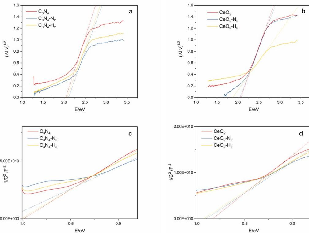
Fig. S3 Plot of  $(Ah\nu)^{1/2}$  versus photon energy of (a). g- $C_3N_4$  and (b).  $CeO_2$  samples and the Mott-Schottky plots of (c). g- $C_3N_4$  and (d).  $CeO_2$  samples.
