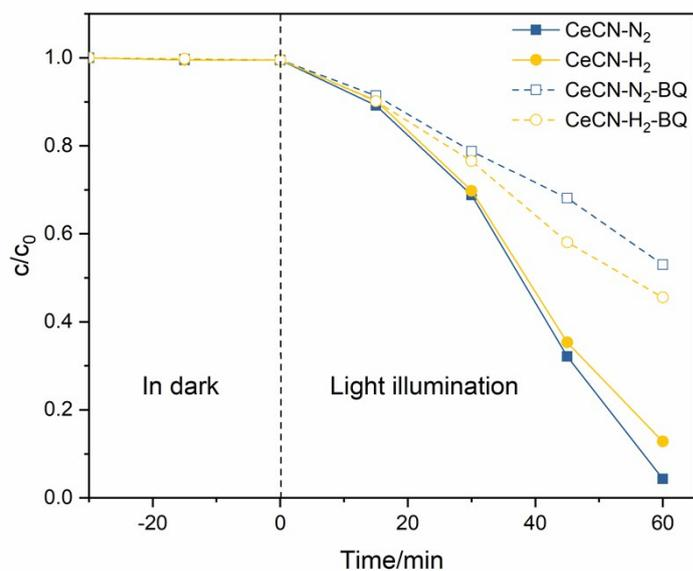
Fig. S4 The activities of MB degradation of  $CeO_2/g-C_3N_4$  samples.
