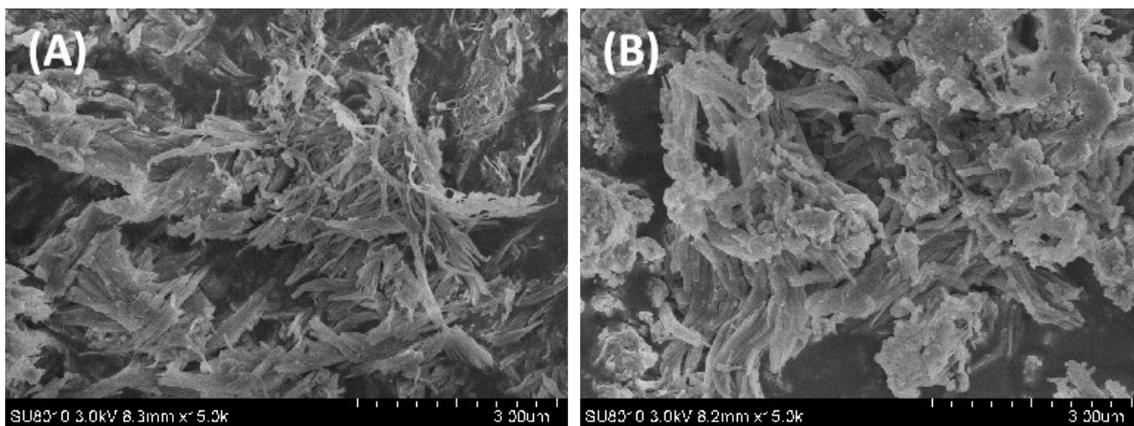
**Figure S1** (A) SEM image of PhC<sub>2</sub>Cu; (B) SEM image of 2% Fe/PhC<sub>2</sub>Cu.
