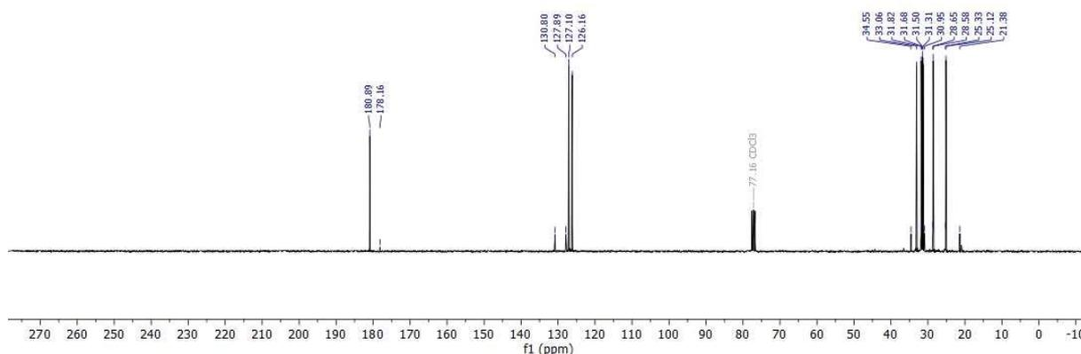
$^{13}\text{C}$  NMR (75 MHz,  $\text{CDCl}_3$ ) spectrum of 2c.
