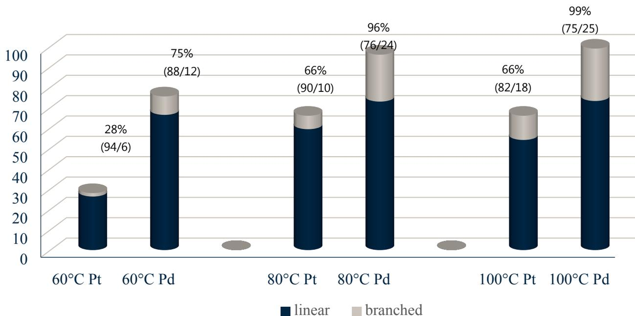
Conditions: 1.0 mmol 1a, 1.0 mol% [M], 2.2 mol% L9, 0.5 mL H<sub>2</sub>SO<sub>4</sub> [0.6 M], in 1.5 mL acetic acid, X °C, 18 h. Results are obtained by GC analysis.
