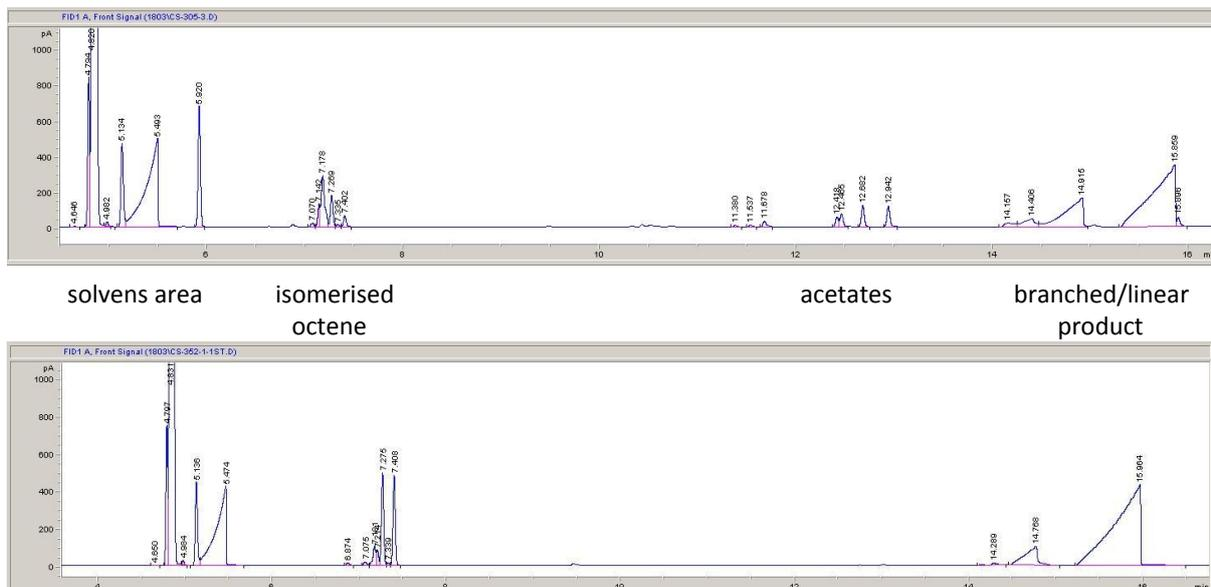
TOP: Reaction conditions: 1.0 mmol 1a, 1.0 mol% PtCl<sub>2</sub>, 2.2 mol% L9, 0.5 mL 0.3M H<sub>2</sub>SO<sub>4</sub>, 1.5 ml acetic acid, 40 bar CO, 120 °C, 18 h.
