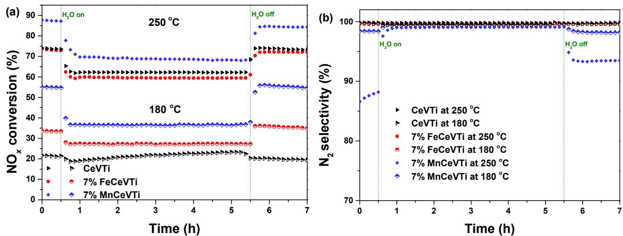
**Fig. S2** The effect of H<sub>2</sub>O on (a) NO<sub>x</sub> conversion and (b) N<sub>2</sub> selectivity of CeVTi, 7%FeCeVTi and 7%MnCeVTi with time at 180 °C and 250 °C with GHSV of 150, 000 h<sup>-1</sup> in the reaction gas containing 500 ppm NO, 500 ppmNH<sub>3</sub>, 5 vol% O<sub>2</sub>, 3 vol % H<sub>2</sub>O and N<sub>2</sub> balance.
