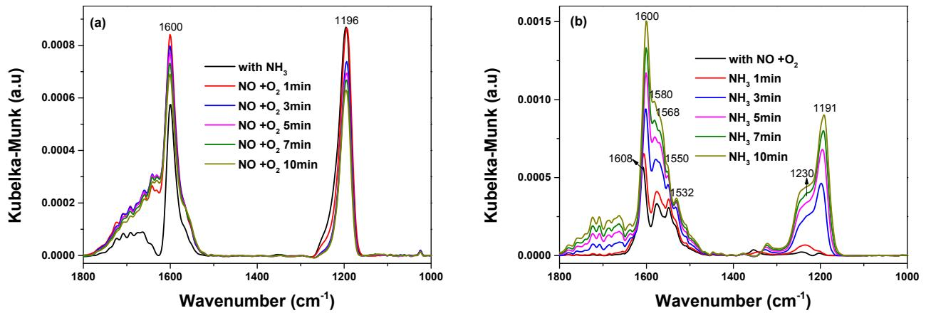
**Fig. S6** In situ DRIFTS of CeVTi catalyst exposed to (a) 500 ppm NO+5% O<sub>2</sub>/N<sub>2</sub> after 500 ppm NH<sub>3</sub>/N<sub>2</sub> for 30 min followed with 20 min N<sub>2</sub> purge, and (b) 500 ppm NH<sub>3</sub>/N<sub>2</sub> after 500 ppm NO+5% O<sub>2</sub>/N<sub>2</sub> for 30 min followed with 20 min N<sub>2</sub> purge in order at 250 °C.
