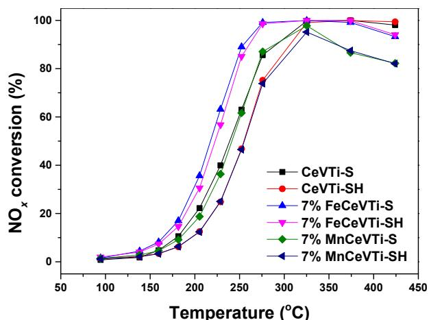
**Fig. S3** NO<sub>x</sub> conversion of used CeVTi, 7%FeCeVTi and 7%MnCeVTi after SO<sub>2</sub> resistance (suffix-S) and SO<sub>2</sub>-H<sub>2</sub>O resistance test (suffix -SH) measured at different temperatures with a gaseous mixture containing 500 ppm NO, 500 ppmNH<sub>3</sub>, 5% O<sub>2</sub> and N<sub>2</sub> balance.
