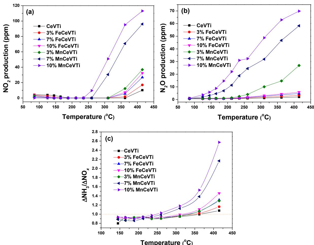
Fig. S1 (a)  $\text{NO}_2$  production, (b)  $\text{N}_2\text{O}$  production, (c)  $\Delta\text{NH}_3/\Delta\text{NO}_x$  of the prepared catalysts
