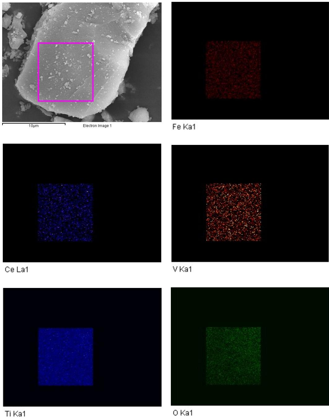
**Fig. S5** EDS-mapping images of elements in 7%FeCeVTi catalyst
