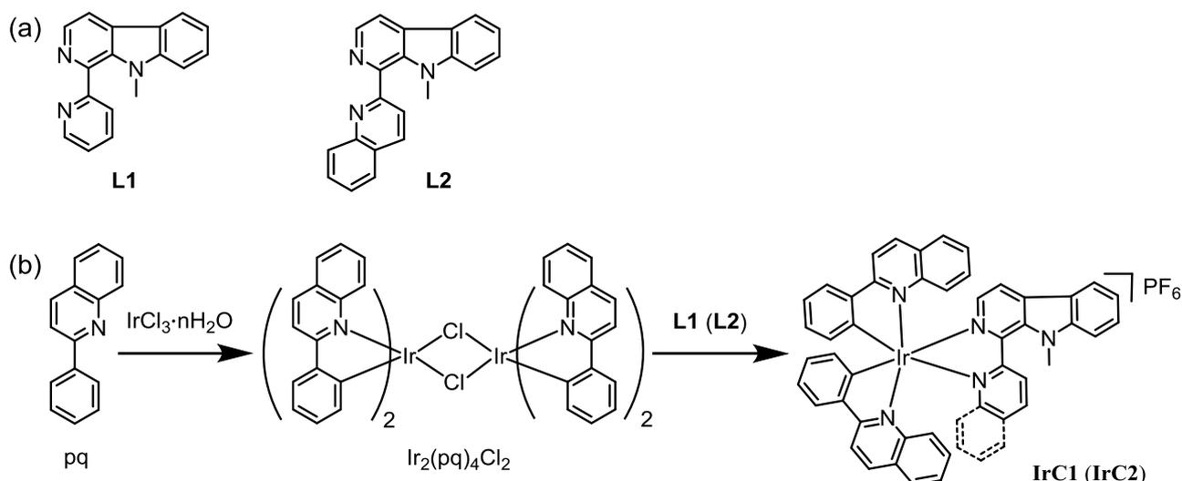
**Scheme S1.** (a) Chemical structures of **L1** and **L2**. (b) Synthetic procedures of iridium(III) complexes **IrC1** and **IrC2**.
