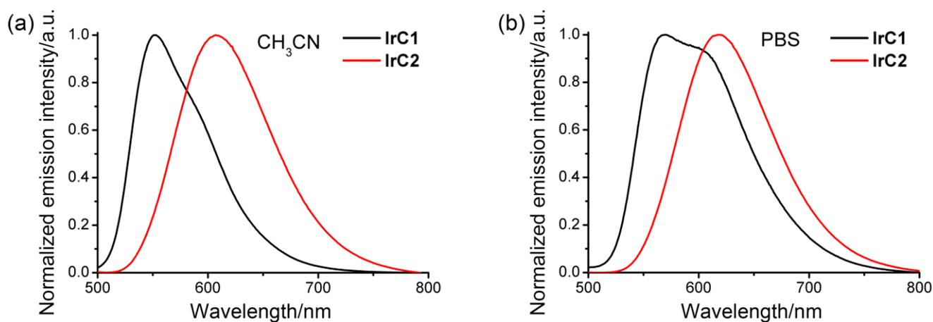
**Fig. S8** Emission spectra of complexes IrC1 and IrC2 (10 μM) measured in (a) CH<sub>3</sub>CN and (b) PBS at 25 °C.  $\lambda_{\text{ex}} = 405$  nm.
