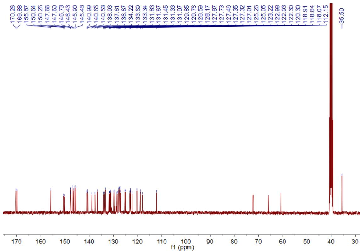
Fig. S5  $^{13}\text{C}$  NMR spectrum of IrC1 in  $d_6$ -DMSO.
