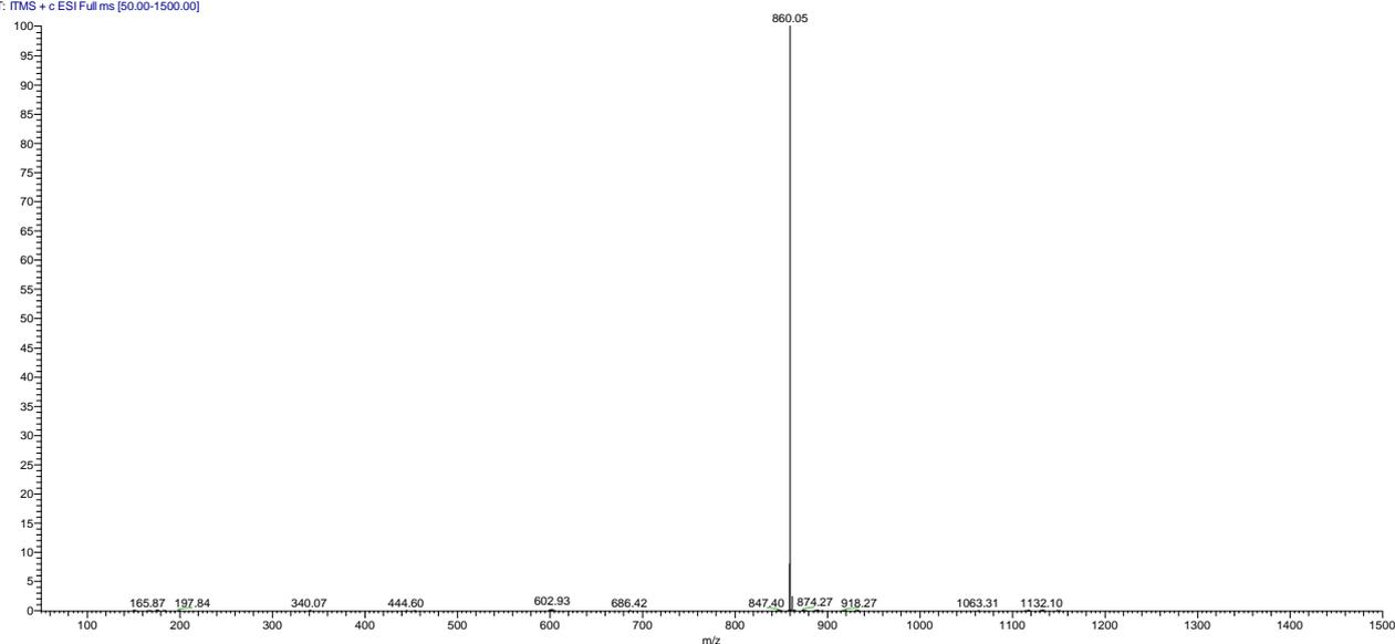
**Fig. S1** ESI-MS characterization of **IrC1**, 860.05  $[M-PF_6]^+$ .
