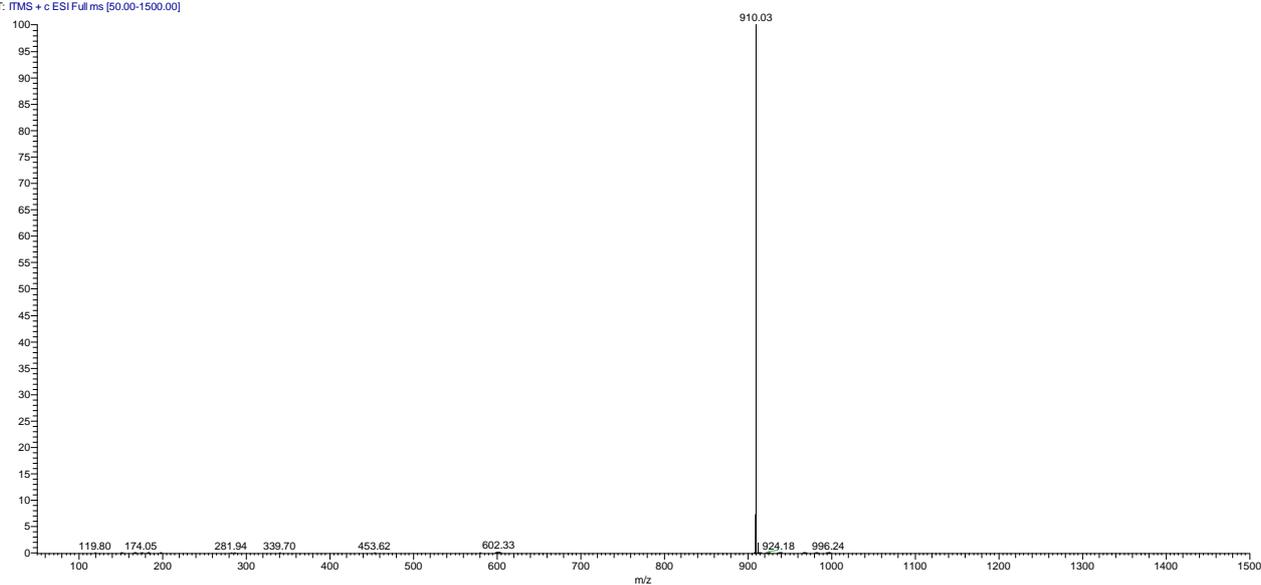
**Fig. S2** ESI-MS characterization of **IrC2**, 910.03  $[M-PF_6]^+$ .
