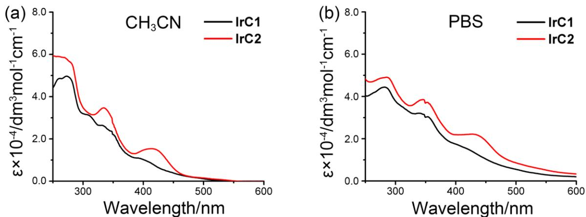
**Fig. S7** UV/Vis spectra of IrC1 and IrC2 (10 μM) measured in (a) CH<sub>3</sub>CN and (b) PBS at 25 °C.
