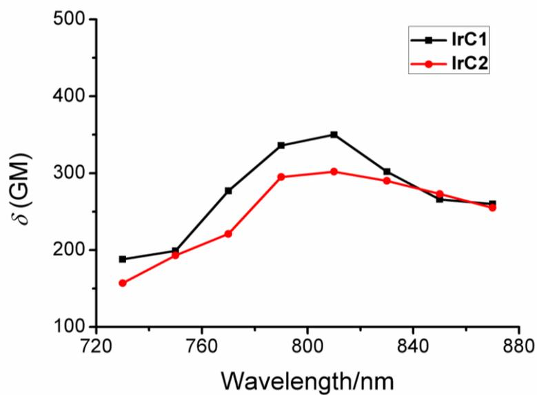
**Fig. S9** TPA cross-sections ( $\delta$ ) of IrC1 and IrC2 at excitation wavelengths between 730 and 870 nm.
