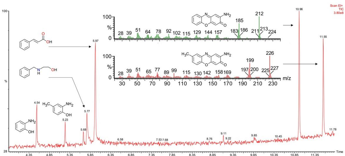
**Figure S18.** Fragment of the chromatogram showing the reaction products, non-reacted substrates and ligands in the oxidation of 2-amino-*p*-cresol (APC) and *o*-aminophenol (OAP), 5 mM each, catalysed by **1** (1 mM). The inset shows the EI mass-spectra of the products.
