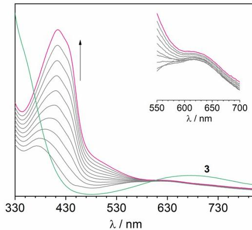
**Figure S16.** Increase in the phenoxazine band (435 nm) over time (the spectra were recorded with 2 min intervals) in the oxidation of OAP (2.4 mM) catalysed by **3** ( $[Cu]_0 = 0.5$  mM) in  $CH_3OH$  at room temperature. Green line shows the absorption spectra of pure **3** (1 mM) in  $CH_3OH$  taken. Inset shows evolution of 620 nm absorption with time.
