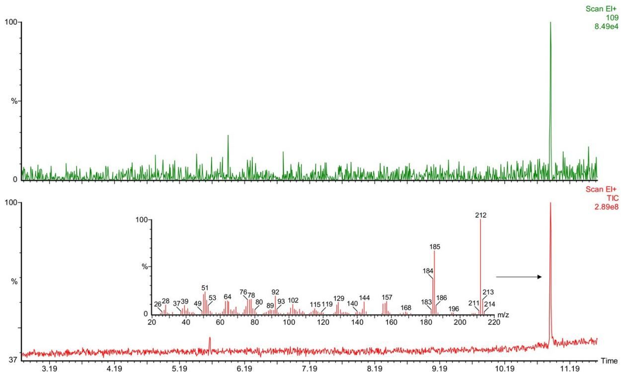
**Figure S12.** Fragments of the chromatogram (bottom) showing the peak of a phenoxazinone chromophore (at 10.9 min) after 24 h oxidation of OAP catalysed by 2 mM of **2**. The inset shows the respective EI mass spectrum. The top chromatogram shows the intensity of 109 m/z signal, corresponding to a substrate (OAP), indicating the complete conversion of OAP.
