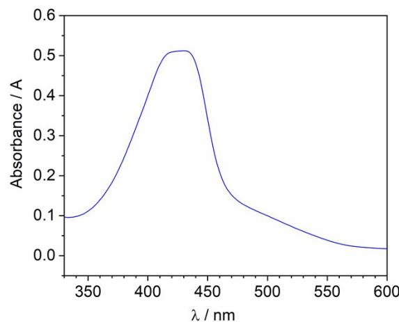
**Figure S13.** UV-Vis spectrum of the solution obtained after 24 h stirring of 0.01 mM of OAP and 1.1 mM of **3** in methanol, under inert atmosphere. Due to strong absorbance of phenoxazinone chromophore direct measurement of solution spectrum was not possible. Instead, 0.5 mL of reaction mixture was diluted with 4 mL of methanol, the resulting solution was immediately transferred to UV cuvette. Further measurements performed after 5 and 10 min did not show notable changes of absorbance.
