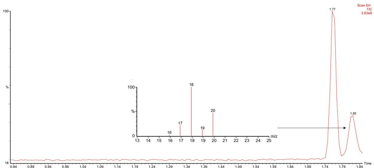
**Figure S17.** Fragment of the chromatogram, showing the peaks of dioxygen (1.77 min) and water (1.83) in the oxidation of OAP (10 mM) with  $^{18}O_2$ , catalysed by **3** (1.2 mM), in methanol, after 3 h. The inset shows the EI mass-spectrum that discloses the presence of  $H_2^{18}O$ .
