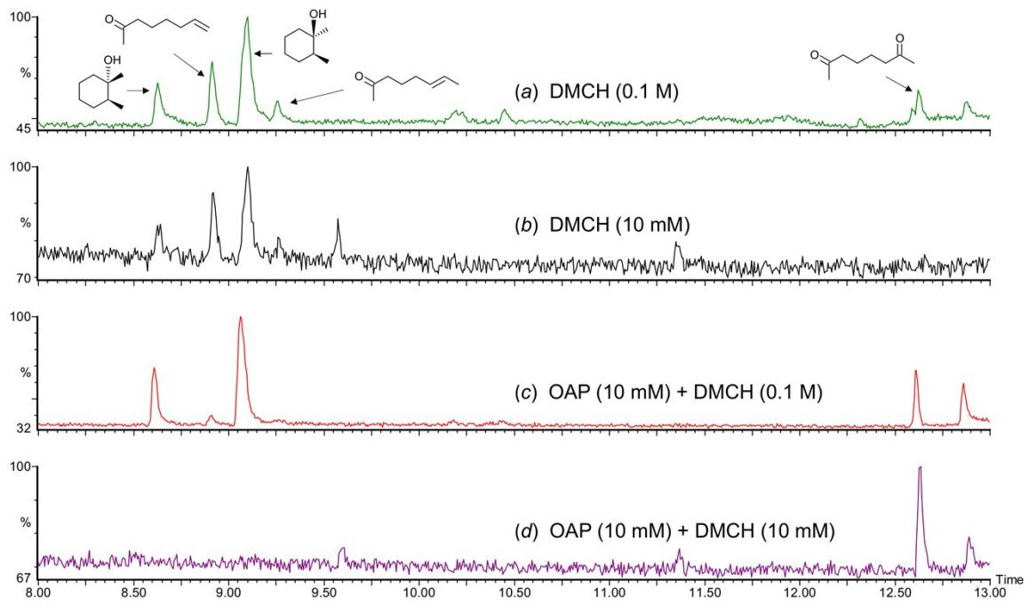
**Figure S20.** Fragments of the chromatograms showing the products of the aerobic oxidation of *cis*-1,2-dimethylcyclohexane, catalysed by **3** (1.5 mM), in the presence or absence of OAP.
