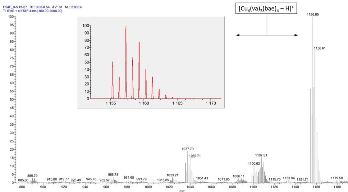
**Figure S8.** Fragment of the ESI-MS spectrum of **2** showing the experimental and theoretical (inset) MS isotopic patterns for [Cu<sub>4</sub>(va)<sub>3</sub>(bae)<sub>4</sub> - H]<sup>+</sup>.
