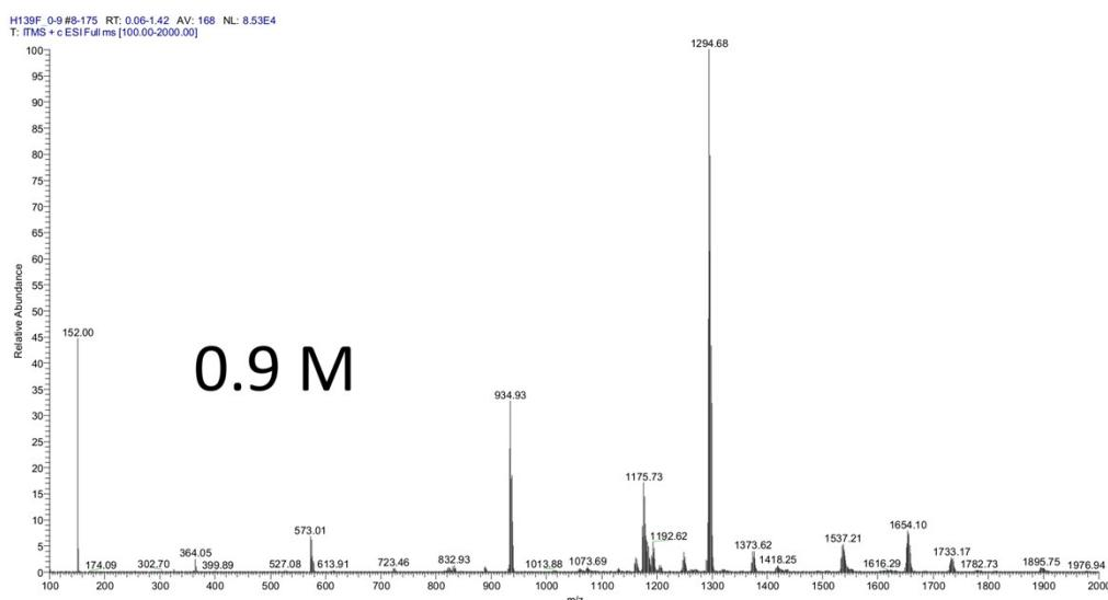
**Figure S9.** ESI-MS spectra of **1** in methanol depending on the full concentration of copper.
