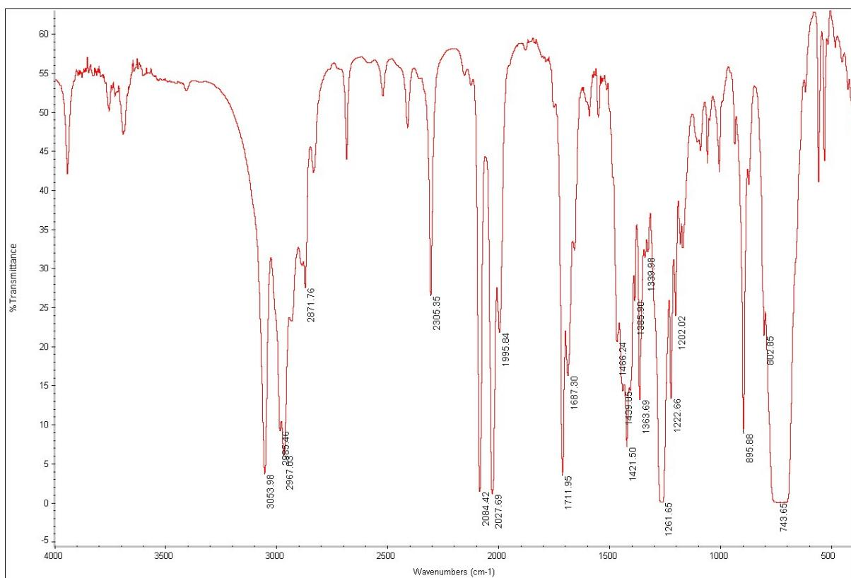
**Figure S20.** Solution ( $\text{CH}_2\text{Cl}_2$ ) IR spectrum of **3** treated with CO.
