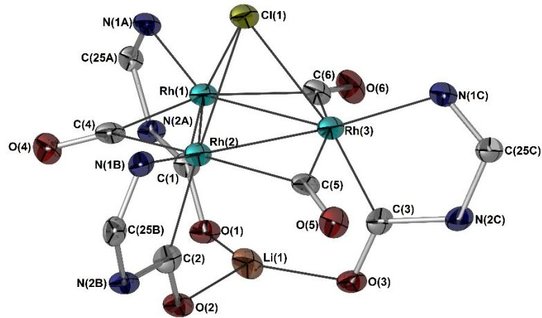
**Figure S1.** Molecular structure (50% displacement ellipsoids) of **2**. All Dipp groups and hydrogen atoms removed for clarity.
