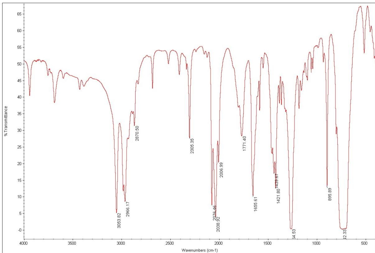
**Figure S22.** Solution ( $\text{CH}_2\text{Cl}_2$ ) IR spectrum of **4** treated with CO and aged for 24 h at room temperature.
