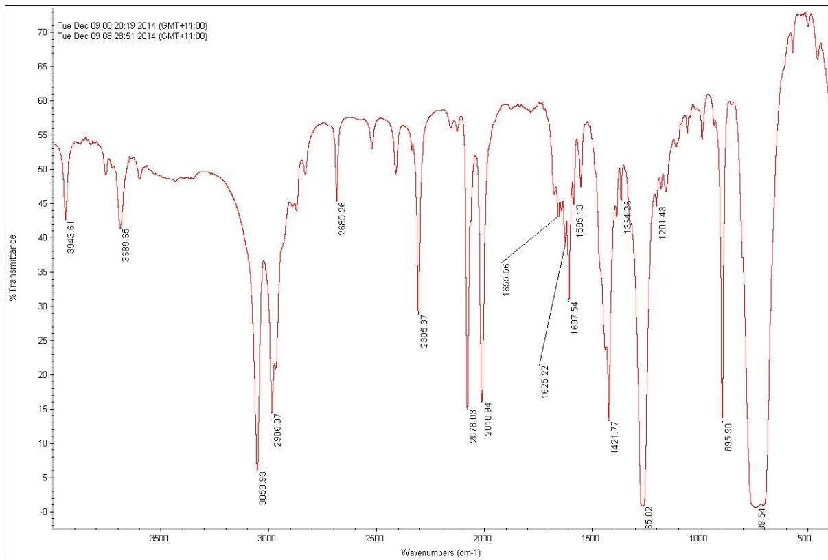
**Figure S21.** Solution ( $\text{CH}_2\text{Cl}_2$ ) IR spectrum of **4** treated with CO.
