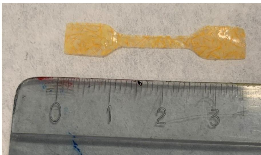
**Figure S24.** Macrograph of  $[\text{Cu}(\text{NH}_2\text{-MeIN})\text{I}]_n@\text{EVA}$  composite sample.
