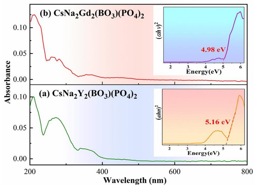
**Figure S5.** Experimental UV-Vis absorption spectrum of  $\text{CsNa}_2\text{REE}_2(\text{BO}_3)(\text{PO}_4)_2$  (REE = Y, Gd) ranging from 200 to 800 nm.
