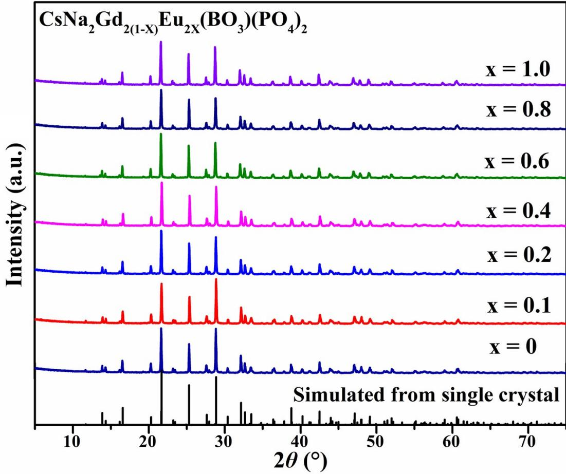
**Figure S2.** Simulated X-ray powder diffraction pattern of CsNa<sub>2</sub>Gd<sub>2</sub>(BO<sub>3</sub>)(PO<sub>4</sub>)<sub>2</sub> and experimental XRD patterns of CsNa<sub>2</sub>Gd<sub>2(1-x)</sub>Eu<sub>2x</sub>(BO<sub>3</sub>)(PO<sub>4</sub>)<sub>2</sub> ( $x = 0-1$ ) in the  $2\theta$  range of  $5-75^\circ$ .
