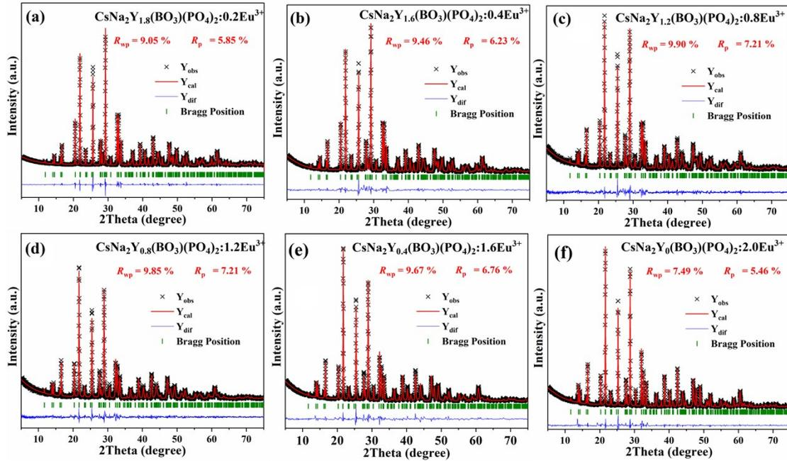
**Figure S3.** (a), (b), (c), (d), (e) and (f) Rietveld refinements of the XRD files for CsNa<sub>2</sub>Y<sub>2(1-x)</sub>Eu<sub>2x</sub>(BO<sub>3</sub>)(PO<sub>4</sub>)<sub>2</sub> ( $x = 0.1, 0.2, 0.4, 0.6, 0.8$  and  $1.0$ ), respectively.
