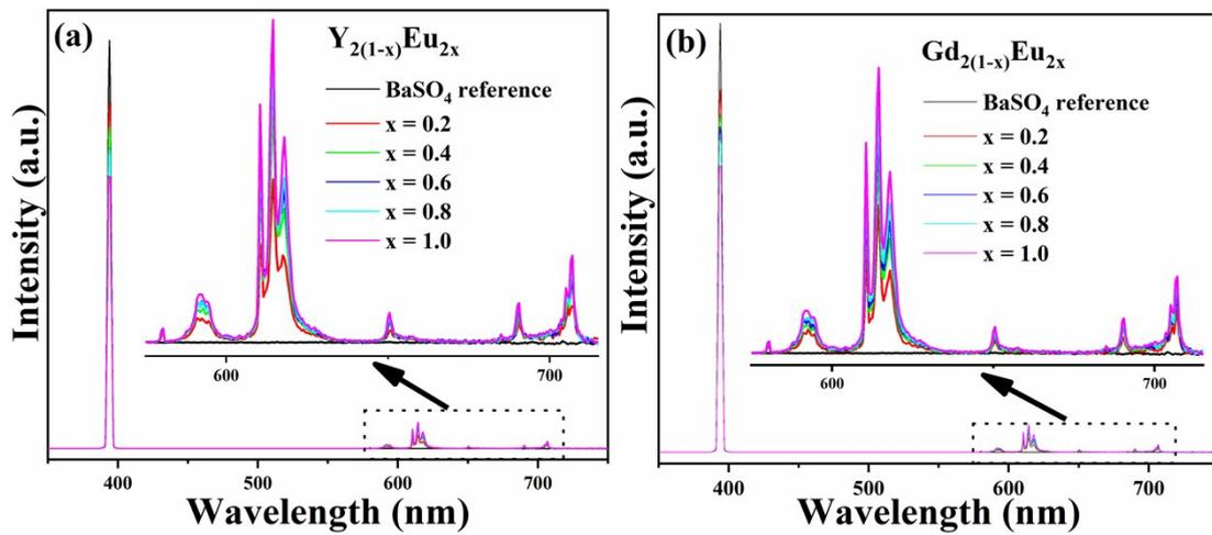
**Figure S7.** Excitation line of  $\text{BaSO}_4$  and emission spectra of phosphor  $\text{CsNa}_2\text{Y}_{2(1-x)}\text{Eu}_{2x}(\text{BO}_3)(\text{PO}_4)_2$  (a) and  $\text{CsNa}_2\text{Gd}_{2(1-x)}\text{Eu}_{2x}(\text{BO}_3)(\text{PO}_4)_2$  (b) collected by using an integrating sphere.
