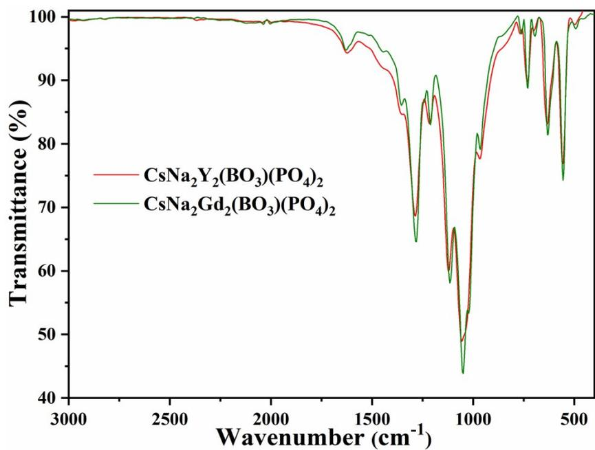
**Figure S4.** The IR spectra of  $\text{CsNa}_2\text{REE}_2(\text{BO}_3)(\text{PO}_4)_2$  (REE = Y, Gd).
