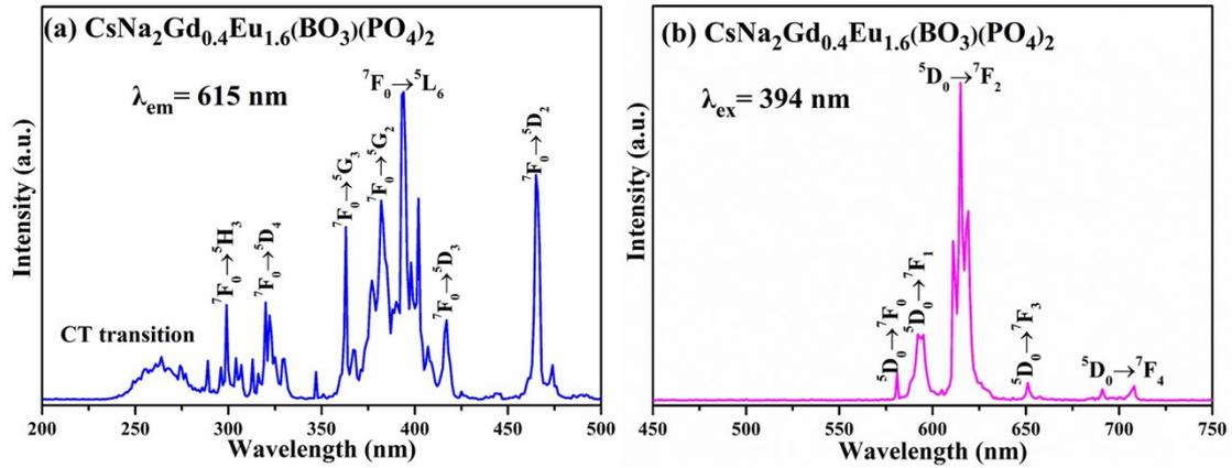
**Figure S6.** (a) Excitation spectrum of the  $\text{CsNa}_2\text{Gd}_{0.4}\text{Eu}_{1.6}(\text{BO}_3)(\text{PO}_4)_2$  by monitoring the emission wavelength at 615 nm; (b) Emission spectrum of the  $\text{CsNa}_2\text{Gd}_{0.4}\text{Eu}_{1.6}(\text{BO}_3)(\text{PO}_4)_2$  and excited by 394 nm.
