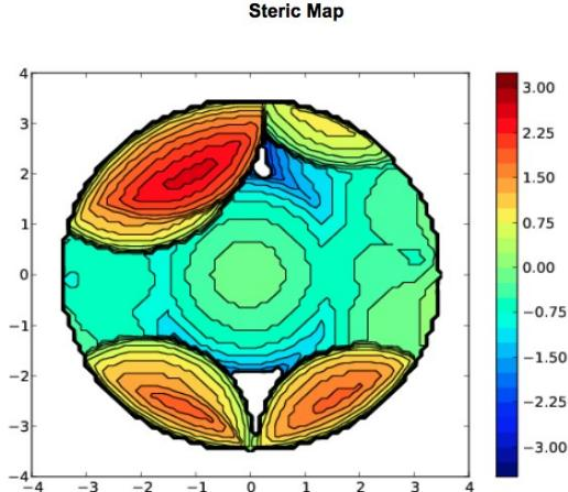
F. %V<sub>Bur</sub> for **4a** with distance C-Ag normalized at 2.1 Å, sphere radius 3.5 Å.
