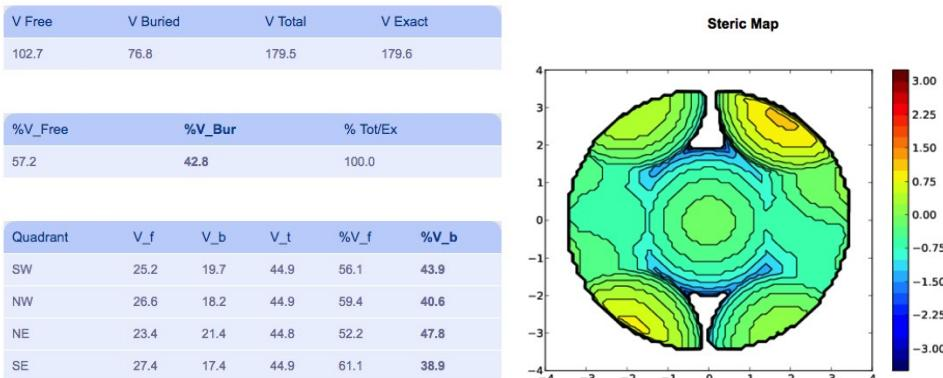
D. %V<sub>Bur</sub> for **2b** with distance C-Ag normalized at 2.1 Å, sphere radius 3.5 Å.
