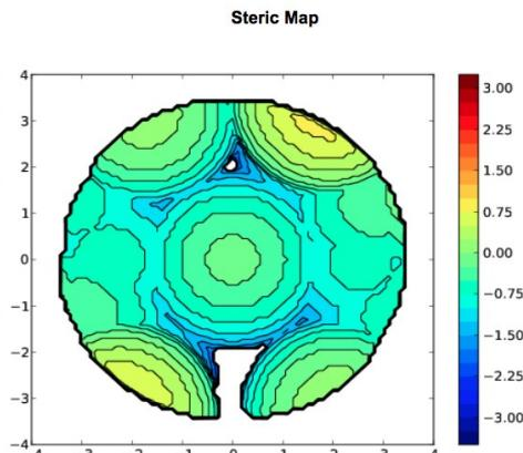
J. %V<sub>Bur</sub> for **4b** with distance C-Ag normalized at 2.1 Å, sphere radius 3.5 Å.
